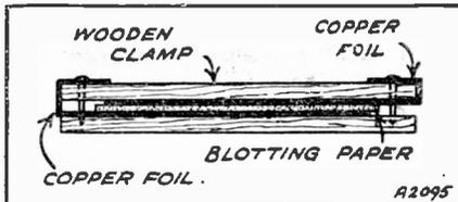
The blotting paper is sandwiched between the copper foil like the dielectric of a condenser.
