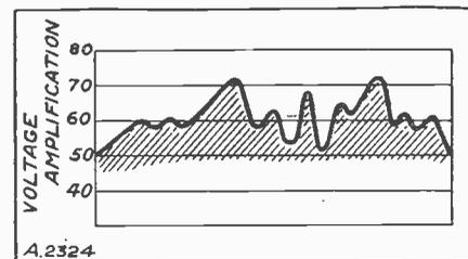
Although the voltage-amplification variations shown look very nasty, it is unlikely that even a keen ear would hear the difference between these and a completely straight-line response.
