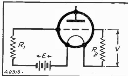
In this diagram the resistances are shown as they appear in a circuit in practice.  $R_2$  represents the valve's impedance between grid and filament, and  $R_1$  the value of the grid leak through which the bias is applied.
