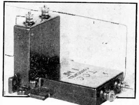
Nowadays, some fixed condensers have very useful "double feet." They enable these components to be mounted in two positions.
