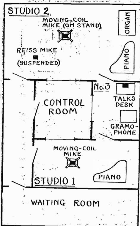
The engineers in the control room can see into any of the studios through plate-glass windows.
