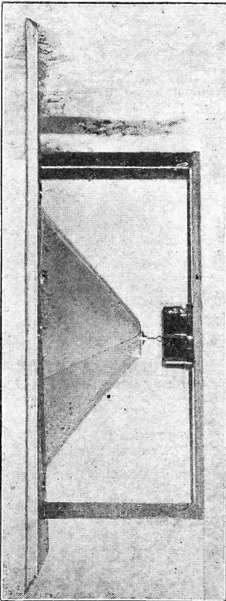
This is what the speaker looks like from the side. Note that the front edge of the cone comes flush with the back of the baffle.
