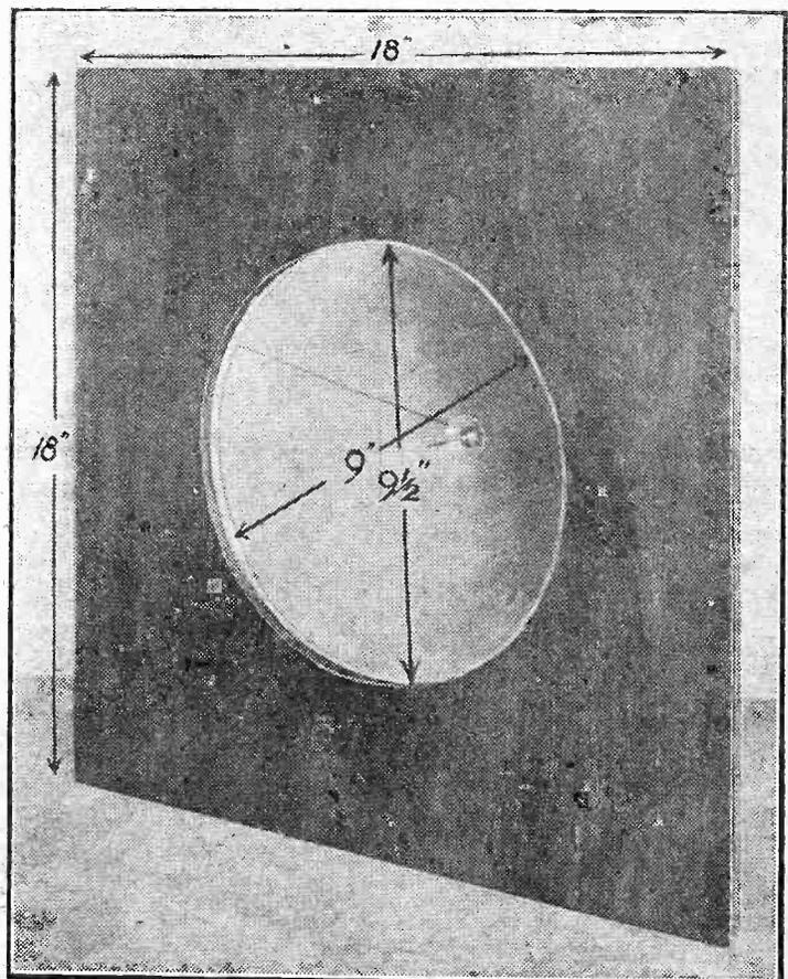
You won't find anything difficult in cutting the baffle to size. Note that the hole in it is 1/2 inch larger than the cone's diameter. This is to ensure that the edge of the cone will not touch the baffle anywhere.
