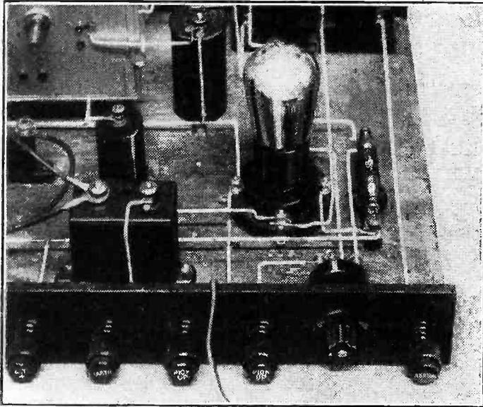
On the right is the aerial terminal, and next to it the radio-gram switch and the two terminals for the leads to a pick-up, if used.
