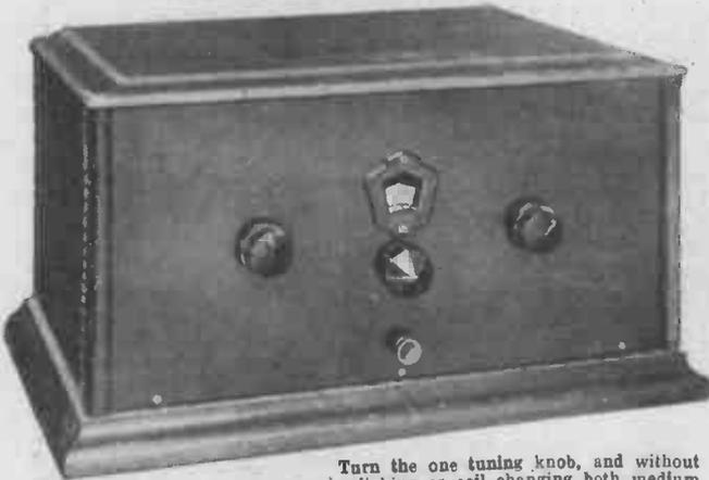
Turn the one tuning knob, and without switching or coil changing both medium and long broadcasting wave-lengths are covered. The same controls are used for short-wave reception.
