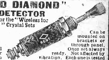
Can be mounted on brackets or through panel. Once set always ready. Not affected by vibration. Each one is tested on broadcast before despatch.
