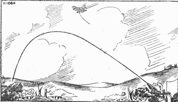
An extremely useful job for radio-equipped aeroplanes is to "spot" for the big guns. The observer in the machine wirelesses to the gunners and tells them if their shells are hitting the mark, and gives them information that will assist in finding the range.
