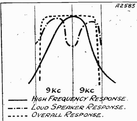
Capt. Eckersley suggests that the peak tuning given by ordinary coil and condenser arrangements is "the thing for modern needs," as it tends to "correct" the response of the average modern loudspeaker or, if you prefer it, vice-versa. You see by the "dash dot" curve that a loudspeaker deals less efficiently with the low notes and that these represent just that part of the "audio" range of frequencies which "peak tuning" emphasises.
