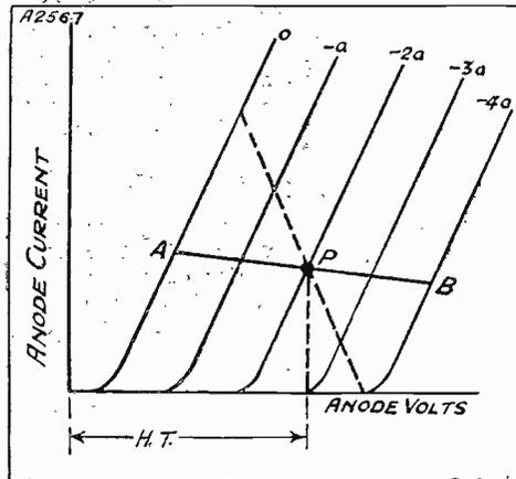
This sketch illustrates how a high anode impedance prevents bottom bending, as explained in the reply to E. T. of Cricklewood.
