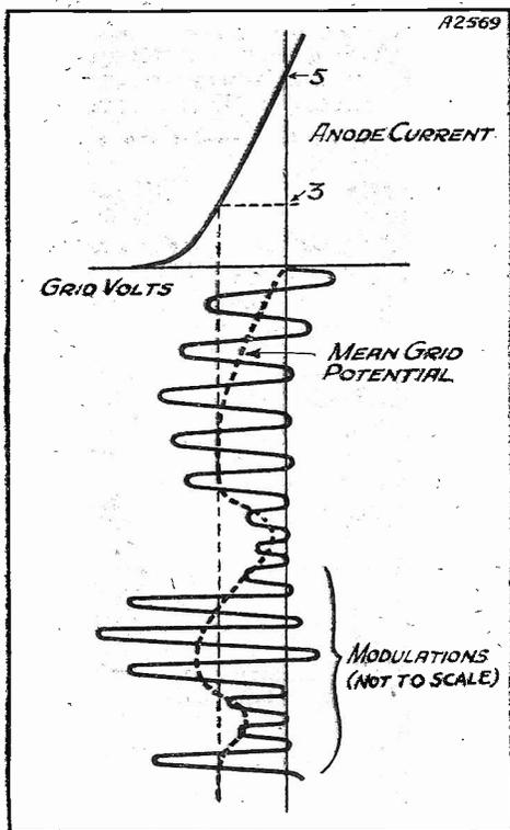
With the aid of this diagram Capt. Eckersley explains to J.M. why the anode current of a grid detector falls when a station is tuned in.
