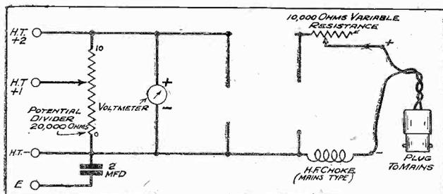
This is a simple unit for deriving H.T. from D.C. mains, but three of the "components" have been omitted. Can you fill them in correctly? LOOK OUT FOR THE ANSWERING DIAGRAM NEXT WEEK.
