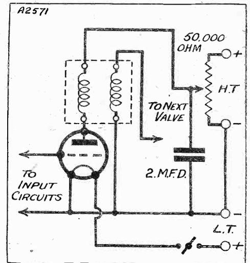
This diagram illustrates a method of providing the 1st detector of a super-het. with a variable H.T. tapping.
