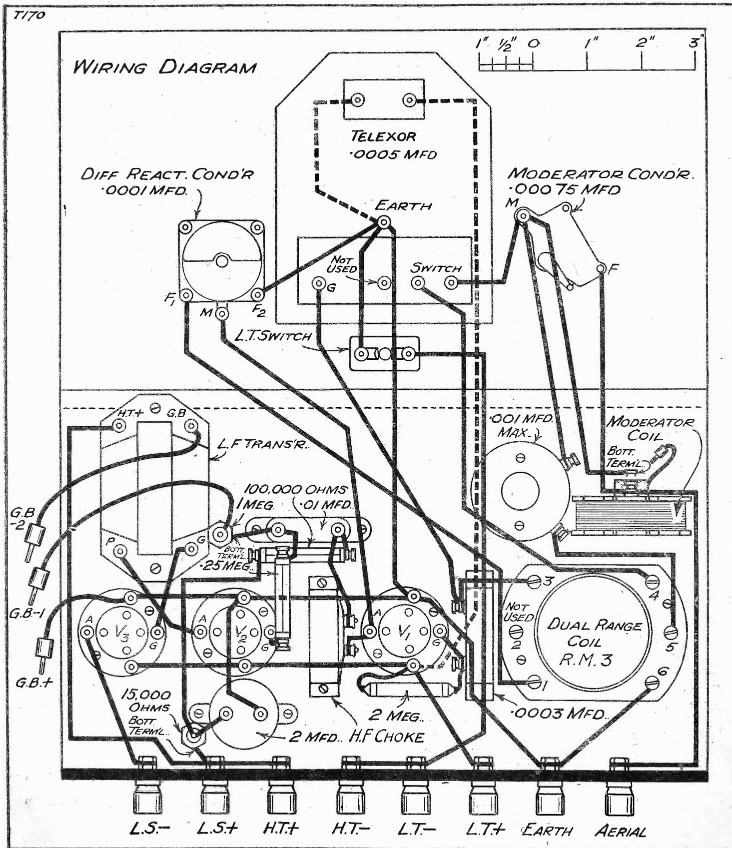
The dotted lines indicate the dial-light leads. Constructors should note that the L.T. switch must be fixed and wired before mounting the "Telexor."
