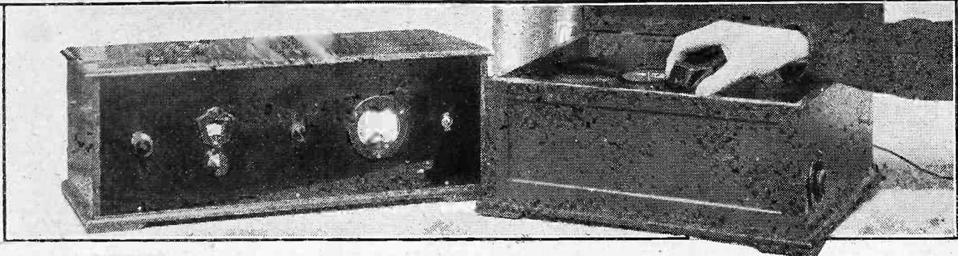
THE question of operating a radio-gramophone from batteries is always cropping up, and last time in these notes I mentioned that there were two ways out of the output voltage problem—to use either push-pull or one of the new pentodes.
