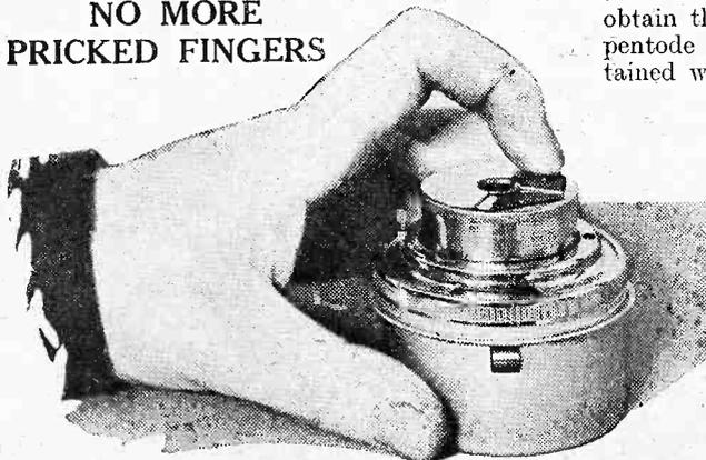
Here is the latest automatic needle-holder which obviates the need for fiddling about in a box of needles, with the usual physical discomfort from the sharp points. By pressing down the cylinder a needle is brought up on a horizontal "lift," while used needles are deposited in the large container surrounding the central cylinder.
