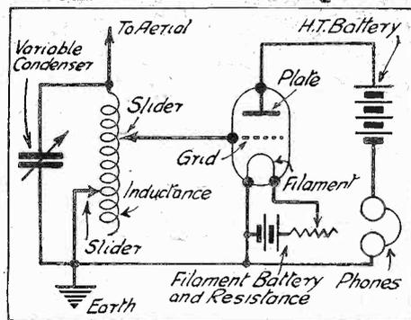
This ten-year-old one-valver had the telephones connected to H.T. negative, and used no grid-condenser or leak! A modern one-valver would knock spots off it!
