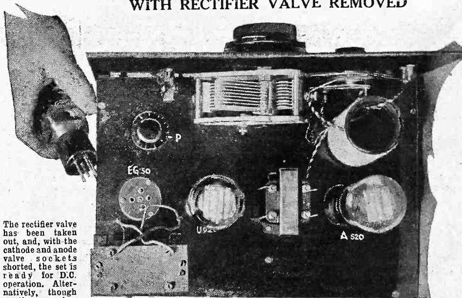
The rectifier valve has been taken out, and, with the cathode and anode valve sockets shorted, the set is ready for D.C. operation. Alternatively, though wasting a valve, the set can be used on D.C. with the rectifier *in situ*. The letters (with the exception of P, the potentiometer) refer to the types of valves used in the set. Note the copper "fishing net" over the bulb of the detector.
