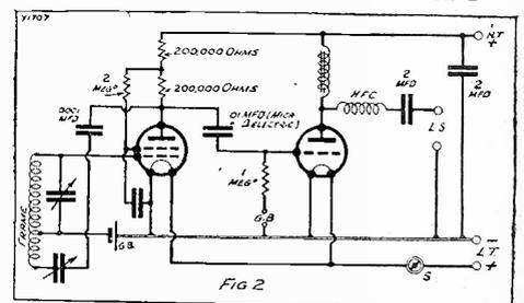
Greater sensitivity can often be obtained by using an S.G. detector. The screening-grid voltage is critical, but the arrangement of resistances shown here ensures that it will be correct.
