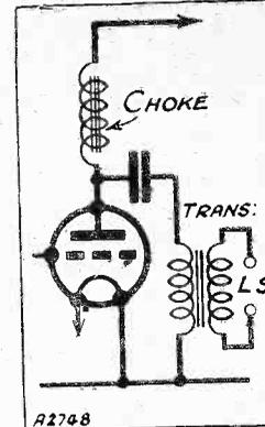
Note how choke and transformer both play their part in this Speaker coupling recommended by Mr. Rampton.
