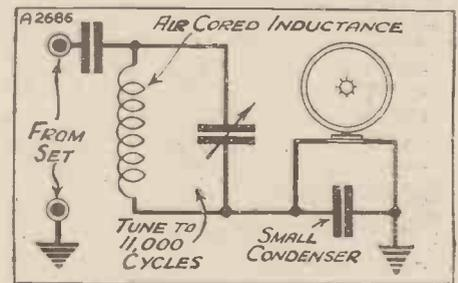
A tuned circuit in the loudspeaker lead is an alternative scheme to that shown in the opposite diagram.
