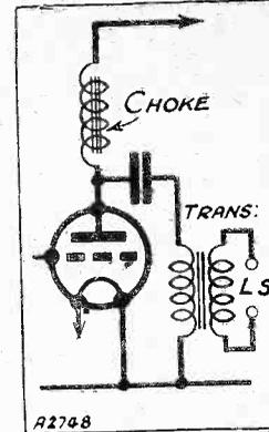
Note how choke and transformer both play their part in this Speaker coupling recommended by Mr. Rampton.
