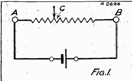
If a resistance is connected across a battery as illustrated above, any desired voltage, up to the maximum of the battery, can be tapped off with the slider. Hence its name—a potential divider.
