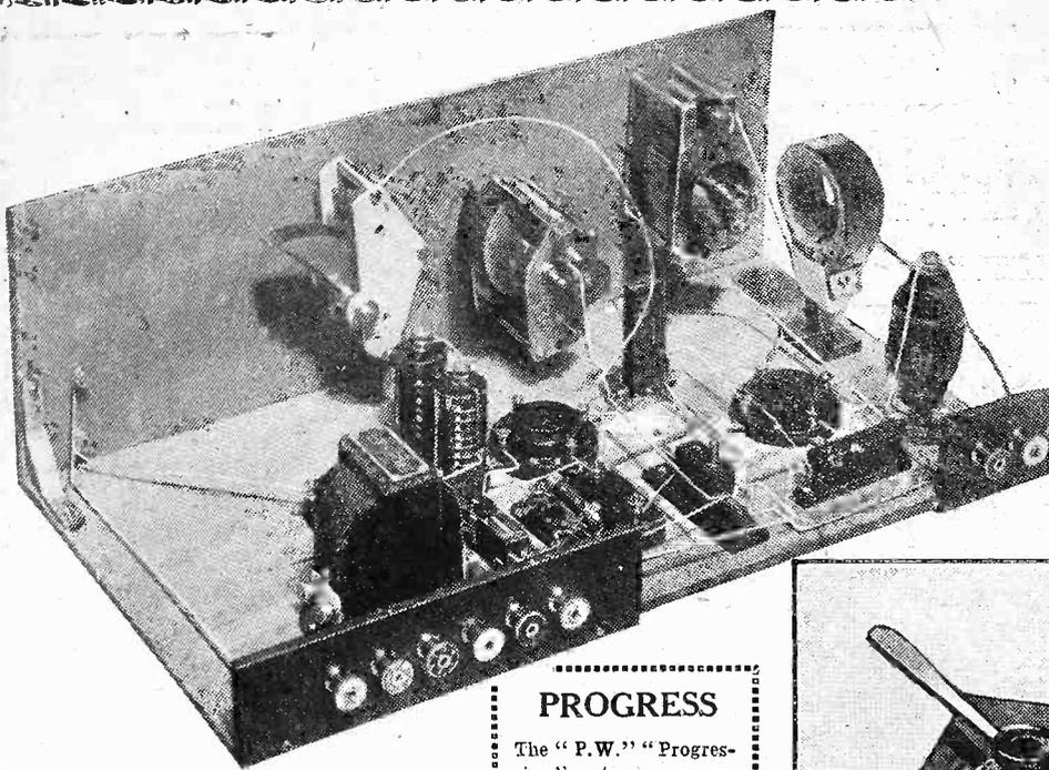
both an H.F. and an L.F. amplifier. Moreover, by means of switches the valve could be cut out of circuit and the set used as a crystal receiver. And remembering how much L.T. current the very precious and delicate "bright emitter" valve of 1922 took,
