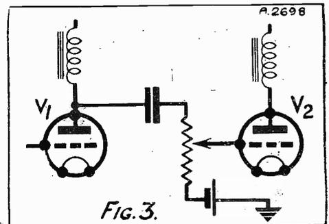
When a potential divider is used in this manner as an L.F. volume control there will be no voltage variation due to load. This is because for all practical purposes there is no current flowing in the grid circuit.
