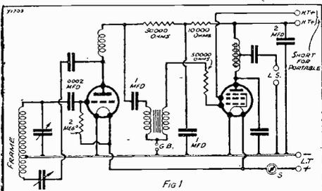
Although two valves only are used in this circuit, it will give excellent loudspeaker results when operated in conjunction with either a frame or a small outdoor aerial.
