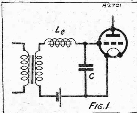
What is known as the magnetic leakage of a transformer can be considered as an inductance in series with the secondary winding. Unless properly used, this inductance can completely spoil the response curve of a transformer.
