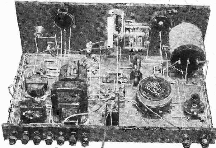
A combination of unique "P.W." features appeared in the "Comet." These were the "P.W." Dual-Range Coil, which later was to sell and be home-constructed by the hundred thousand; "Flexicoupling," a forerunner of the "Moderator"; and an up-to-date application of the "P.W." Progressive principle.
