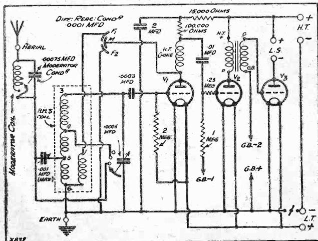
The Moderator coil and condenser bring the aerial circuit into resonance at "medium-wave" frequencies, and thus enable the maximum of power to be developed.
