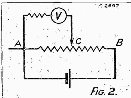
If current is taken from a potential divider, the voltage across that section of the resistance which is in use will drop considerably. (This explains why misleading readings are obtained when cheap low-resistance voltmeters are used for testing mains units employing such an arrangement.)
