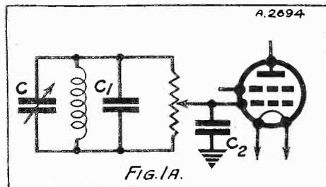
Here are the two diagrams to which Capt. Eckersley refers above. He explains how such a method of high-frequency volume control is not satisfactory, since its regulation is influenced by several inconstant factors.
