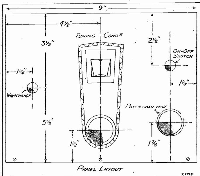
Full details for drilling the panel are given in this diagram. Although the tuning knob and escutcheon look somewhat complicated, it will probably surprise you to know that three holes only are required.
