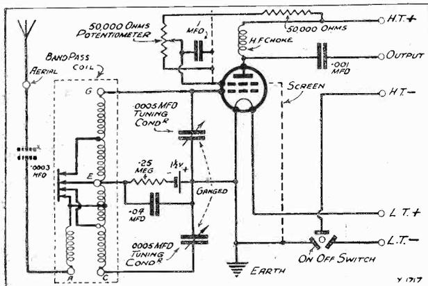
It will be seen from this circuit that the unit comprises a complete stage of S.G., H.F. amplification, with band-pass tuning. The output terminal connects up to the aerial terminal of your set, and you can use the same batteries or mains unit for receiver and "Booster."
