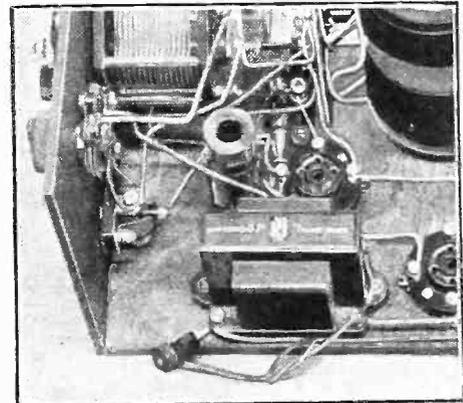
When wiring the volume control in a circuit such as this, take care to keep the leads from the components concerned as short as possible. That is, if you want pleasing results!
