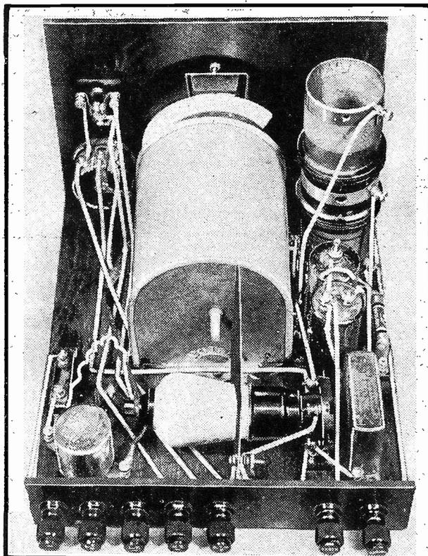
The two-gang condenser is totally enclosed in the metal can seen here, and besides effectively screening this vital component, it assists considerably in separating the anode circuit of the S.G. valve from the rest of the unit.
