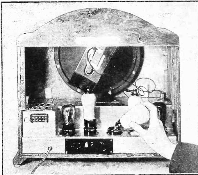
This back view of the set shows how the valves are arranged, and gives a good idea of the completeness of the screening.
