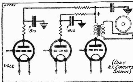
The fundamental cure for motor-boating is to decouple thoroughly the different anode circuits. Such decoupling applies particularly to the detector valve.
