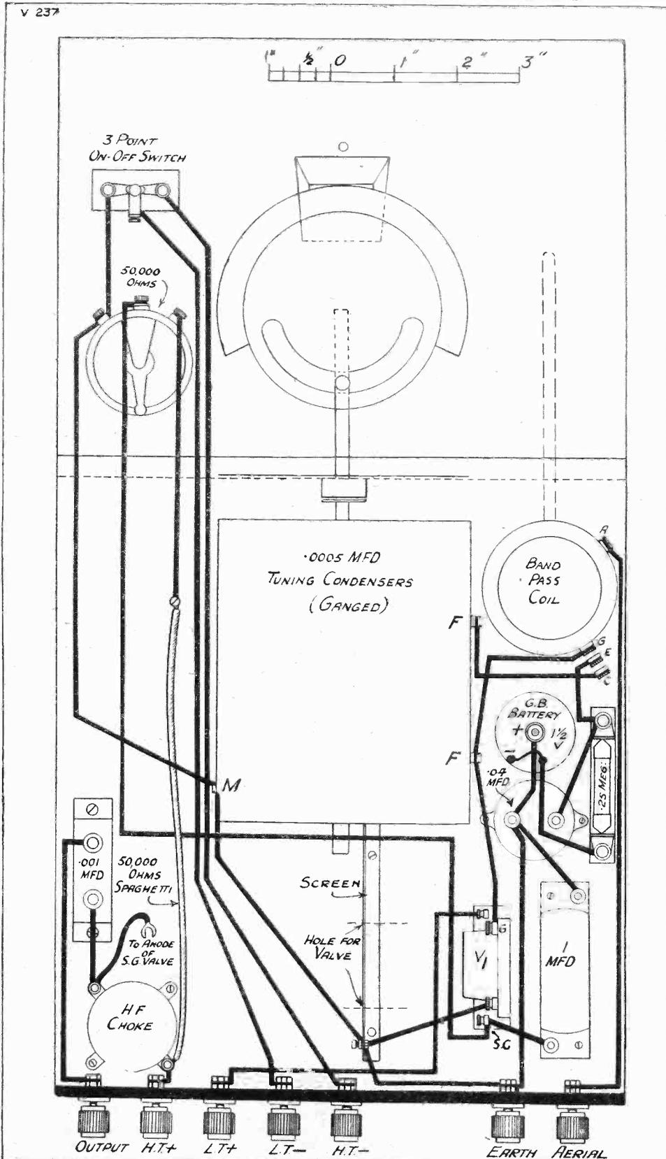
The wiring is particularly simple, there being a mere handful of connections. When joining up the "Square-Peak" coil you will find the lettering for the various terminals on the metal band round its middle, and not near the terminals, as you might at first expect.
