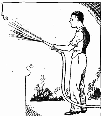
In order to obtain a powerful jet from a hose nozzle it is necessary for the pressure of water to be high. If the pressure of water is low only a trickle will flow from the nozzle of the hose.
