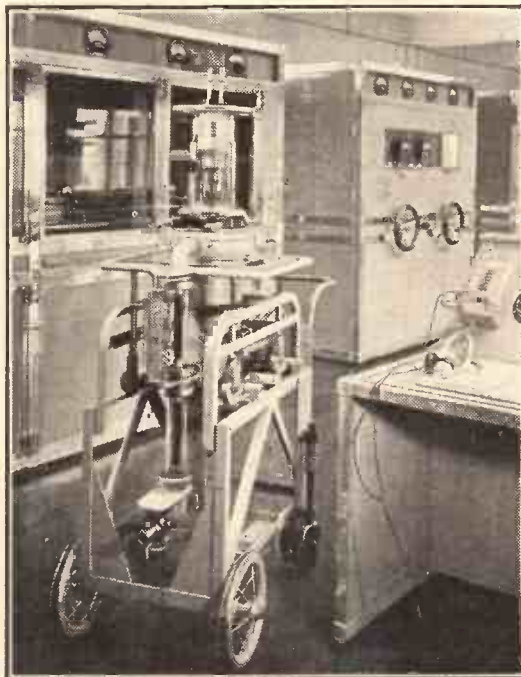
One of the big output valves used at Droitwich ready for fitting into the transmitter. These valves are each capable of a maximum output of 50 kw. Owing to their weight and physical size a special trolley is provided for wheeling them into position, with a jack to lift them on to their seatings.
