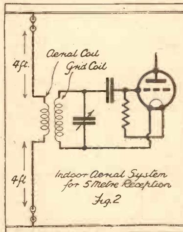
Fig. 2.—A resonant aerial of this type gives excellent results on the 5-metre band, and may generally be accommodated indoors. As a refinement the coupling between the two coils may be loosened and the aerial coil, as well as the grid coil, tuned.
