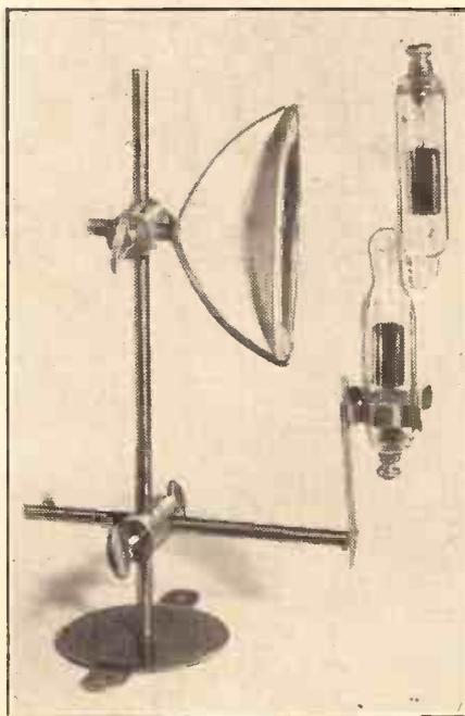
The "T.I." lamp, with its stand and reflecting mirror. The pictures obtained with this outfit are much brighter than those given by an ordinary neon-tube light source.
