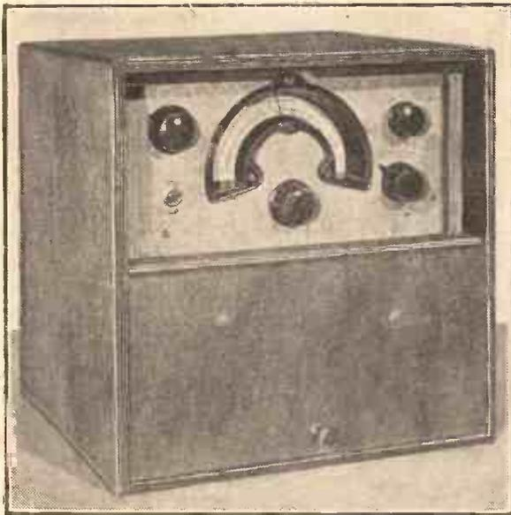
The completed receiver, showing the controls for the broadcast section. The short-wave controls are immediately below the broadcast panel, underneath the hinged cover.
