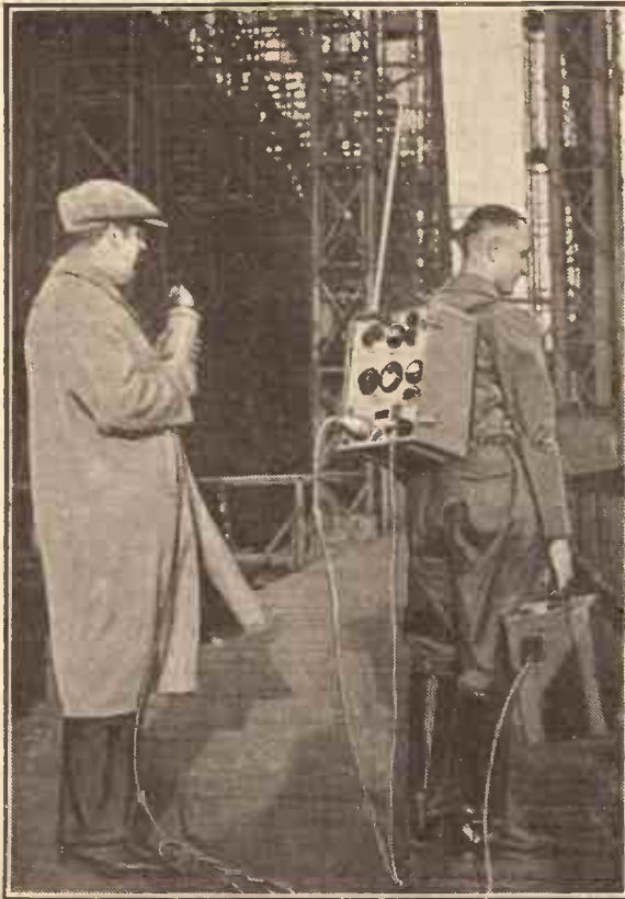
How the radio reporter works. The transmitter is entirely complete so that the engineer and commentator are free to go anywhere.
