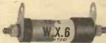
The "Westector"—a small metal rectifier designed for use as a second detector in superhets.
