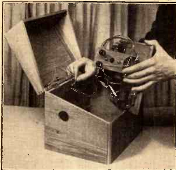
The battery leads are grouped together and pass through a small hole in the back of the cabinet. These leads should be threaded through before the set itself is finally placed into position.
