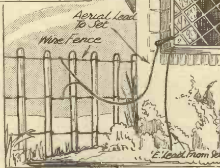
Fig. 3. How wire fences with wooden posts can be utilised.
