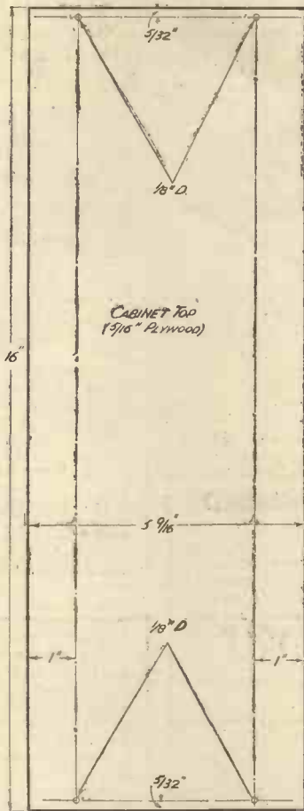
Fig. 2.—Details for preparing the top of the "Easy-Cabinet." Dimensions for the side pieces are given in the diagram on page 594.
