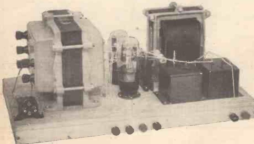
The power-pack of the 14-watt receiver. Two rectifiers are employed.
