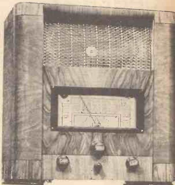
An H.M.V. receiver with visual tuning. It covers the short waves in addition to the medium and long, and utilises a six-valve circuit. The price is 14½ guineas.
