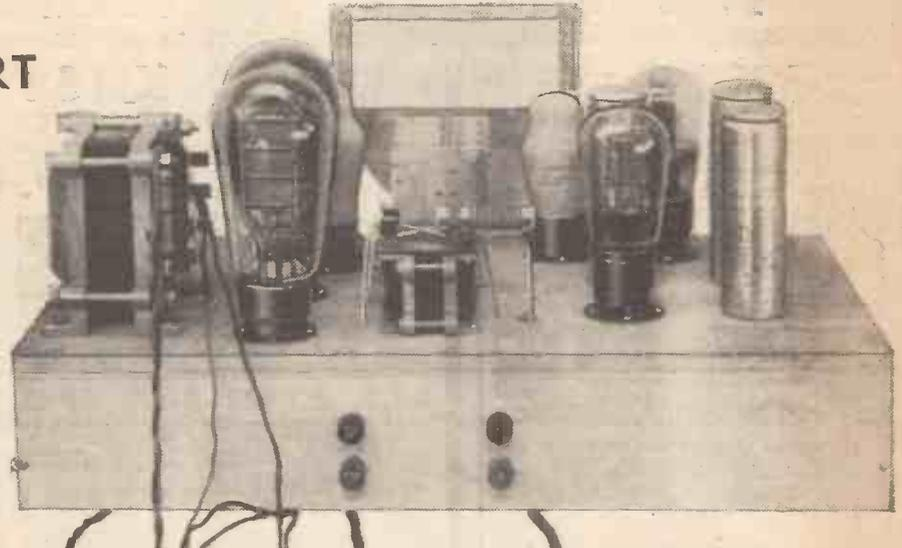
The radio and L.F. amplifier unit. A bandpass H.F. input circuit is used and the power grid detector is resistance coupled to an L.F. valve which in turn is coupled to two large output valves in push-pull.
