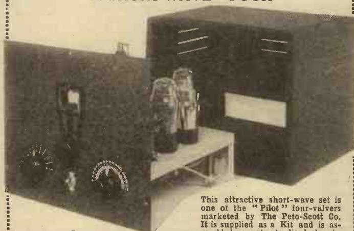
This attractive short-wave set is one of the “Pilot” four-valvers marketed by The Peto-Scott Co. It is supplied as a Kit and is assembled on a standardised chassis,
