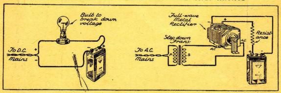
the accumula tor is connected up correctly from the polarity point of view. With D.C mains, a resistance which may conveniently be an electric lamp is needed. In "Datagram" No. 4 will be found a list of lamps with their wattages and voltages, showing the currents they pass. With A.C. mains a transformer and rectifier are required, a Westinghouse metal rectifier being the most practicable. It is not advisable to omit the resistance shown
