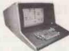
computer with color graphics, 12" CRT; 101 Key Keyboard, including color and numeric clusters; File Handling DISK BASIC; 32 lines 64 characters per line. Mini Disk drive with
