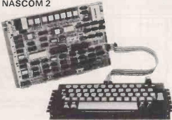
Kit includes all parts to build CPU board which has resident 8K microsoft BASIC and 2K NAS-SYS 1 monitor for machine code programming. Included with kit is a fully assembled LICON QWERTY SOLID STATE KEYBOARD specially designed to exploit the potential of the NAS-SYS monitor. Other interfaces include video to monitor or domestic TV, Kansas City standard cassette interface (300/1200 baud) or RS232/20mA teletype interface.
