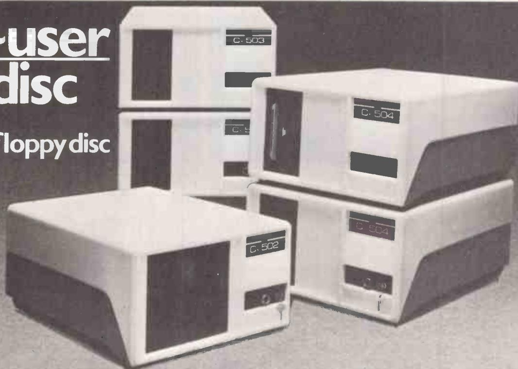
The Transdata Cx 500 family of Business and Scientific Microcomputers features upgrade potential from the Cx 502 single user 8" floppy disc system to the Cx 504 multi-user hard disc system. All Cx 500 systems feature an advanced multi-processor architecture which results in higher performance with simple expansion.
