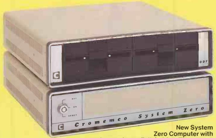
**New System Zero Computer with quad-capacity DDF disk drive. The system includes built-in diagnostics for a quick system test of memory, controller and disk drives**
