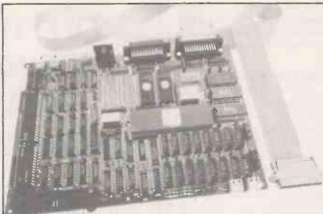
The Profi Kit 2 is a 16-bit single-board computer using the Motorola 68000 processor. Designed by Force in Germany, the board is an upgrade of the Profi Kit 1. It includes 128K of RAM and serial, parallel and cassette ports. Profi Kit 2 costs £499 plus VAT. Contact Microsystem Services, PO Box 37, Lincoln Road, Cressex Industrial Estate, High Wycombe, Buckinghamshire HP12 3XJ. Telephone: (0494) 41661. □
