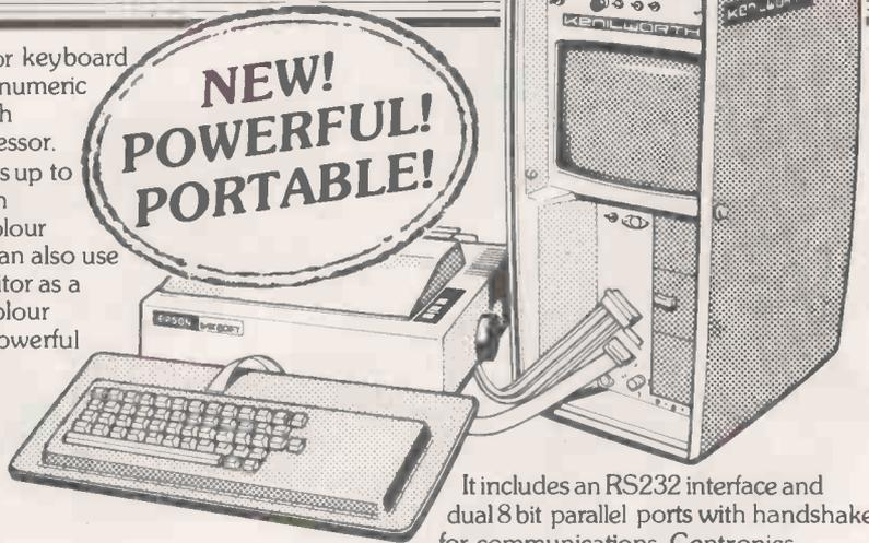
It includes an RS232 interface and dual 8 bit parallel ports with handshake for communications. Centronics standard printers etc.
