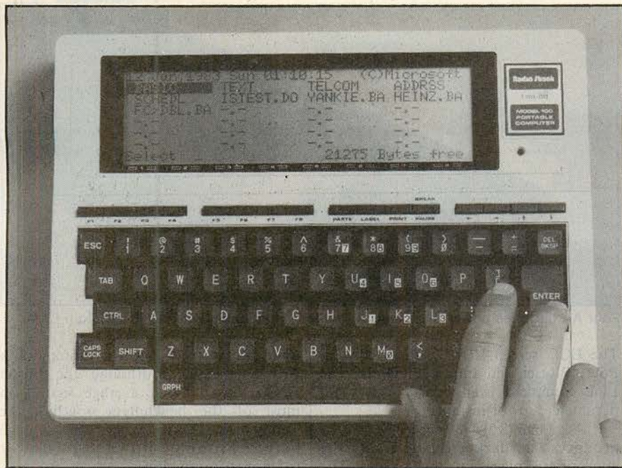
Turning on the machine brings up the main menu, including date and time.
