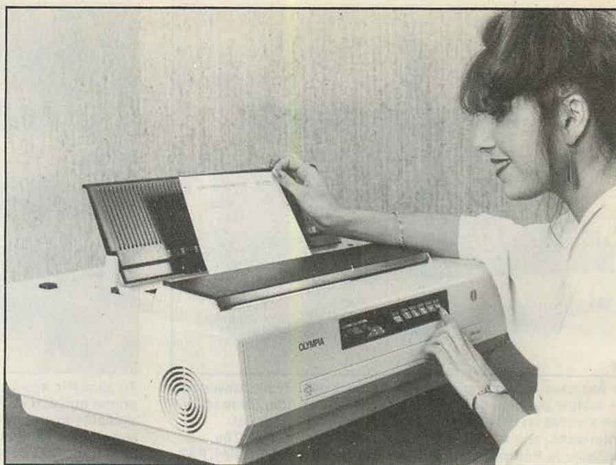
Daisywheel printers are required for high-quality correspondence, but tend to be either very slow or very expensive. The Olympia ESW-3000RO offers a good compromise: it prints bidirectionally at up to 50cps and costs around £1,100 plus VAT. Tractor feed and a single-sheet feeder are optional extras. The supplier is Olympia Business Machines Ltd, Olympia House, 199-205 Old Marylebone Road, London NW1 5QS.
