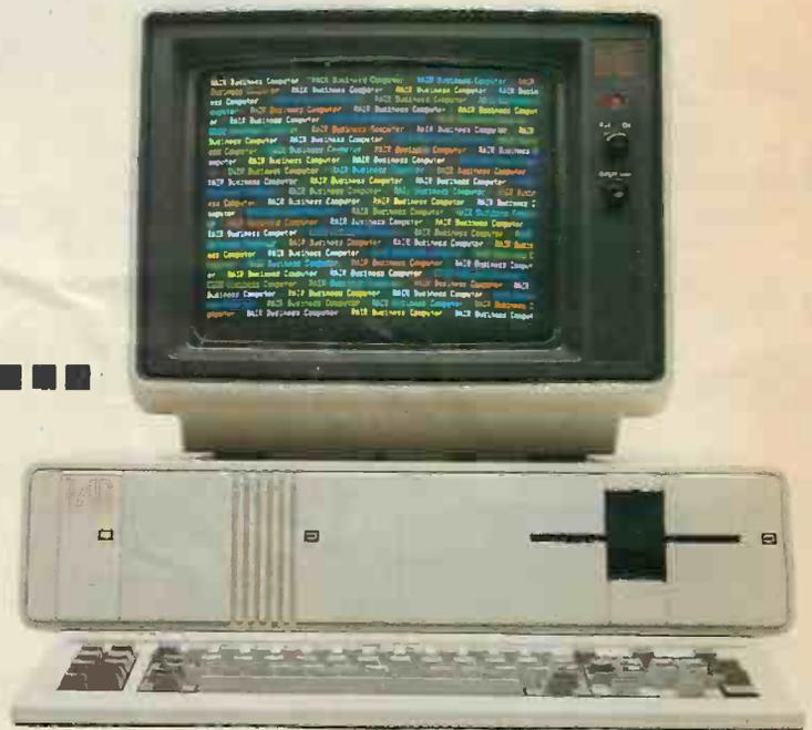
The RAIR Business Computer incorporates both 16-bit and 8-bit microprocessors, up to 1024K bytes of user memory, 20M bytes of disk storage, and supports up to four workstations running CP/M\*, MP/M\* or MS-DOS\* compatible software.
