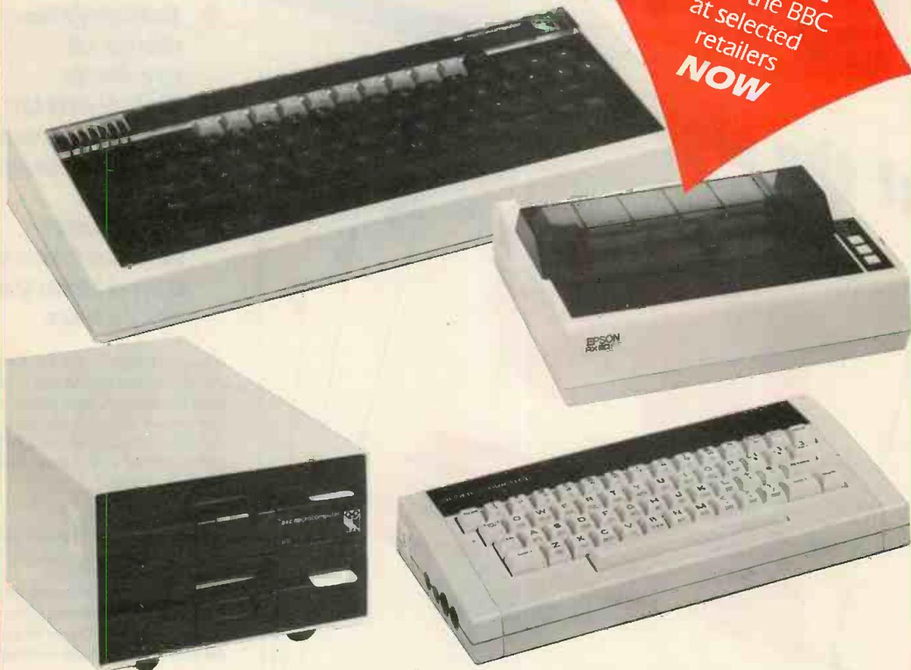
A full colour 32K ROM computer with text and graphics modes up to 640 x 256 graphics and 80 column text screen, extended Microsoft basic, built in assembler 1 MHZ and tube interface, sideways ROM, RS 423, A/D converter.
