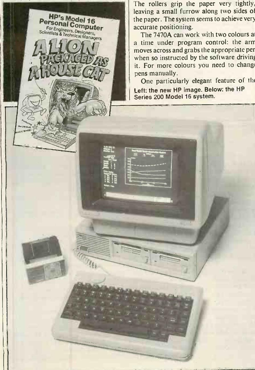
Left: the new HP image. Below: the HP Series 200 Model 16 system.
