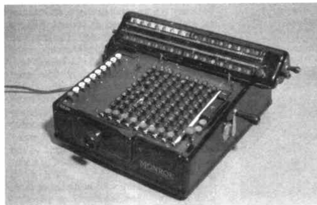
Monroe's "Full Automatic" calculating machine, 1922, the first machine to offer fully automatic multiplication and division. Courtesy Science Museum/Science and Society Picture Library.
