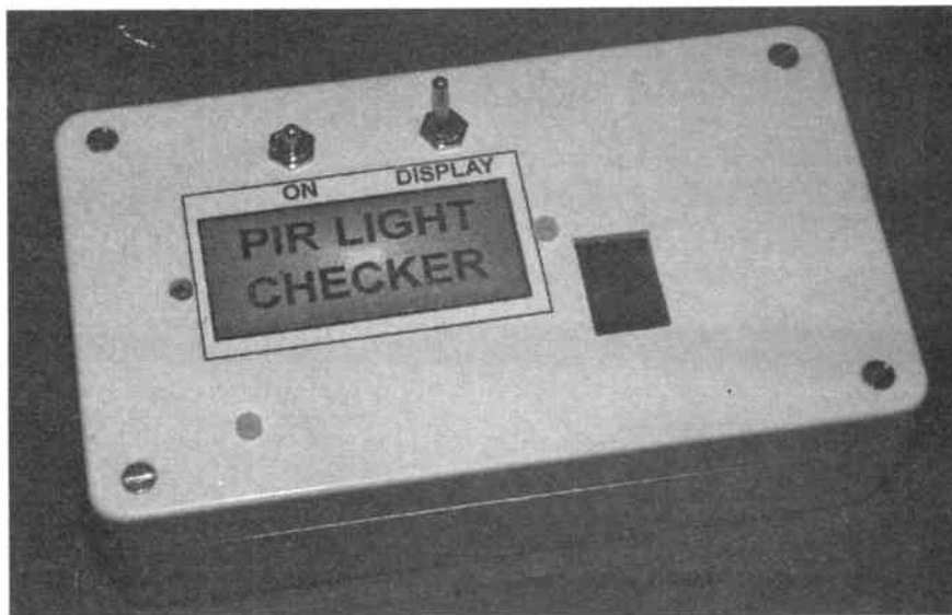
Completed PIR Light Checker front panel layout. The display cutout has been backed with a piece of translucent filter material.
