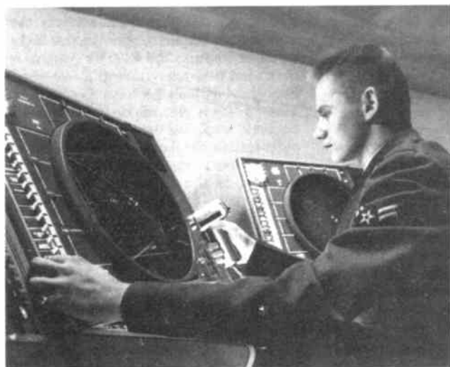
Two of the ballistic track monitors of Sage, the massive US military computer that helped defend the Western World during the Cold War. Courtesy of IBM.
