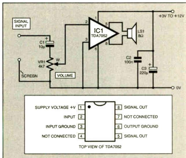
Fig. 3. Circuit diagram and pinout details for the TDA7052 Amp. See left for performance data.
