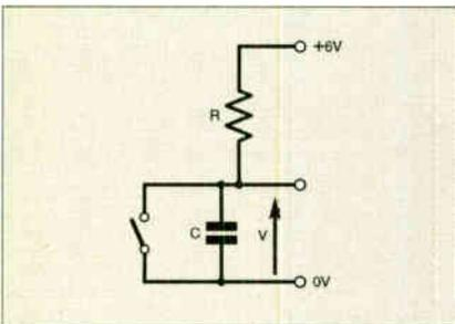
**Fig.3. Simple circuit to demonstrate capacitor charging.**
