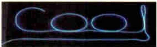
Neon string uses the principle of Electroluminescence. At just 2.5mm in diameter it produces a bright, crisp light, but no heat.
