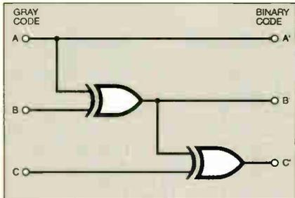
Fig.7.9. Gray code to binary code converter.
