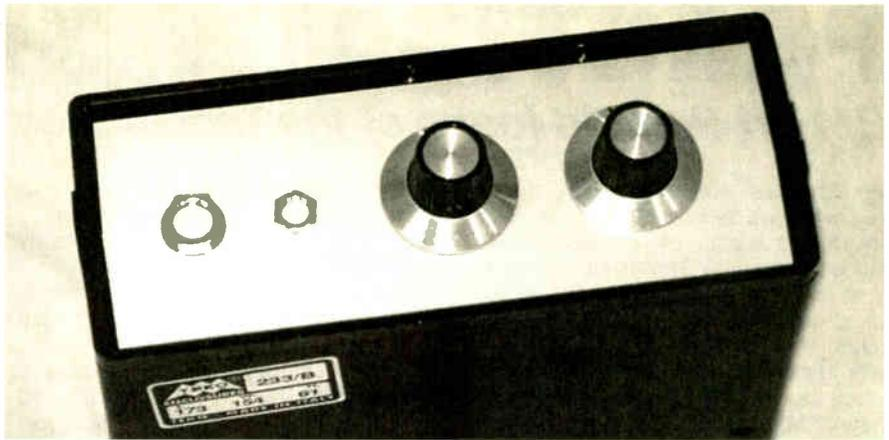
*Position control knobs, etc., on the front panel and move them around to find the best layout.*
