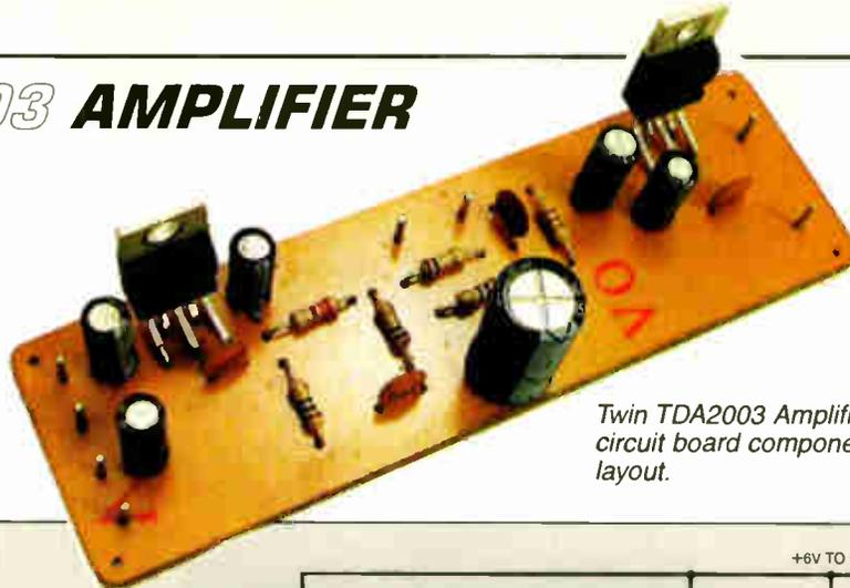
Twin TDA2003 Amplifier circuit board component layout.
