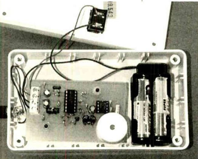
Positioning of components inside the plastic case.
