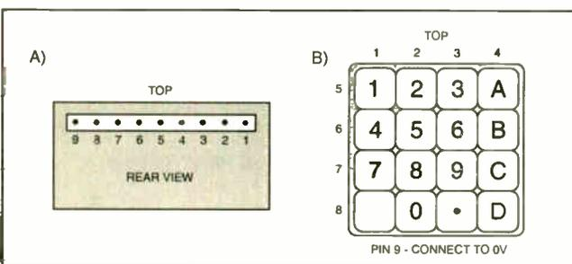
Fig.9. Keypad connection details.
