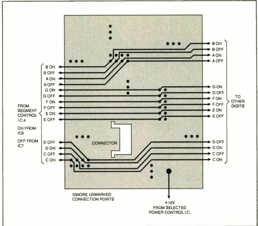
Fig.13. Wiring details for a single digit.
