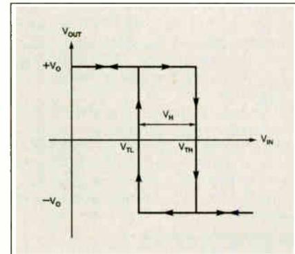
Fig.7.2. Response of an inverting regenerative comparator.
