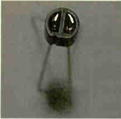
Example of a reflective sensor, as used in the wind vane.
