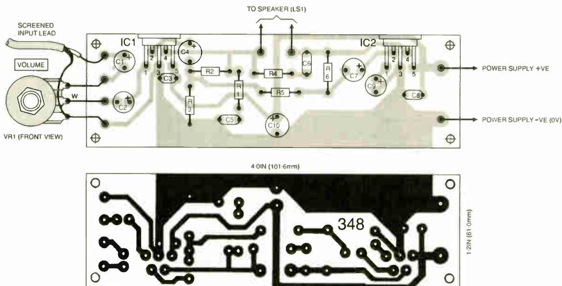
The printed circuit board component layout, wiring and copper foil master are detailed in Fig.12. Again, combined or separate heatsinks must be fitted to the integrated circuit's metal tabs. The p.c.b. is obtainable from the *EPE PCB Service*, code 348 (Twin TDA22003).
