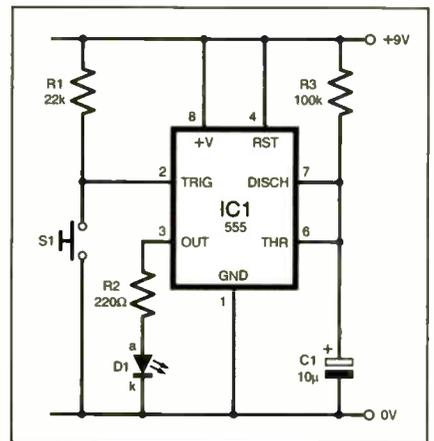
Fig.4. Circuit for testing the re-triggerability of a 555 monostable. Keep switch S1 closed for several seconds and observe the l.e.d. D1.
