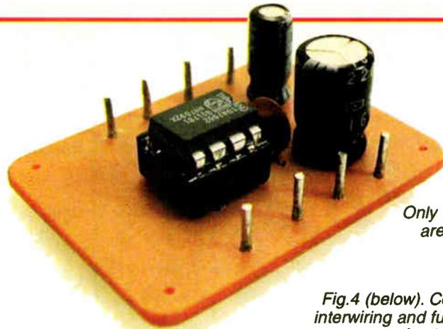
Only four components are mounted on the TDA7052 p.c.b.
