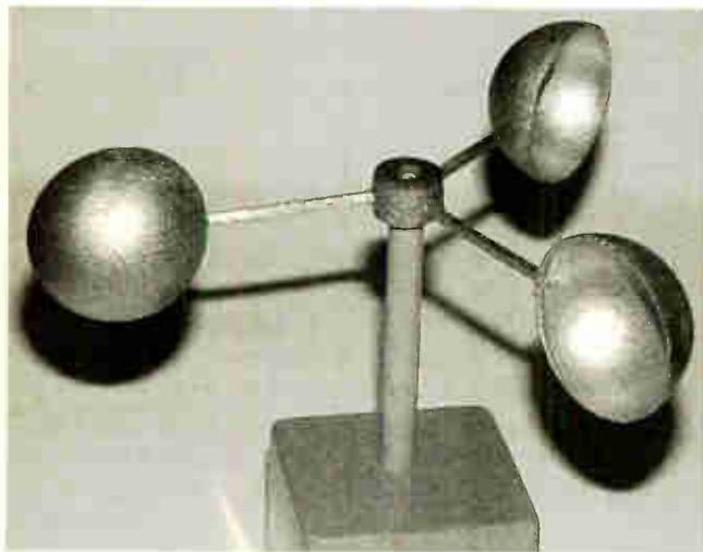
Prototype "homemade" anemometer assembly.
