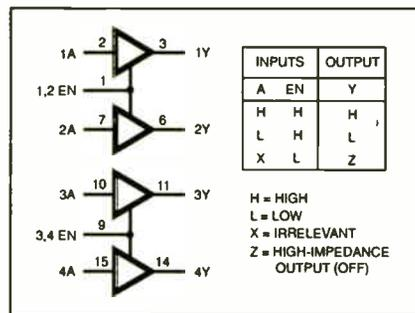
Fig.4. L293DN pinouts and logic table.
