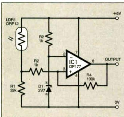
Fig.7.20. Comparator circuit with hysteresis.
