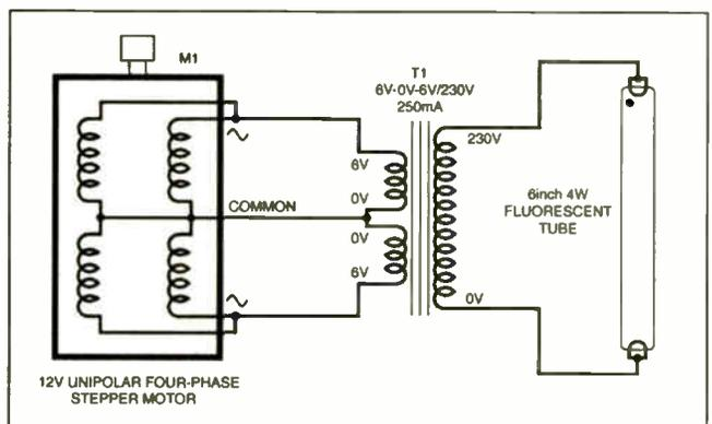
Fig.2. Emergency Light circuit diagram.
