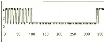
Fig.7.19. Typical noisy output from circuit in Fig.7.18.
