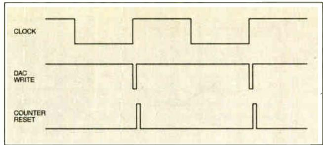
Fig.7.17 (above). Timing diagram of anemometer circuit.
