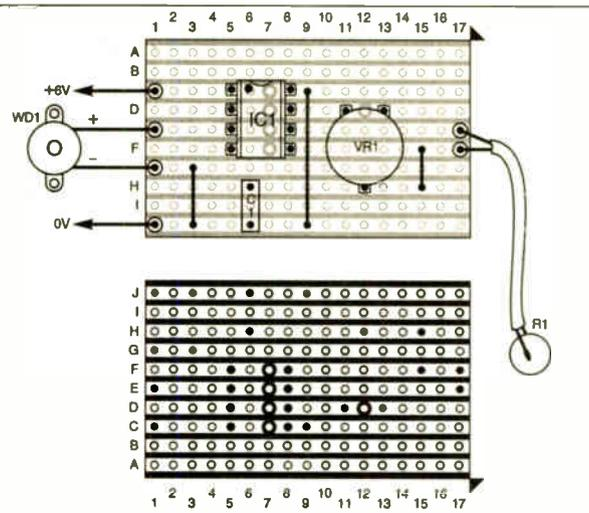
Fig. 10. Stripboard layout for the Freezer Alarm.
