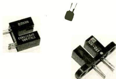
Typical examples of slotted and reflective photosensors.
