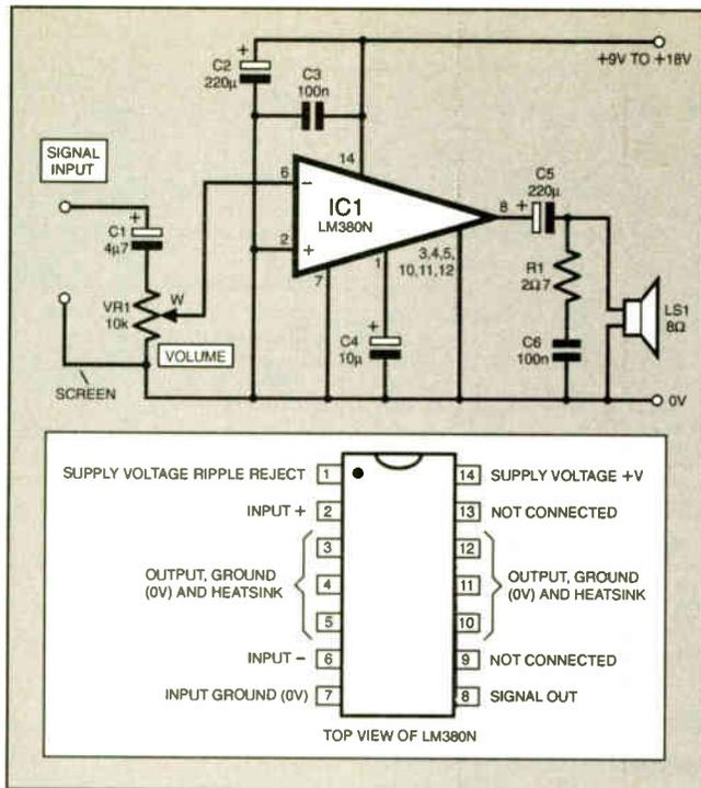
Fig.7. Circuit diagram for the LM380N Amplifier.
