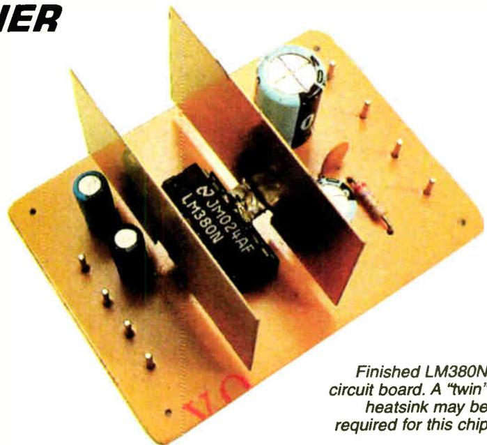
Finished LM380N circuit board. A "twin" heatsink may be required for this chip
