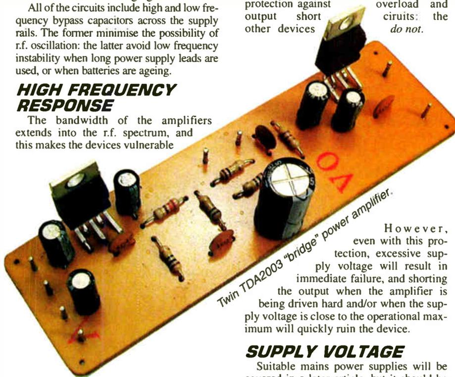
However, even with this protection, excessive supply voltage will result in immediate failure, and shorting the output when the amplifier is being driven hard and/or when the supply voltage is close to the operational maximum will quickly ruin the device.
