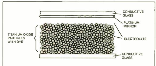
Fig.1. Structure of the solar cell using organic dye and titanium oxide particles.
