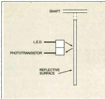
Fig.7.14. Reflective photosensor.
