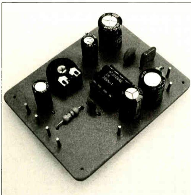
Completed LM386N-1 circuit board.
