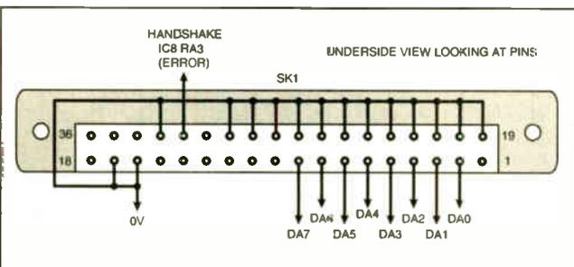
Fig.10. Connections to a 36-way D-type Centronics female connector used in conjunction with a standard PC parallel port cable.
