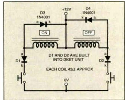
Fig.1. Basic circuit for controlling one segment.
