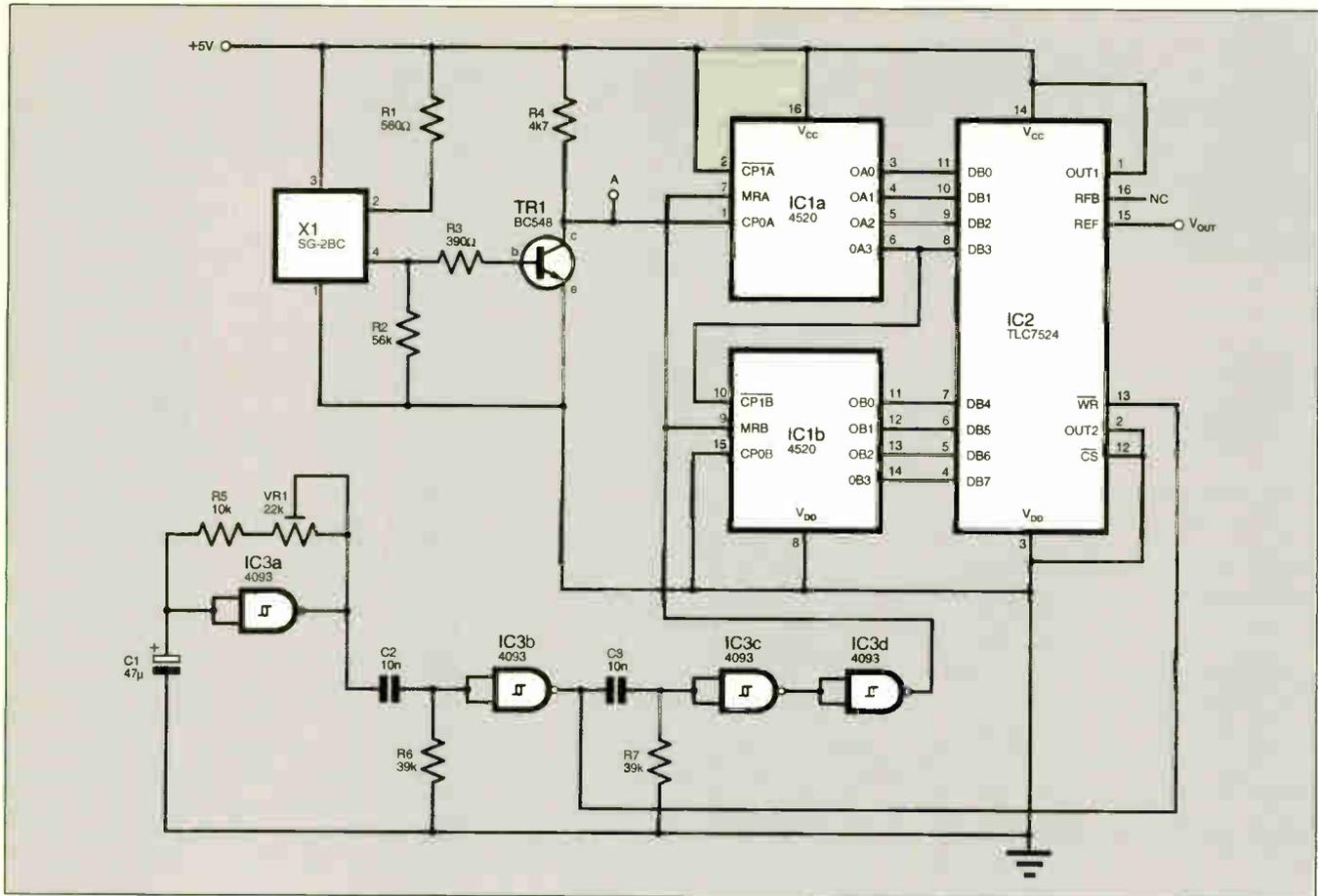
Fig.7.22. Circuit diagram for the anemometer.
