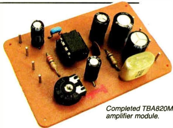
Completed TBA820M amplifier module.
