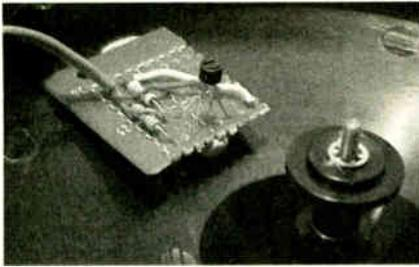
Mounting of the sensor in the prototype anemometer.
