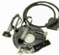
Currently learning about microcontrollers? Need to do something more than flash a LED or sound a buzzer? The ABC Mini 'Hotchip' Board is based on Atmel's AVR 8535 RISC technology and will interest both the beginner and expert alike. Beginners will find that they can write and test a simple program, using the BASIC programming language, within an hour or two of connecting it up.
