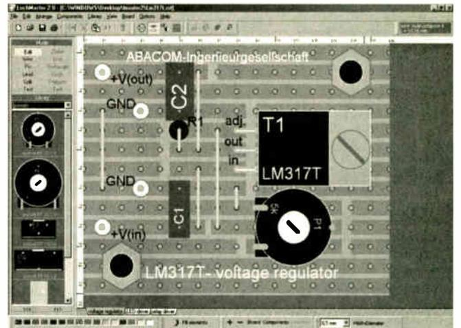
Top view of a small sample board created in Lochmaster 2.0.
