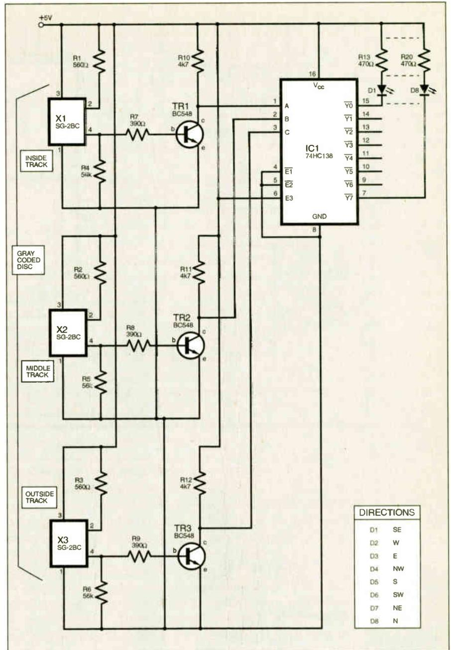
Fig.7.26. Circuit diagram for the wind direction sensor.
