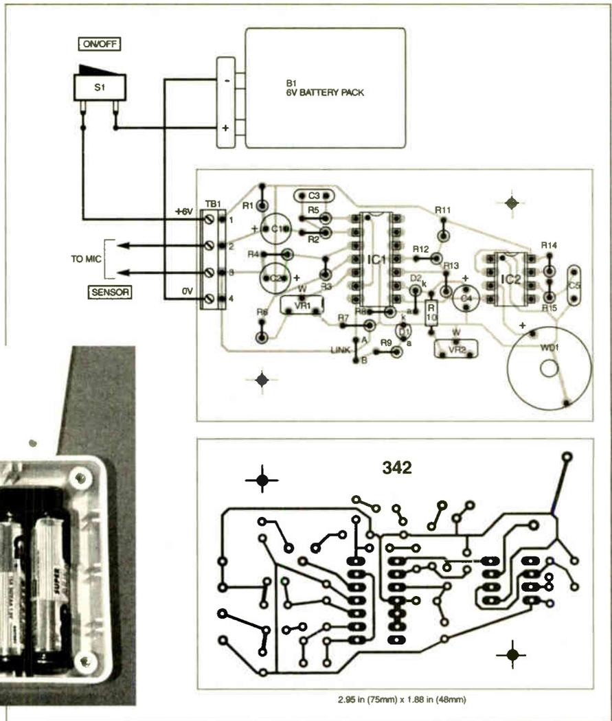
Fig.3. Printed circuit board component layout, full-size copper foil master and wiring to off-board components.
