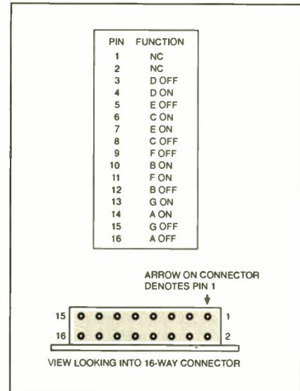
Fig.12. Pinouts for the connector mounted as part of the digit assembly.
