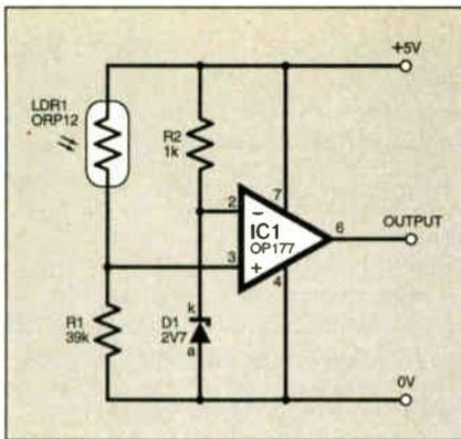
Fig.7.18. Comparator circuit without hysteresis.
