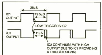
Fig.5. The monostable IC2 will continue to give a High output for as long as its trigger pin is held low by IC1. IC2 can therefore be used as an inverter.
