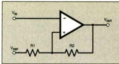
Fig.7.5. Inverting regenerative comparator circuit.
