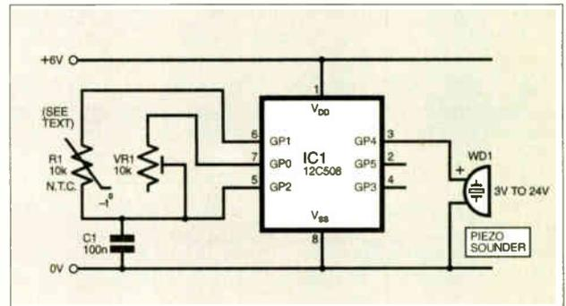
Fig.2 (right). Circuit diagram for the Freezer Alarm.
