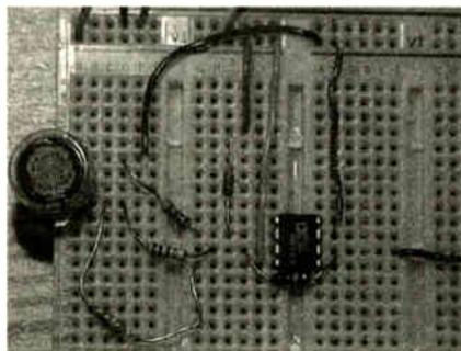
Breadboard assembly for circuit in Fig.7.20.
