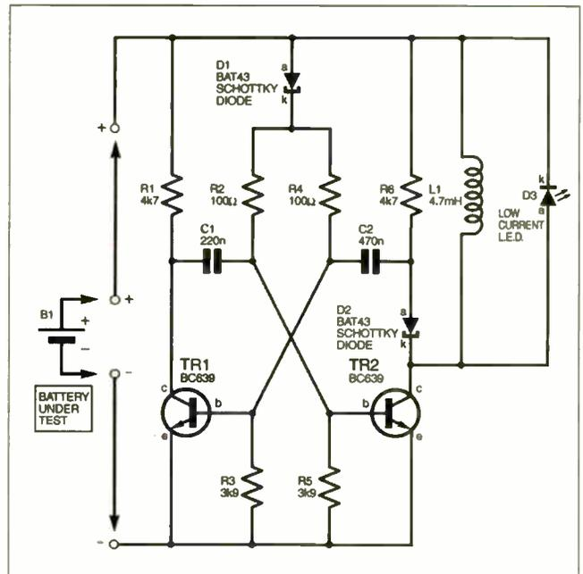
Fig.1. Circuit diagram for the Battery Discharger.
