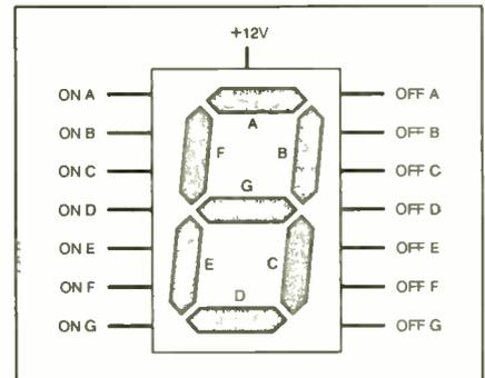
Fig.2. Each digit has 15 connections, 12V power input and two on-off controls for each segment.
