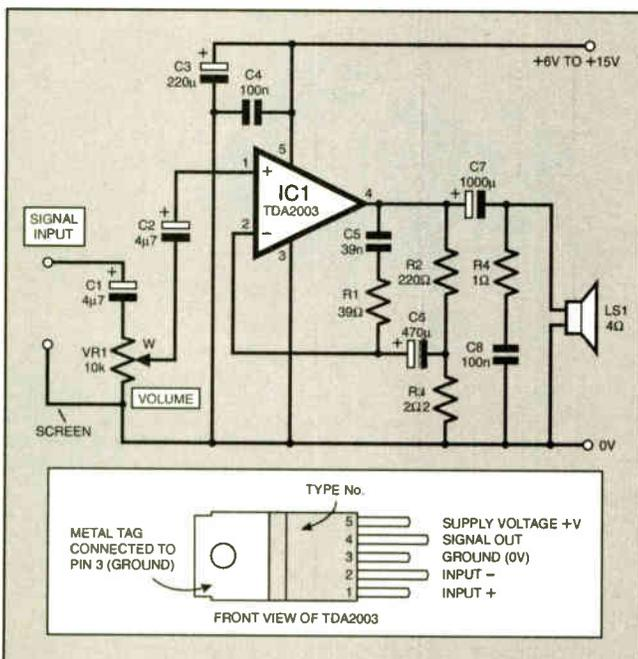
Fig.9. Circuit diagram for a single TDA2003 Amp.
