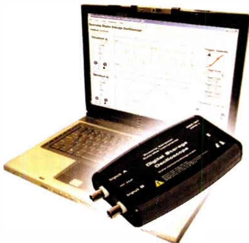
The DSO-101 is a general-purpose two-channel oscilloscope for teaching, development and debugging of electronic circuits. Channels A and B are sampled simultaneously and stored in oscilloscope memory before being sent for display to the host computer. Consequently, they are always time aligned and triggered from the same trigger signal.
