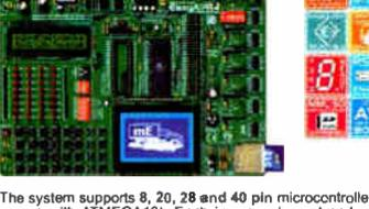
The system supports 8, 20, 28 and 40 pin microcontrollers (it comes with ATMEGA16). Each jumper, element and pin is clearly marked on the board. It is possible to test most of industrial needs on the system: temperature controllers, counters, timers etc. EasyAVR4 is an easy-to-use Atmel AVR development system. On-board USB 2.0 programmer makes your development easy. Examples in BASIC and Pascal language are provided with the board.
