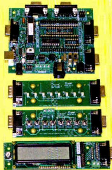
**E**-BLOCKS are dual purpose electronic modules that, in one role, enable users to learn about electronics and PIC programming. For experienced users they provide a means of quickly building and testing PIC, ARM, AVR or CPLD based designs. The E-Block concept is very simple, and it is based on programming modules that can also be used as the basis of prototype units.
