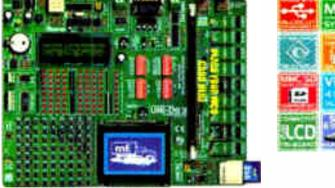
The system supports PIC, AVR, 8051, ARM and PSoC microcontrollers with a large number of peripherals. In order to continue working with different chip in the same development environment, you just need to switch a card. Uni-DS3 has many features that make your development easy. You can choose between USB or External Power supply. Each MCU card has its own USB 2.0 programmer!
