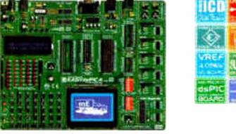
The system supports 18, 28 and 40 pin microcontrollers (it comes with dsPIC30F4013 general purpose microcontroller with internal 12-bit ADC). EasydsPIC4 has many features that make your development easy. Many of these already made examples in C, BASIC and PASCAL language guarantee successful use of the system. Ultra fast on-board programmer and mikroICD (In-circuit Debugger) enables very efficient debugging and faster prototype developing.
