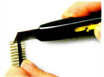
You can easily make 2-way and 4-way pin headers for JP1 and JP2-3 by cutting down a longer strip.
