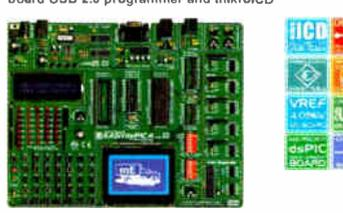
The system supports 18-, 28- and 40 pin microcontrollers (it comes with dsPIC30F4013 general purpose microcontroller with internal 12-bit ADC). EasydsPIC4 has many features that make your development easy. Many of these already made examples in C, BASIC and PASCAL language guarantee successful use of the system. Ultra fast on-board programmer and mikroICD (In-circuit Debugger) enables very efficient debugging and faster prototype developing.
