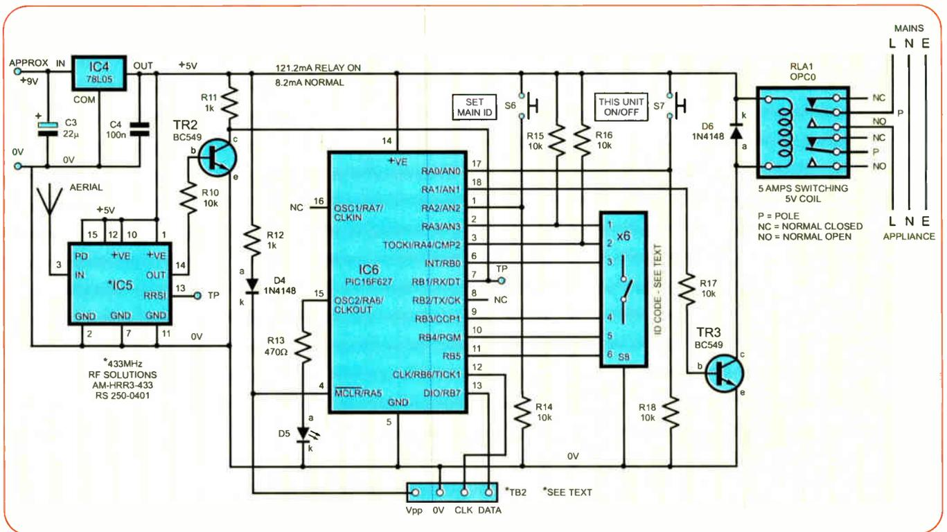
Fig.2. Circuit diagram for the remote receiver section of the Standby Power Saver
