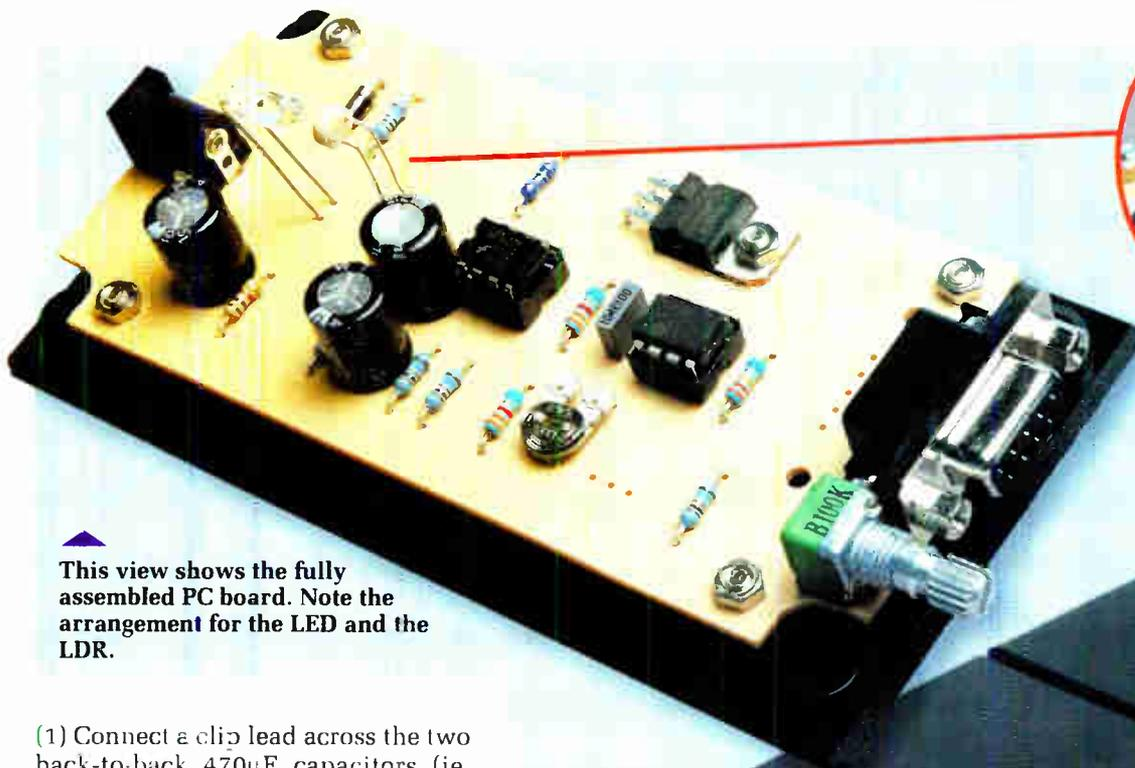
▲ This view shows the fully assembled PC board. Note the arrangement for the LED and the LDR.
