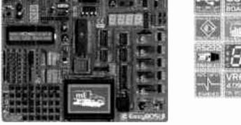
System is compatible with 14, 16, 20, 28 and 40 pin microcontrollers (it comes with AT89S8253). Also there are PLCC44 and PLCC32 sockets for 32 and 44 pin microcontrollers. USB 2.0 Programmer is supplied from the system and the programming can be done without taking the microcontroller out.
