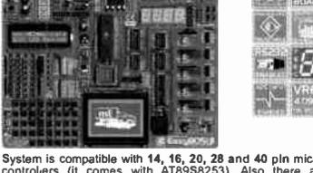
System is compatible with 14, 16, 20, 28 and 40 pin microcontrollers (it comes with AT89S8253). Also there are PLCC44 and PLCC32 sockets for 32 and 44 pin microcontrollers. USB 2.0 Programmer is supplied from the system and the programming can be done without taking the microcontroller out.
