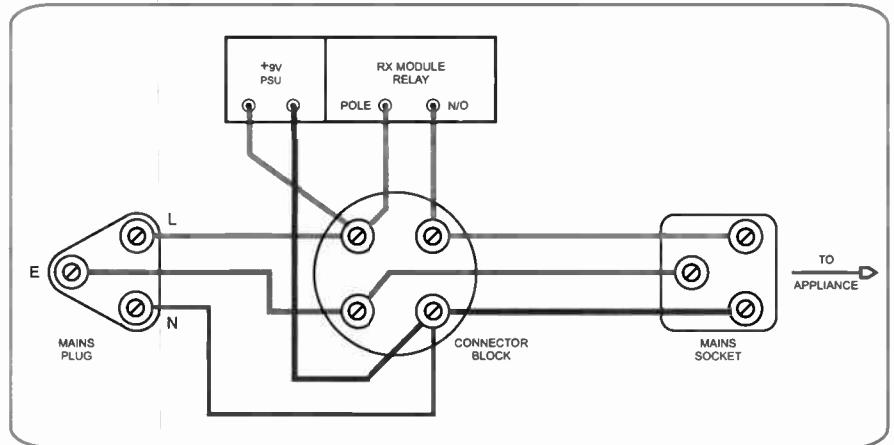
Fig.7. Suggested wiring arrangement linking the receiver unit between the mains supply and the appliance to be controlled
