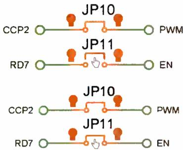
Fig.6. Jumpers are default open as the demo board is generic to all projects, to engage a jumper, simply click on it.
