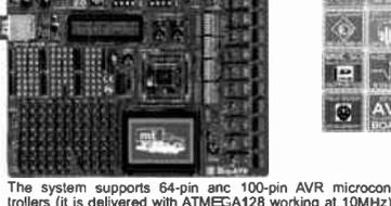
The system supports 64-pin and 100-pin AVR microcontrollers (it is delivered with ATMEGA128 working at 10MHz). Many already made examples guarantee successful use of the system. BIGAVR is easy to use Atmel AVR development system. BIGAVR has many features that makes your development easy. You can choose between USB or External Power supply. BIGAVR also supports Character LCD as well as Graphic LCD.
