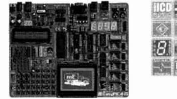
Following tradition of its predecessor EasyPIC3 as one of the best PIC development systems on the market, EasyPIC4 has more new features for the same price. The system supports 8-, 14, 18, 20, 28 and 40 pin PIC microcontrollers (it comes with PIC16F877A). USB 2.0 on-board programmer with mikroCD (In-Circuit Debugger) enables very efficient debugging and faster prototype development. Examples in C, BASIC and Pascal language are provided with the board.
