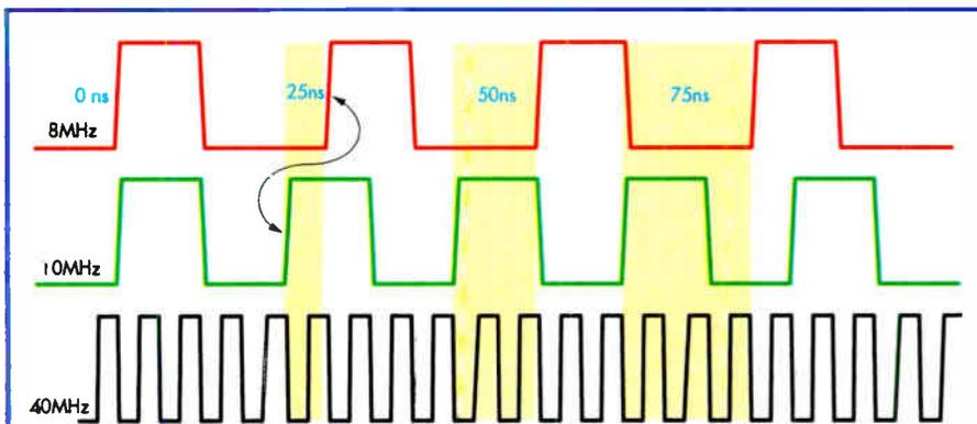
**Fig.8:** the time difference between the rising edges of 8MHz and 10MHz clock signals are exploited to enable high-speed sampling. The micro latches a high on PD1 (pin 3) on the rising edge of its 10MHz clock and after a 0, 25, 50 or 75ns delay, the rising edge of the 8MHz clock freezes the input voltage at that instant.
