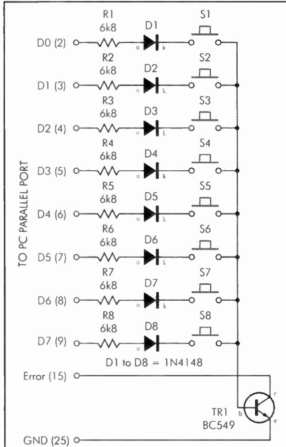
Fig.1. Simple 'active' circuit for monitoring eight switches
