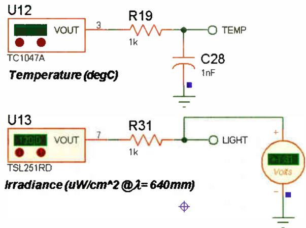
Fig.2. The virtual sensors with additional virtual instrument to compare output voltage with stated value.
