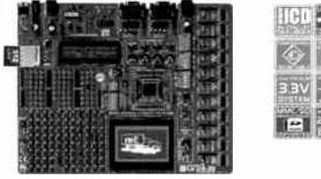
System supports 64, 80 and 100 pins PIC24F/24H/dsPIC33F microcontrollers (it comes with PIC24FJ64GA010 - PIC24 16-bit Microcontroller, 96 KB Flash Memory, 8 KB RAM in 100 Pin Package). Examples in BASIC, PASCAL and C are included with(in) the system. You can choose between USB and External Power supply. LV 24-33 has many features that make your development easy. USB 2.0 on-board programmer with mikroCD (In-Circuit Debugger) enables very efficient debugging and faster prototype development.
