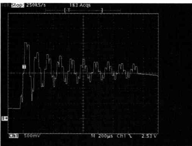
Fig.7c: with a timebase of 200 $\mu$ s/div, the sample-and-hold control signal is now just a succession of spikes and is not shown. At this time scale, the sequence of flat plateaus reproduces a digitised version of the original ringing waveform of Fig.7a, occurring at a rate almost 1000 times faster.
