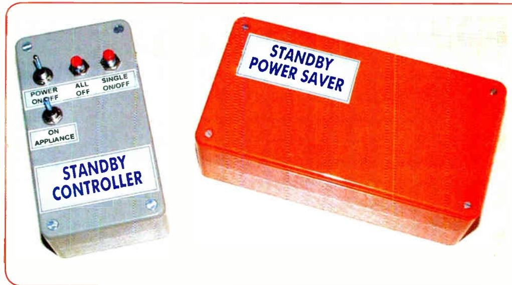
The completed prototype transmitter (left) and receiver (right) modules that make up the Standby Power System. Not shown on the receiver unit are the Main ID and Unit On/Off pushbutton switches (S6 and S7)
