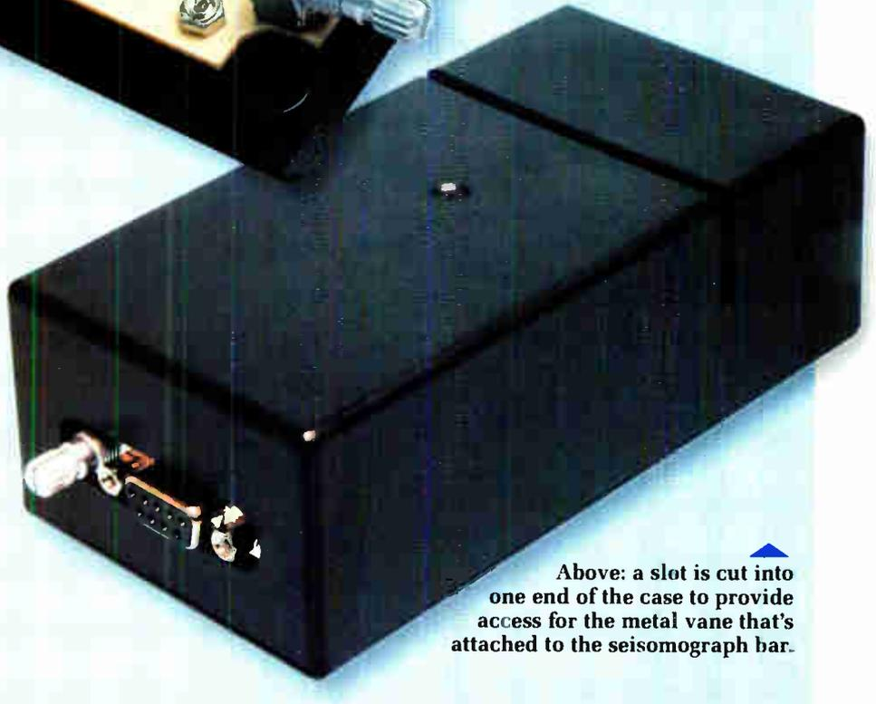
▲ Above: a slot is cut into one end of the case to provide access for the metal vane that's attached to the seismograph bar.
