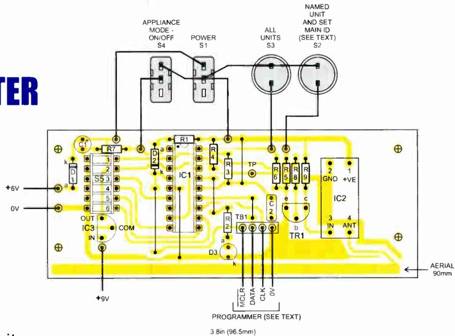
Fig.4: Printed circuit board topside component layout, interwiring details and full-size underside copper foil master for the transmitter unit
