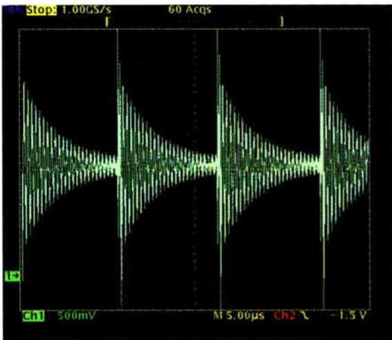
**Fig.3:** this scope shot shows the response of an LCR circuit to an applied pulse. Decaying oscillations give rise to a ringing waveform, which continues until all energy supplied by the pulse is dissipated in the circuit resistance. The frequency of oscillation is the same as would occur at the peak in the spectral response.
