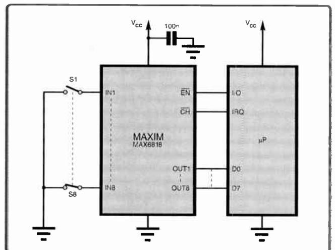
Fig.6. Multiple switch debounce using a MAX6818 (Maxim datasheet)
