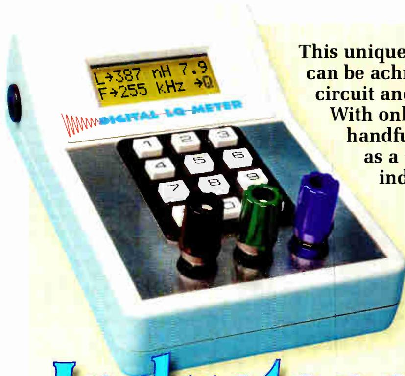
This unique project demonstrates what can be achieved with a relatively simple circuit and some clever programming. With only a microcontroller and a handful of components, it functions as a wide-ranging, multi-frequency inductance and Q-factor meter.
