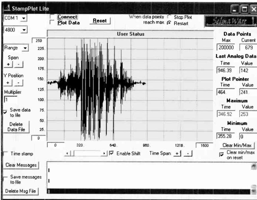
**Fig.3:** this simulated plot of an earthquake was produced during final sensitivity tests of the seismograph. A gentle puff of air aimed towards the seismograph masses from two metres away produced the first 'earthquake' waves, while similar puffs from one metre gave the full scale deflection.
