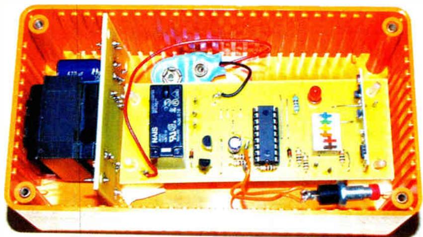
Layout of components, including optional mains power supply, inside a partially completed receiver unit
