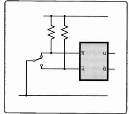
Fig.4. Switch debounce using an RS flip-flop
