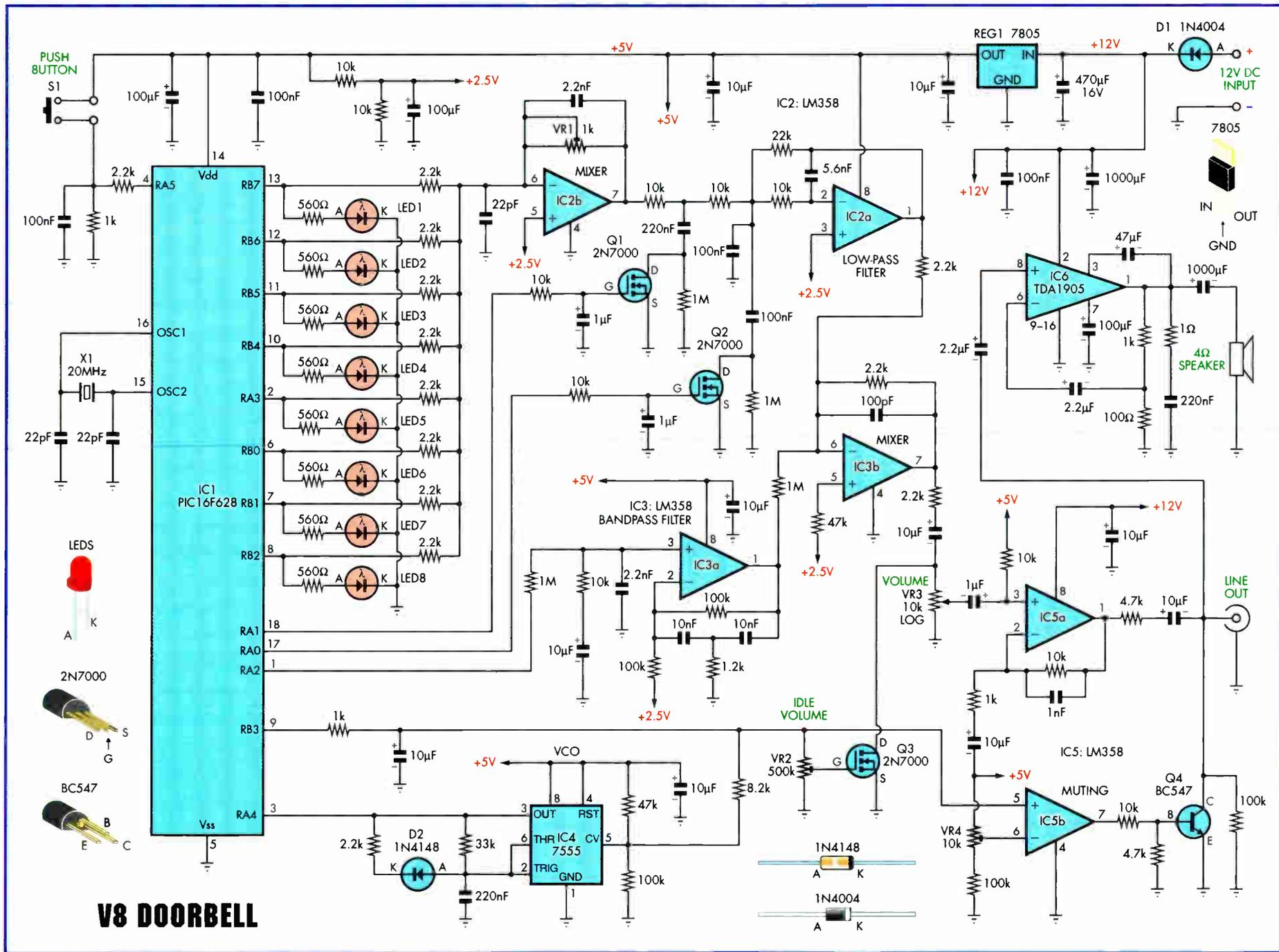
**Fig.2 (left): the complete circuit of the V8 Doorbell. A PIC16F628 microcontroller (IC1) produces the simulated V8 engine signals. These signals are then processed and fed to audio amplifier stage IC6.**
