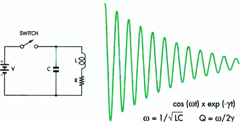
Fig.2: the temporal method used in this design relies on decaying oscillations after a rectangular pulse is applied to the resonant circuit. The Q factor manifests as the ratio of the oscillation coefficient (the angular frequency) to twice the decay coefficient.
