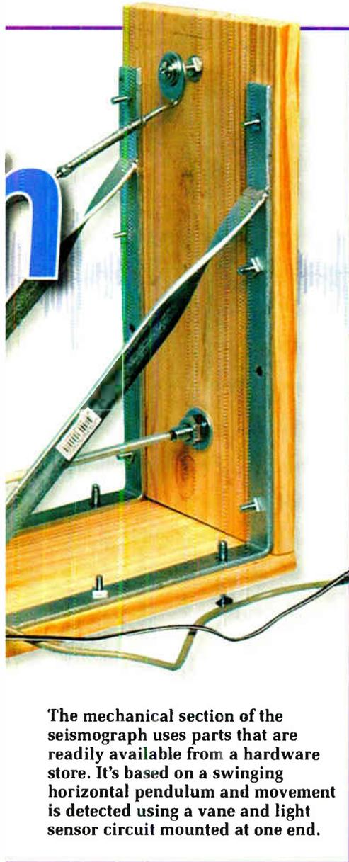
The mechanical section of the seismograph uses parts that are readily available from a hardware store. It's based on a swinging horizontal pendulum and movement is detected using a vane and light sensor circuit mounted at one end.
