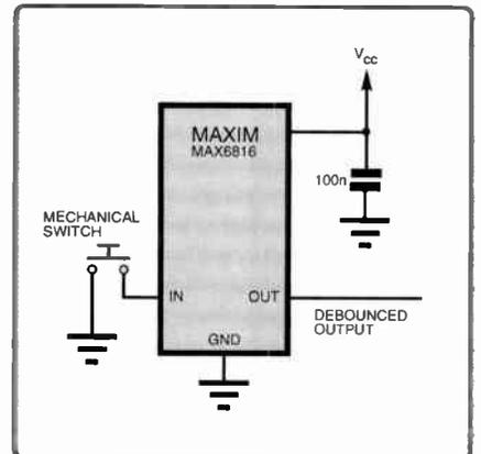
Fig.5. Switch debounce using a MAX 6816 (Maxim datasheet)
