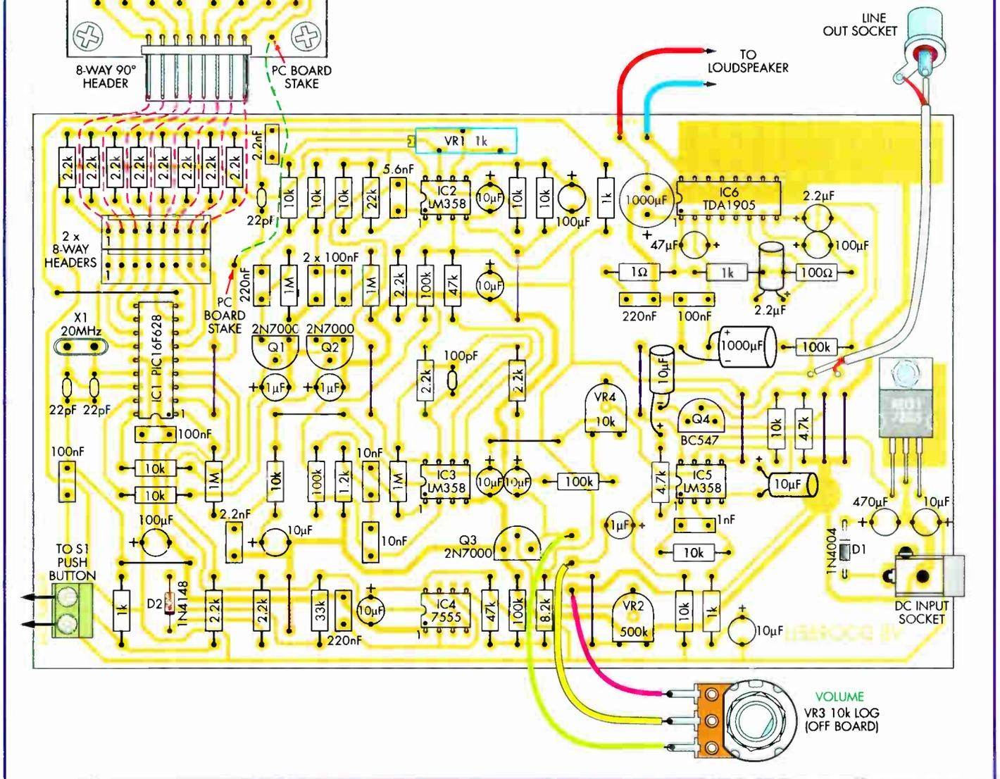
The trimpots and capacitors can go in next. When installing the capacitors, note that the polarised types must be installed with the correct polarity. Note also that three electrolytic capacitors have to be placed on their side, so that there is room for the loudspeaker later on (see layout diagram photos).
