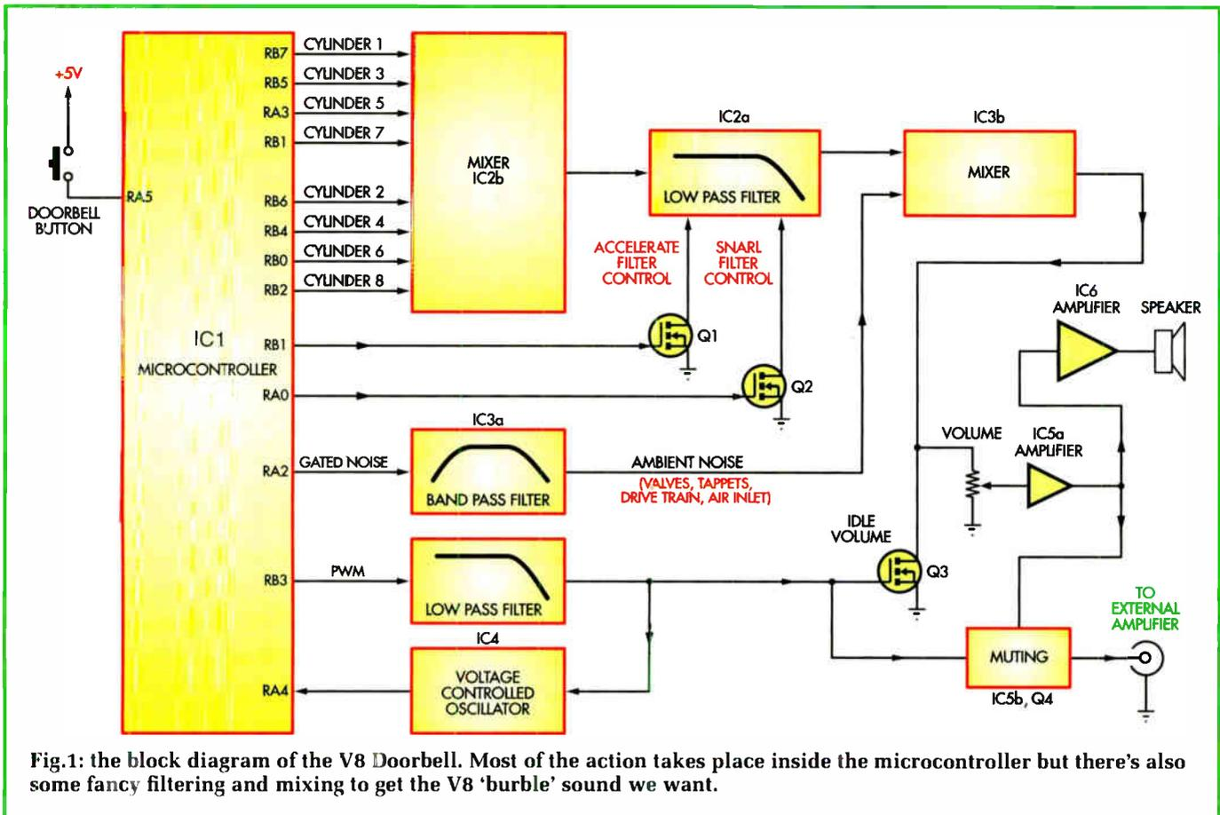
Fig.1: the block diagram of the V8 Doorbell. Most of the action takes place inside the microcontroller but there's also some fancy filtering and mixing to get the V8 'burble' sound we want.
