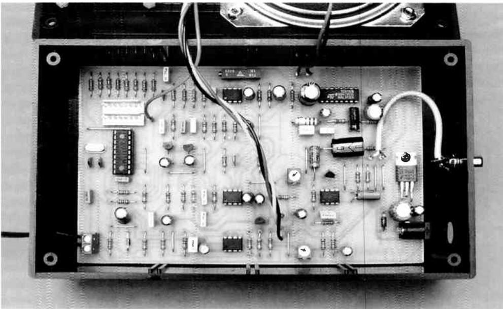
The PC board is secured by clipping it into the integral slots in the side of the case. Power comes from a 12V DC 1A plugpack.
