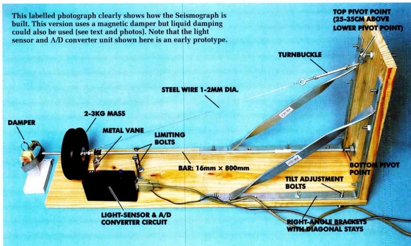
frame shown, the unit could be built into any strong cupboard, bookcase, shelf or even a strong, metal frame. In that case, the brackets and wooden frame would not be needed. Any type of metal rod could be used (as long as it's strong enough) and the same goes for the mass at one end.
