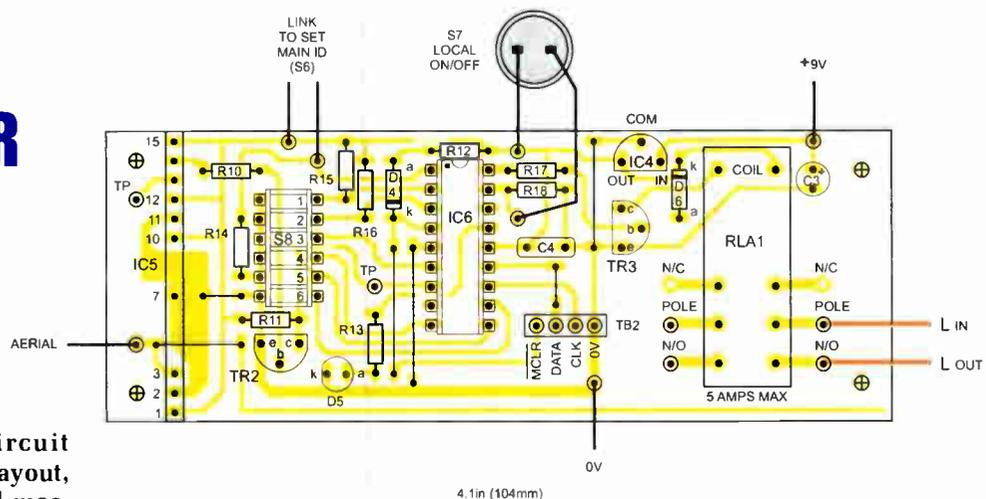
Fig.5: Printed circuit board component layout, full-size copper foil master and wiring details for a single receiver unit. You will, of course, require a receiver for each additional appliance. Note the relay contacts must be rated according to the appliance being controlled
