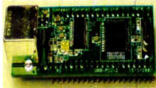
Compatible with Microchip's MPLab 'free of charge' programming environment. Libraries and linker scripts included to support assembler programs (MPLab) and popular compilers.
