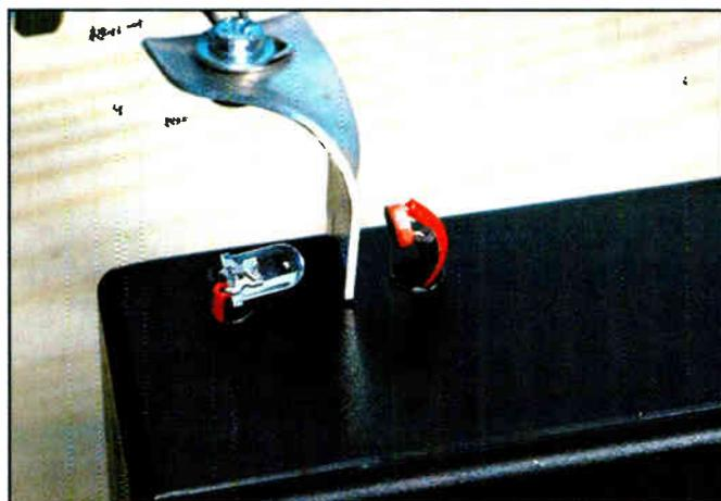
In the prototype, the LED and the LDR were brought out through holes in the case, with the vane sitting between them – see above. By contrast, in the final version, the LED and LDR are inside the case and the vane rides in a slot. The vane is positioned so that it normally 'shadows' about half the LED body.
