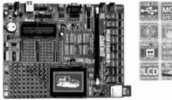
The system supports PIC, AVR, 8051, ARM and PSoC microcontrollers with a large number of peripherals. In order to continue working with different chip in the same development environment, you just need to switch a card. UNI-DS3 has many features that make your development easy. You can choose between USB or External Power supply. Each MCU card has its own USB 2.0 programmer!
