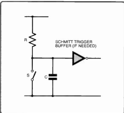
Fig.2. Using a capacitor to debounce a switch
