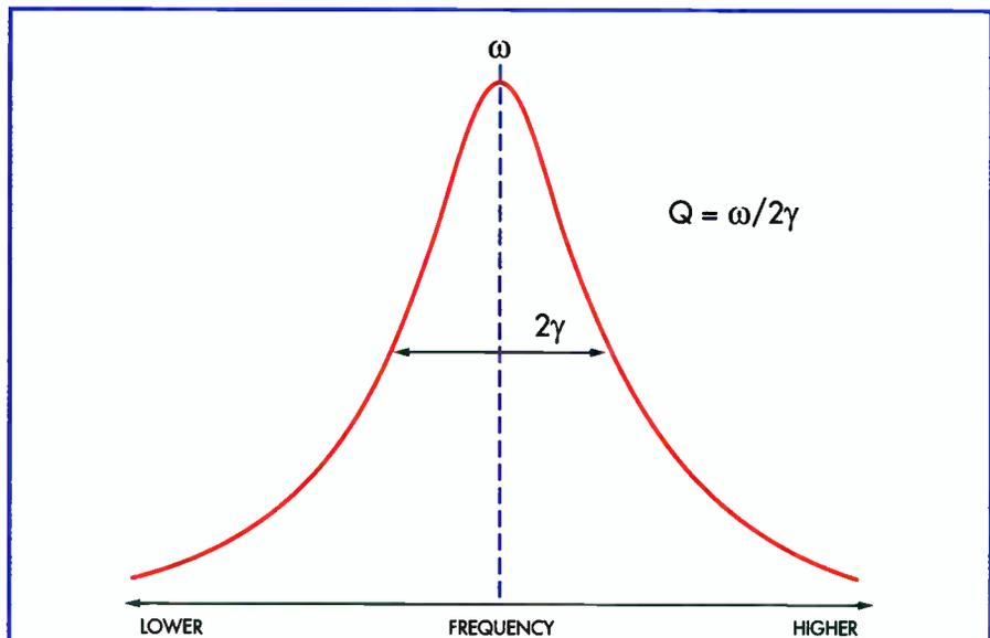
Fig.1: the spectral response of a resonant circuit reveals a peak at a given frequency, dropping away on both sides in a bell-shaped curve. The Q factor is manifest as the ratio of the peak frequency to the width of the bell-shaped curve at half-power.
