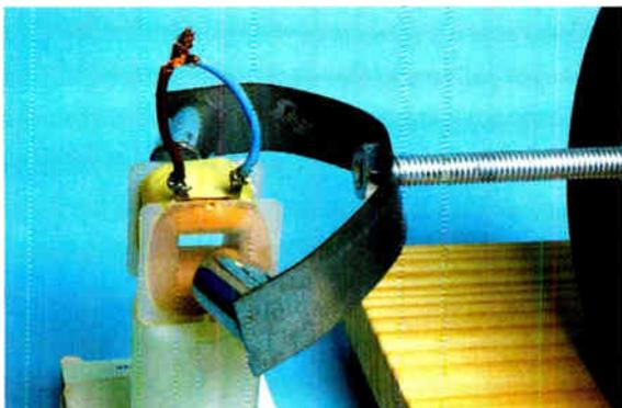
Above and right: these two views show the alternative damping methods for the swinging bar. Magnetic damping (above) uses a couple of super magnets and a coil of wire, while liquid damping (right) uses a 40 x 50mm plastic paddle dipped into a rectangular container of water.
