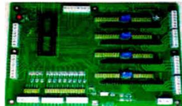
All options are configured using jumpers, and stepper motor drive current can be easily adjusted for each module by variable resistors. All connections are made by high quality screw terminals. The board has been designed to accommodate other driver modules as they become available.
