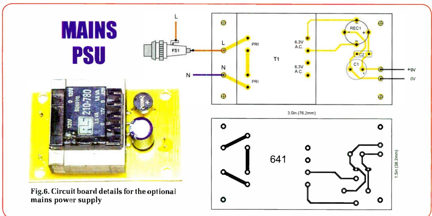
Fig.6. Circuit board details for the optional mains power supply
