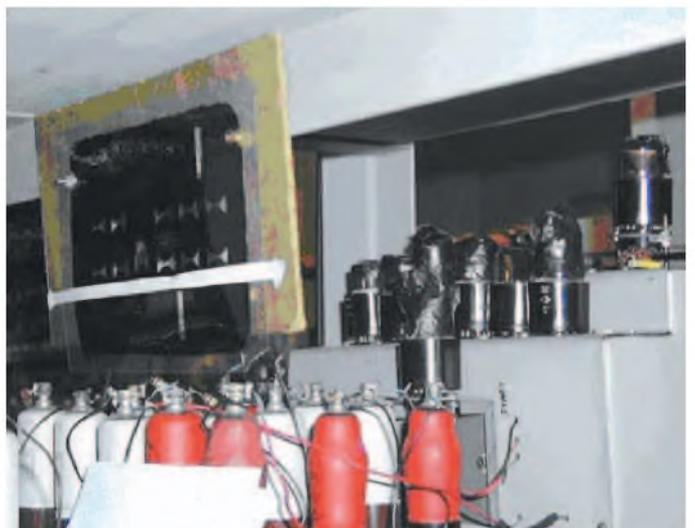
In the photograph of the *Colossus* rebuild, the tape reader can be seen on the right. A bright light is shone through the tape and focused onto hard vacuum photocells, one for each bit of data and one for the clock pulse. The photocells used in the rebuild are original *Colossus* parts.
