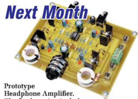
**Prototype Headphone Amplifier.** The final version includes a second headphone socket and has a few other minor changes
