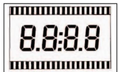
Fig.4. Four-digit static LCD Panel
