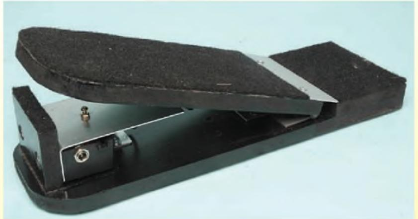
The footswitch is made using the MDF panelling as shown below. We painted the assembly with black paint and covered the foot areas with speaker carpet.
