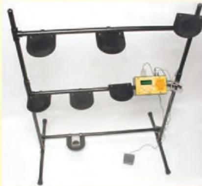
The wires for the sensors can be made tidy along the frame using cable clips.
