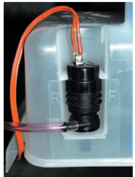
A simple pump/reservoir combination for an intercooler water spray can be cheaply obtained by using a windscreen washer reservoir and pump.
