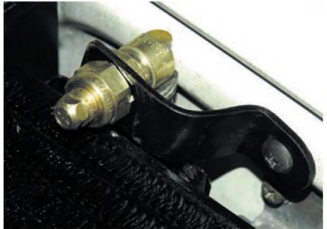
This Spraying Systems nozzle incorporates a filter. The nozzle gives far better results than the small garden irrigation nozzles that are widely used in intercooler spray applications.
