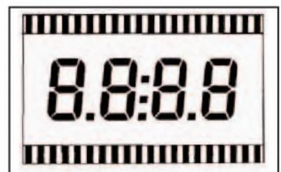
Fig.4. Four-digit static LCD Panel
