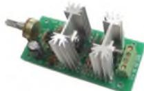
Controls the speed of most common DC motors (rated up to 32Vdc/10A) in both the forward and reverse direction. The
