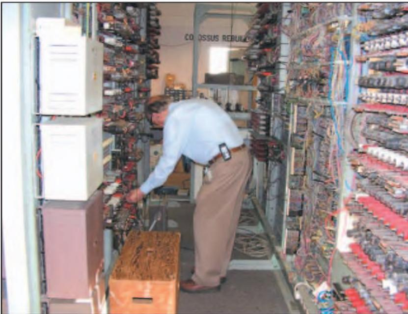
A total of ten *Colossi* were built, the design being improved and upgraded throughout the war. These machines were used to decode tens of thousands of intercepted messages and made a huge contribution to the Allied victory.
