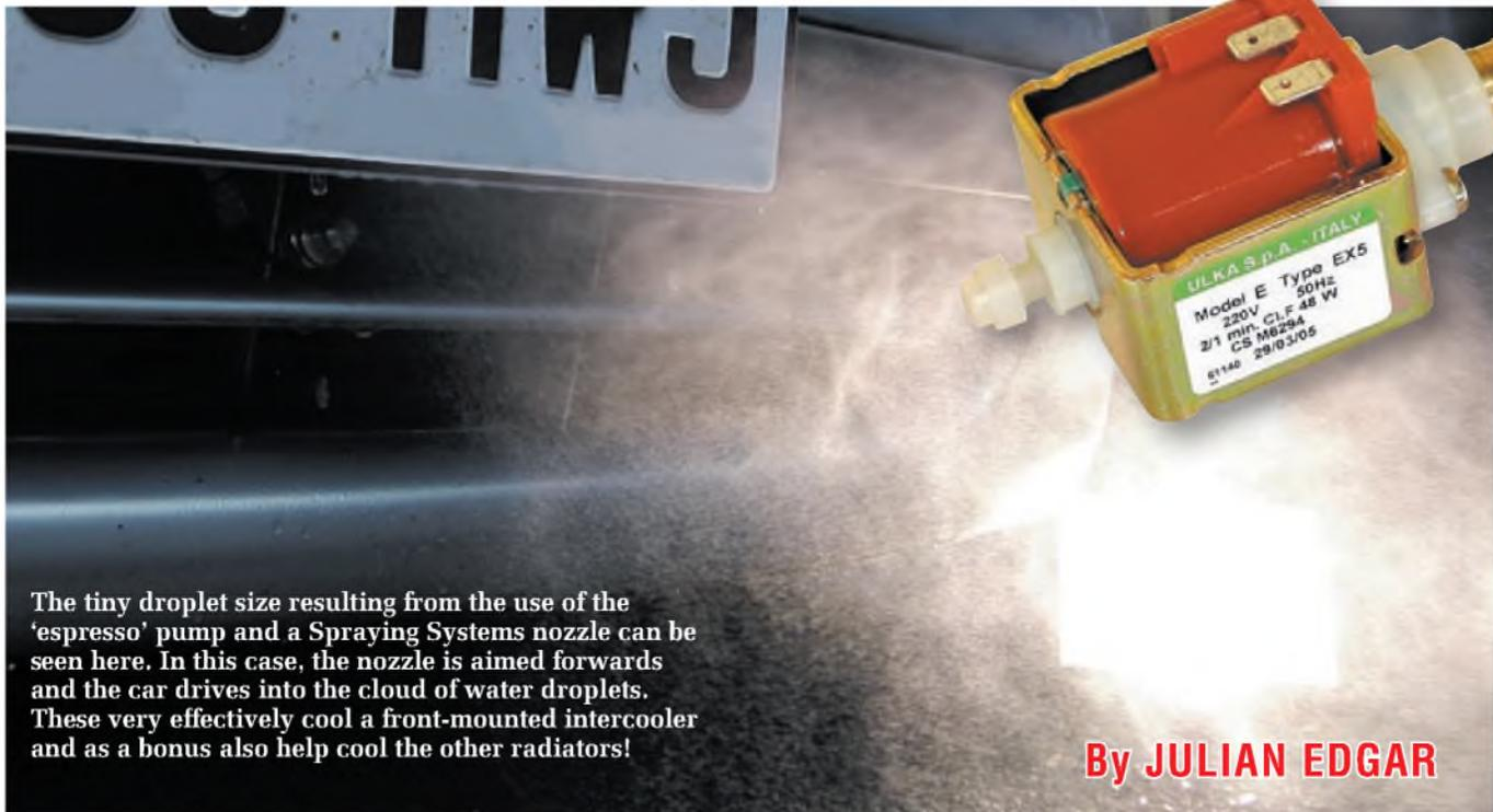
The tiny droplet size resulting from the use of the 'espresso' pump and a Spraying Systems nozzle can be seen here. In this case, the nozzle is aimed forwards and the car drives into the cloud of water droplets. These very effectively cool a front-mounted intercooler and as a bonus also help cool the other radiators!
