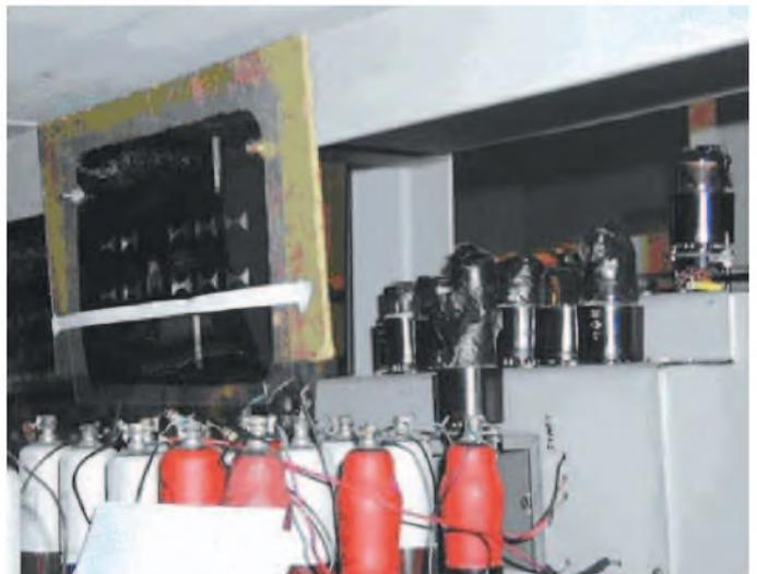
In the photograph of the *Colossus* rebuild, the tape reader can be seen on the right. A bright light is shone through the tape and focused onto hard vacuum photocells, one for each bit of data and one for the clock pulse. The photocells used in the rebuild are original *Colossus* parts.
