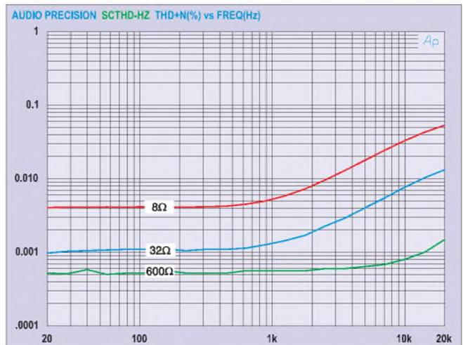
**Fig.7: amplifier total harmonic distortion (THD) and noise versus frequency, measured with an output power level of 100mW. As is clear from these curves, the amplifier performs much better when driving 32Ω and higher impedance headphones. Most headphones will reach full output well below 100mW, so you can expect even better performance than these already excellent curves reveal!**
