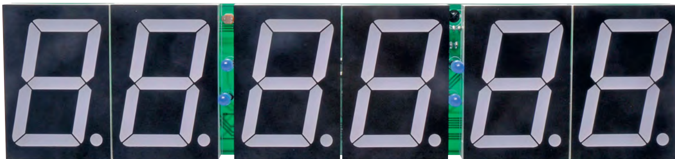
Above: the 7-segment LED displays plug into sets of 5-way SIL sockets, as shown on Fig.2. Make sure that the displays are all correctly oriented (ie, decimal points at bottom right).
