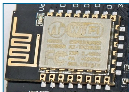
Fig.12.1. ESP8266 serially-controlled Wi-Fi gateway
