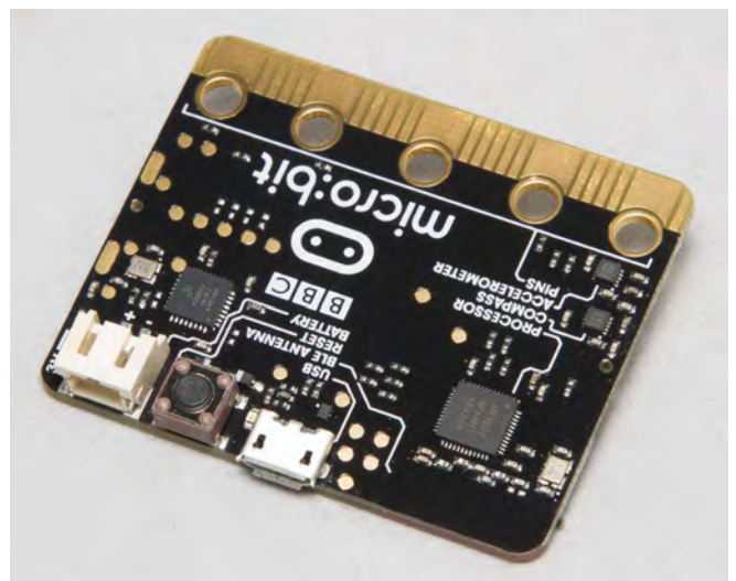
Fig.5. The reverse side of the board, showing the power connector, reset switch and Micro USB port. Opposite these is the edge connector that provides a useful GPIO port – note that some of its input/output lines are shared with hardware on the board.
