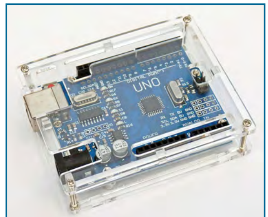
Fig.12.20. Typical low-cost enclosure for an Arduino Uno
