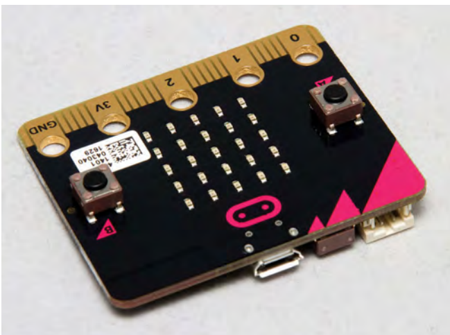
Fig.4. The front side of the BBC Micro Bit board showing the two input buttons and the LED array. It also has a built-in accelerometer and a magnetic sensor
