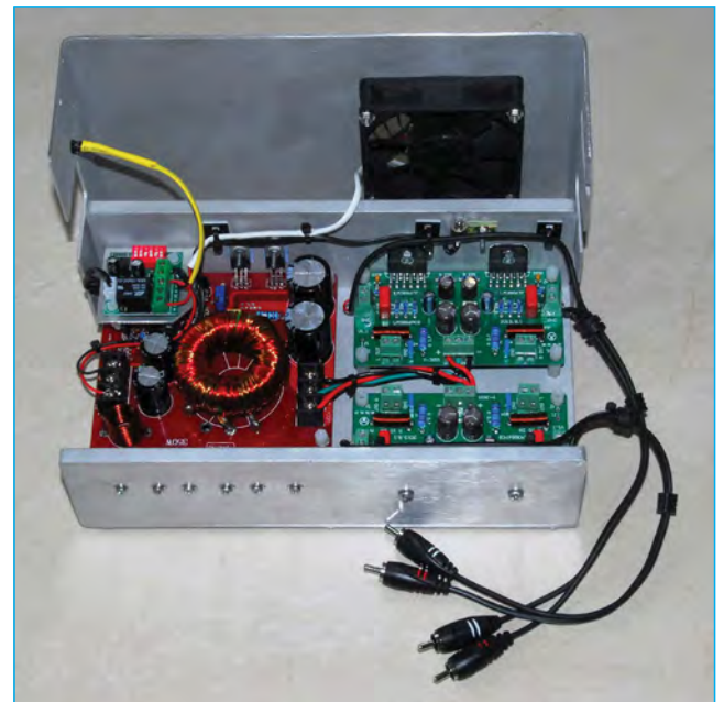
The completed four-channel, 12V amplifier – the power supply module is on the left, and the two 2-channel amplifier modules on the right. When the lid is placed on top, it locates the fan above the amplifier modules. (A similar-sized vent hole to the fan is located under the power supply module.)
