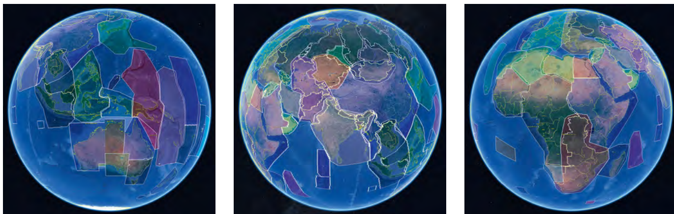
Fig.10(a-d): this series of images shows the complete global land mass coverage of the time zone data programmed into the clock. There are 128 separate shaded areas, mapped to 73 different time zones, each with different UTC/GMT offsets and daylight savings rules. Note that many zones overlap, which has been done to reduce the compressed size of the data set; see text for more details.
