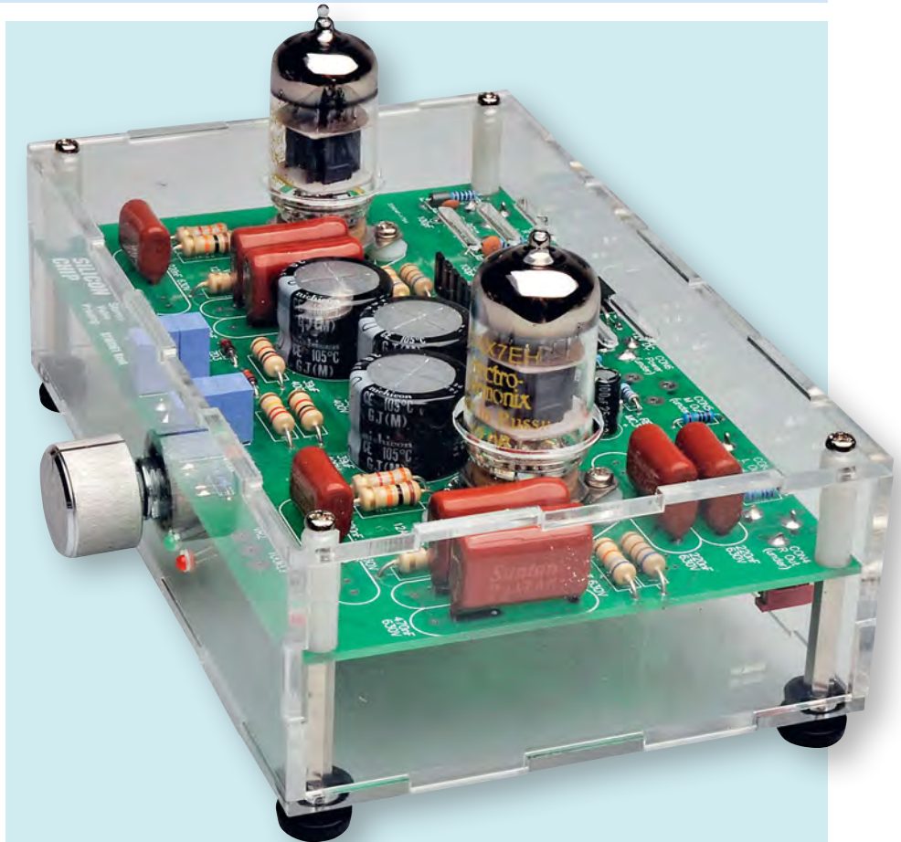
The case is assembled by first fastening the top and bottom panels and the PCB together (see also Fig.10). The rear panel is then glued to the base, after which the base is removed and the remaining panels fitted as detailed in the text. DO NOT glue the front panel or any of the other panels to the top cover.
