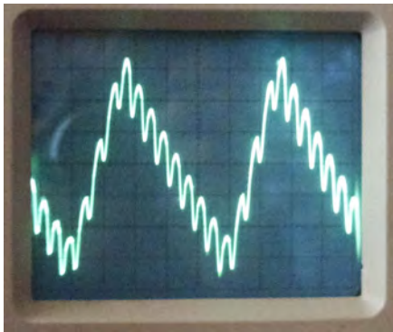
Fig.23. Oscilloscope showing how audio superimposes itself onto the ripple waveform on the power supply.
