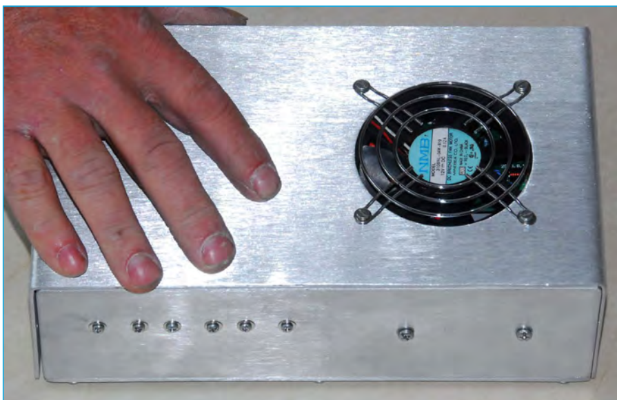
One of the requirements was that the amplifier be reasonably compact and light. The final item has a mass of 1.75kg and dimensions of 250 x 140 x 75mm.
