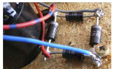
Fig.28. If you use a schottky bridge rectifier it will have to be made from individual diodes.
