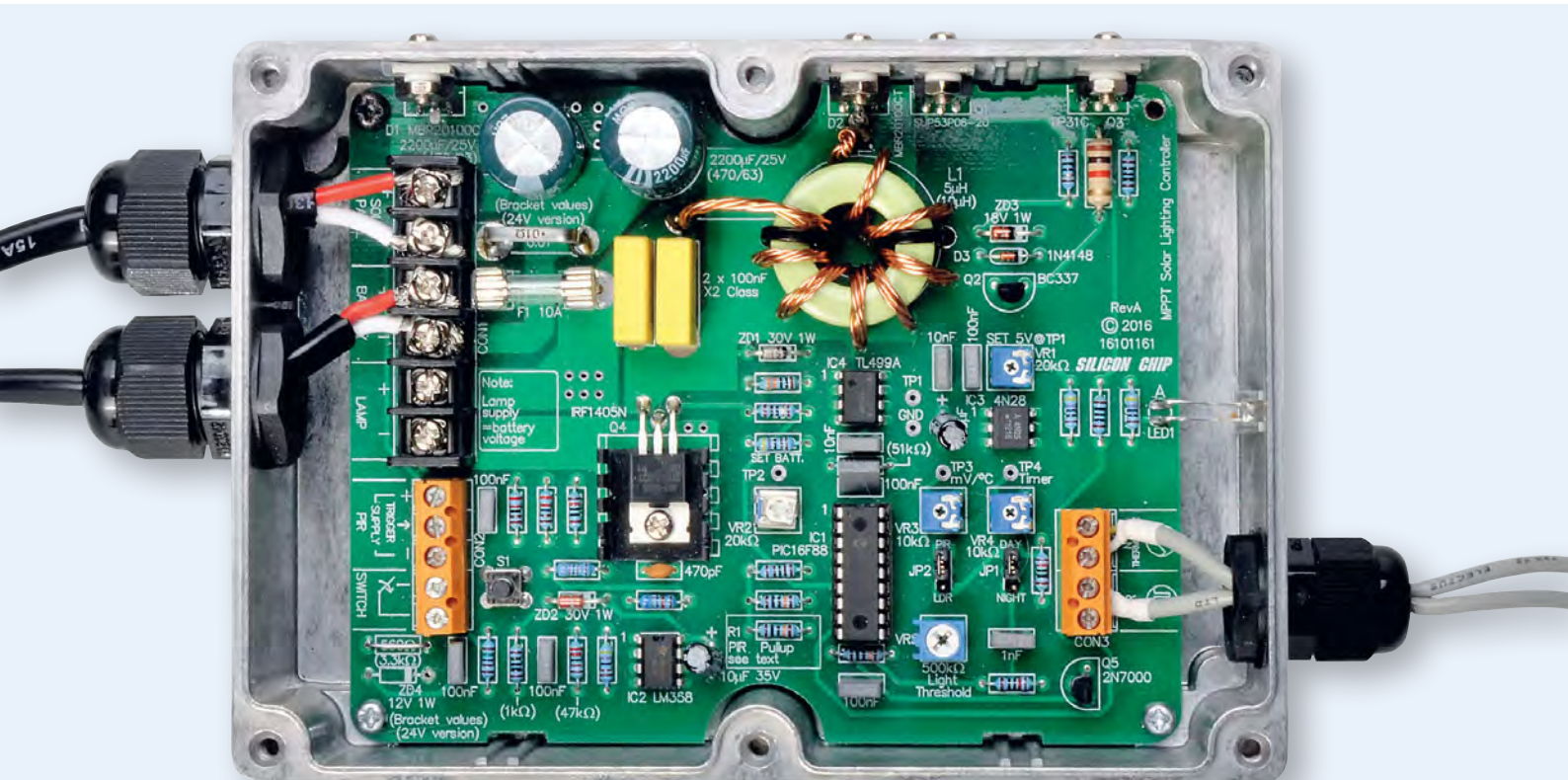
Building the Solar Charger and Lighting Controller is easy, with all parts mounted on a single PCB. This is housed in a diecast metal case which provides the necessary heatsinking. The full assembly details are in Part 2 next month.
