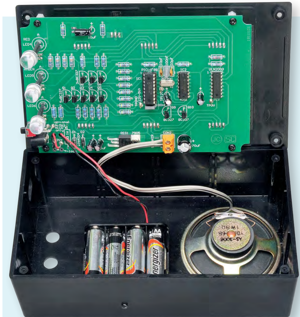
The view inside the completed prototype. The battery holder is secured to the top of the case using a No.4 × 9mm self-tapping screw that goes into a slot at one end of the holder's plastic moulding.
