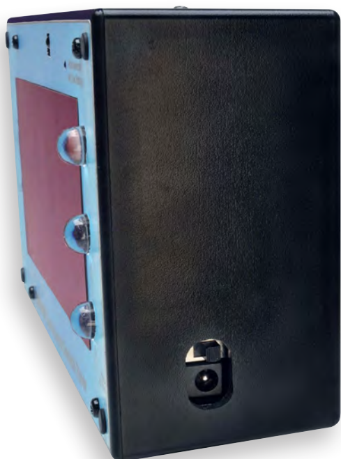
A hole is cut in the righthand end of the case to provide access to the DC socket and on/off switch.
