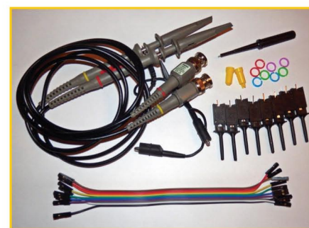
Fig.1. SmartScope is supplied with a comprehensive set of accessories including two switchable \times 1 and \times 10 probes, a digital cable and grabbers.
