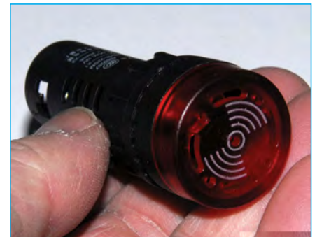
This warning device uses dual LEDs and a beeper to alert the operator. It nominally operates off 12V and will set you back only £4 for five of them.
