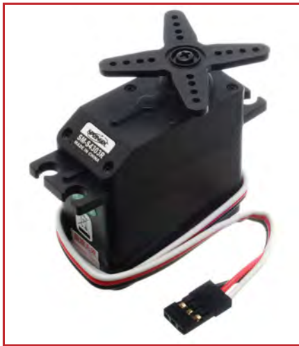
Fig.3. Five of Micromite's I/O pins can generate PWM to drive servos
