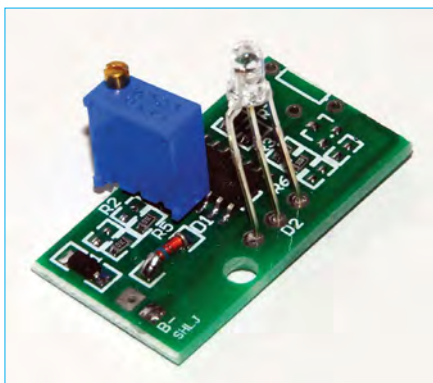
This tiny module uses a red/green LED to show battery voltage, and is good over the range of 6.5 – 20V.
