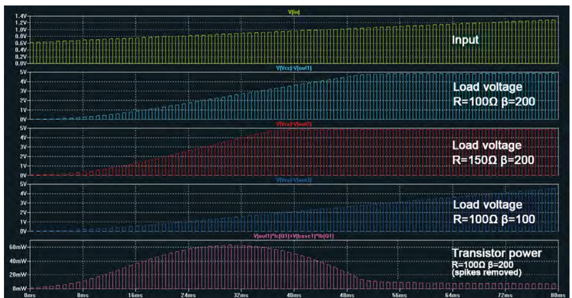
Fig.7. Simulation results for the circuit in Fig.5 with reduced input voltage range and showing the effect of varying load and transistor gain
