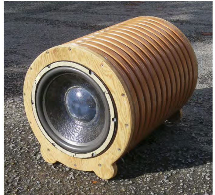
You don't have to be a carpenter or cabinet maker – Julian Edgar encourages innovative cabinet construction techniques. For example, drainpipes can be used to make good sub-woofers.
