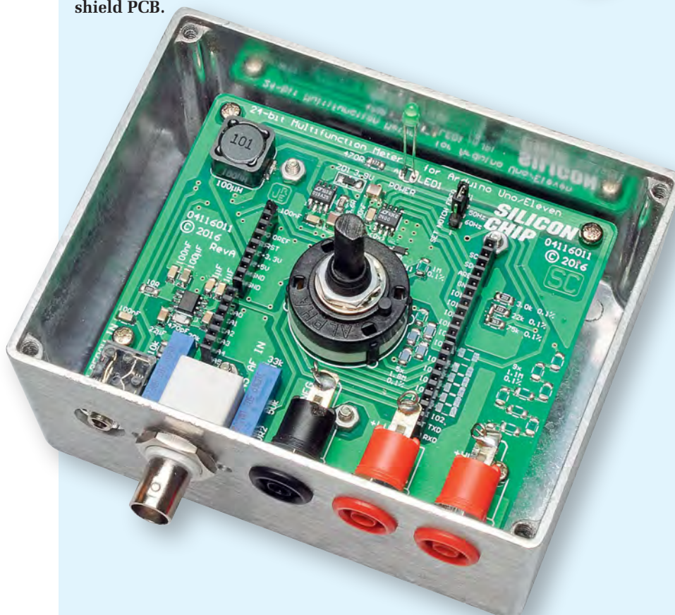
The PCB assembly is installed in the case by first angling the BNC socket down through its hole, then forcing the rear of the assembly down into the case. The three banana sockets are then fitted and wired to the shield PCB.
