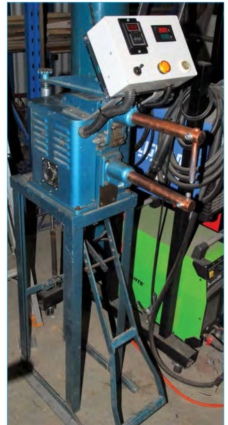
Fig.2. The finished welder with the new control panel, positioned above the welding electrodes. The panel incorporates a digital timer, digital mains voltage and current meters, a 'welding occurring' pilot light, and a manual weld over-ride switch.
