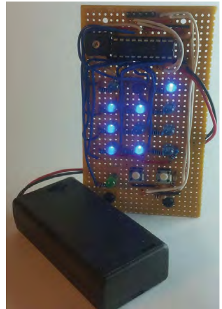
Fig.5. Blue LED Binary Clock
