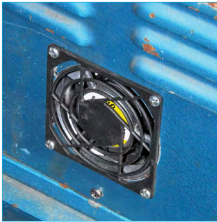
Fig.3. A fan was added to circulate air around the transformer. It's funny to think that when the welder was produced over 50 years ago, cooling fans such as these were unknown!
