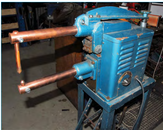
Fig.1. This old spot welder has a high current capability and is built like a tank. However, as purchased, the welding duration was controlled by a mechanical switch operated by a foot pedal. This made setting the welding duration a bit hit and miss.
