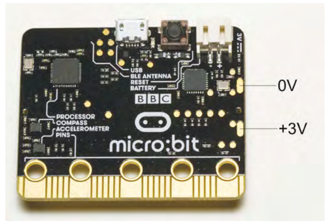
Fig.6. The reverse side of the micro:bit, showing the two power connector pads. Using these pads looks as though it might be a little risky, and due care would have to be exercised.
