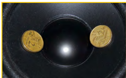
Fig.4. Small weights are added to the cone (here coins have been used). Software to calculate speaker compliance uses the resultant change in resonant frequency of the driver.
