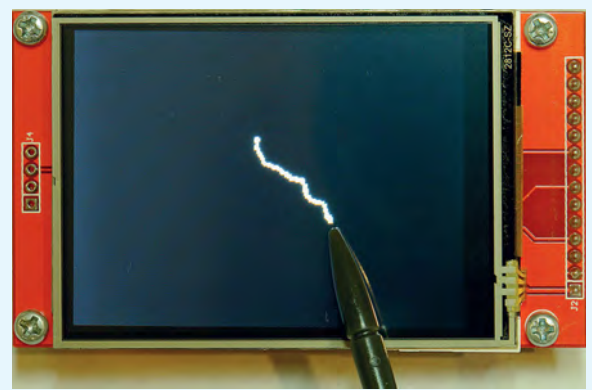
Example of the display when the command GUI TEST TOUCH is used. It illuminates pixels where touched and is a good test for the touch calibration.
