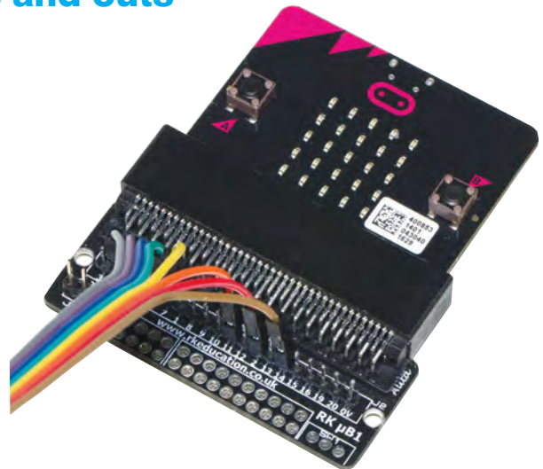
Fig.2. An adaptor is needed to provide proper access to the edge connector so that it can be connected to a solderless breadboard, or other prototyping system
