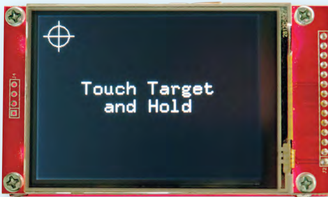
This is an example of the display when calibrating the touch screen using the command GUI CALIBRATE.
