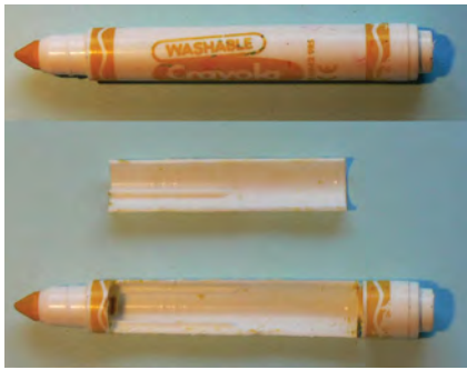
Fig. 5. From magic marker to probe case
