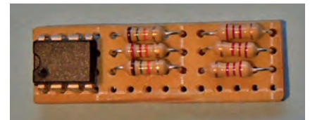
Fig. 11. LM393 circuit on a small piece of board
