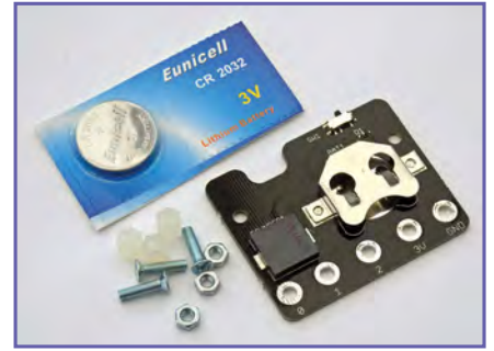
Fig.1.6. The MI:power board designed for attaching to the rear of a micro:bit
