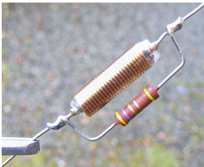
Fig.12. An LC network should be inserted at the output pin if driving high capacitance loads, such as fancy plaited speaker cable.
