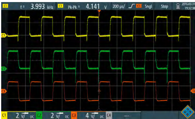
Fig.2: the yellow and green traces show the complementary drive signals applied to the piezo transducer. The two signals are at 3.99kHz and have an amplitude that's close to 3V peak-to-peak, not allowing for the overshoot spikes. The total signal applied to the transducer is shown in the red trace and is 6V peak-to-peak
