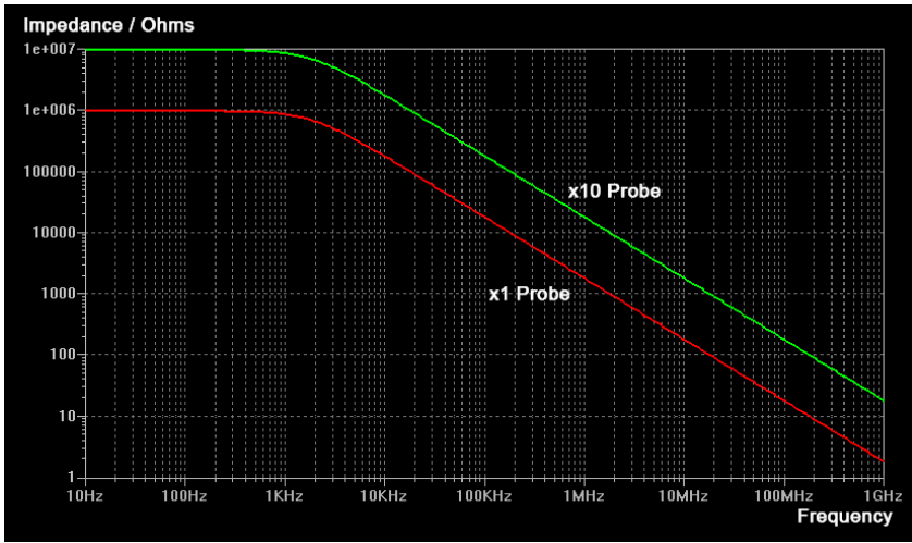
Fig.5. Variation of impedance of probe plus oscilloscope for x1 and x10 passive probes
