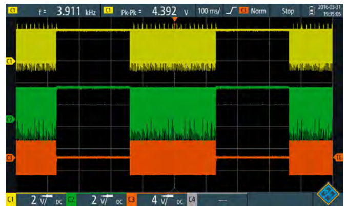
Fig.3: this scope grab shows the same complementary drive signals but at a much slower sweep speed of 100ms/div. The signal bursts are about 280ms long and are separated by gaps of approximately 220ms. The red trace shows the total signal applied to the transducer and is 6V peak-to-peak.
