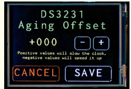
Screen 6: an ageing offset of +1 will slow the clock by about 0.1ppm while -1 will speed it up by the same amount. You can enter -127 to +127.
