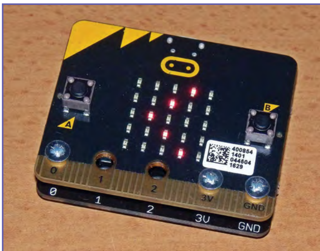
Fig.2.15. The micro:bit electronic spirit level in use
