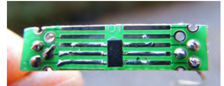
Fig.4. SMT dual-JFET mounted on board; it costs 30-times less than a metal-can version.
