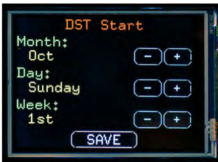
Screen 5: setting daylight saving rules is simple. The clock always increments or decrements the time by one hour at 2am (non-daylight saving time) on the start or ending day specified. The only exception is the UK (time zone zero), where the time switch occurs at 1am.
