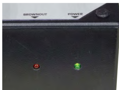
The two LEDs are mounted at right-angles to the PCB so they just poke through appropriate holes drilled in the side of the case. For a detailed case drilling diagram, go to the EPE website.
