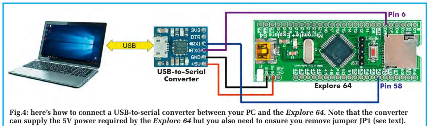
Fig.4: here's how to connect a USB-to-serial converter between your PC and the *Explore 64*. Note that the converter can supply the 5V power required by the *Explore 64* but you also need to ensure you remove jumper JP1 (see text).
