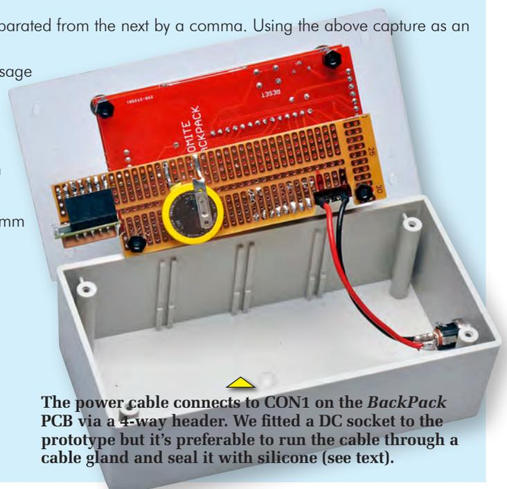
The power cable connects to CON1 on the *BackPack* PCB via a 4-way header. We fitted a DC socket to the prototype but it's preferable to run the cable through a cable gland and seal it with silicone (see text).
