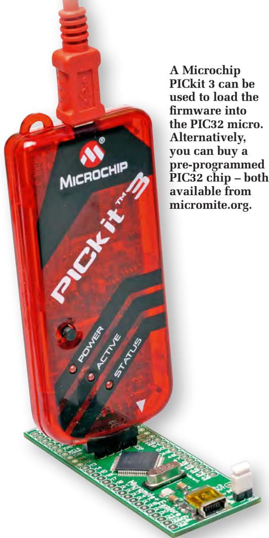
A Microchip PICkit 3 can be used to load the firmware into the PIC32 micro. Alternatively, you can buy a pre-programmed PIC32 chip – both available from [micromite.org](http://micromite.org).
