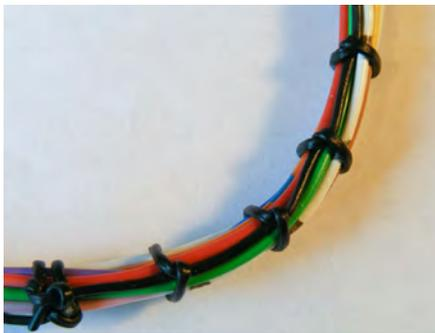
Fig.8. Corners should be laced after forming, with the loops closer together at around 1cm apart.
