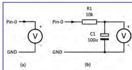
Fig.3.3. Using a voltmeter to read the mean output voltage
