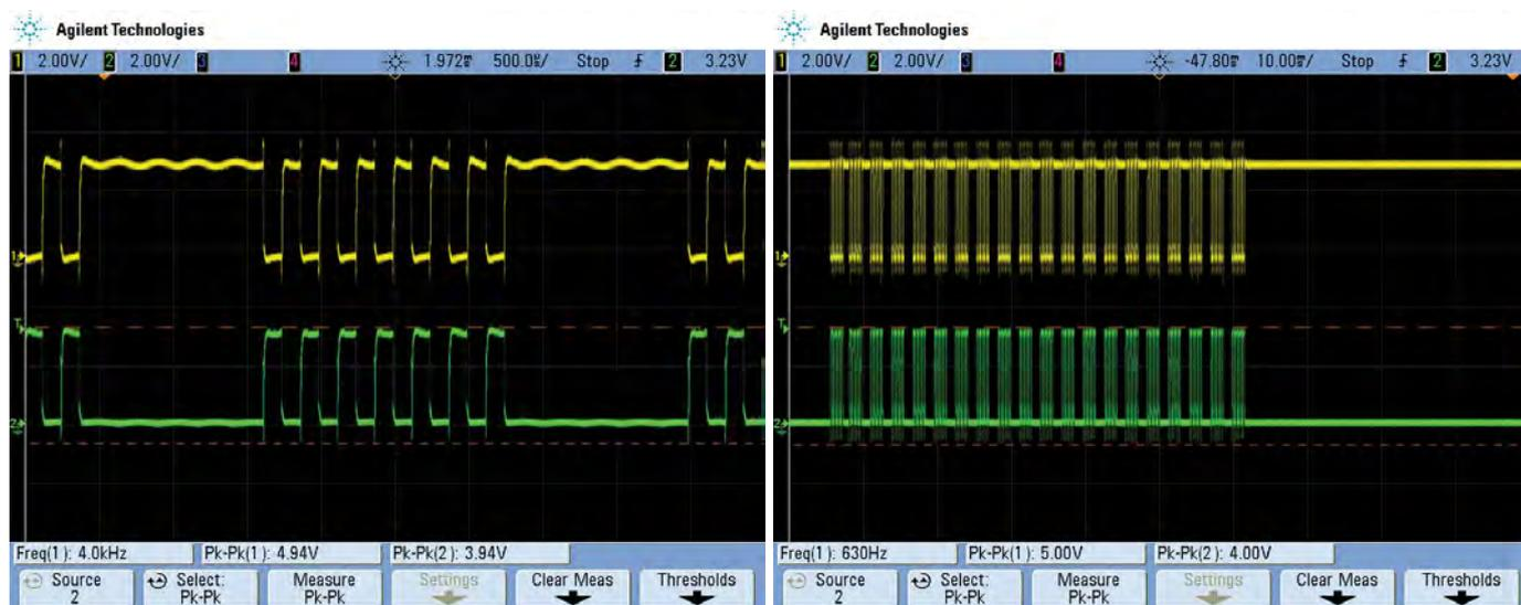
Scope1: This oscilloscope screen shows the drive signals to the piezo transducer, measured at pins 2 and 5 of the PIC microcontroller. The drive frequency is 4kHz. In effect, the total voltage across the transducer is the difference between the two out-of-phase signals, resulting in twice the voltage from pin 2 or pin 5.
