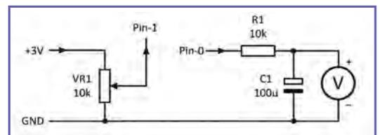
Fig.3.7. Arrangement for testing Listing 3.3
