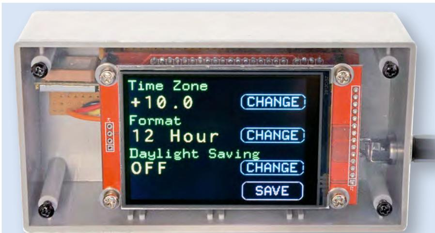
This photo shows the display after the SET button has been pressed for the Clock entry. It allows the time zone to be set, as well as the format for displaying the time (12 or 24-hour). It also allows you to select for daylight saving, in which case one hour is added to the displayed time.
