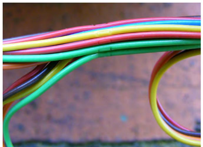
Fig.6. Cable ties can pinch the cable form.
