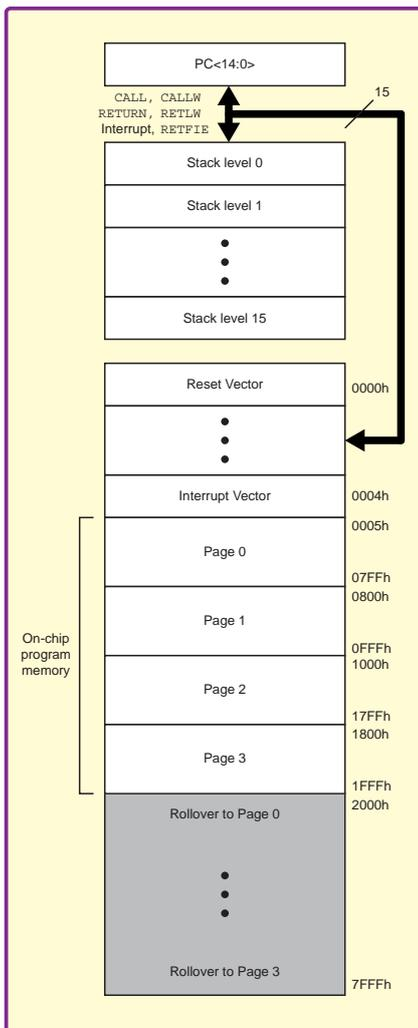
Fig.2. Program memory map and stack for PIC16F1829
