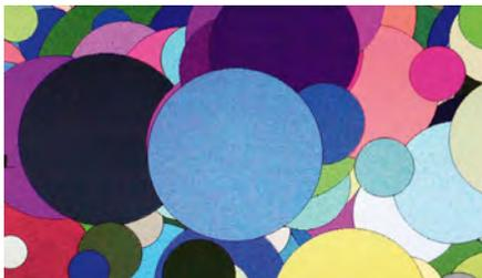
Fig.6: this is the display that you will see on the LCD when the command **GUI TEST LCDPANEL** is used. The display is animated with the circles being rapidly drawn on top of each other.
