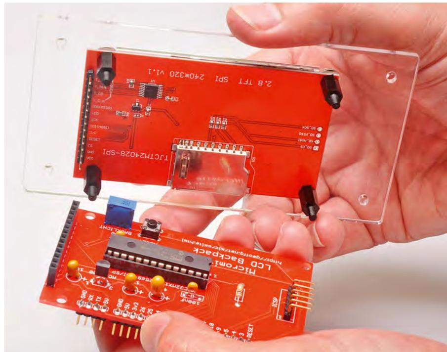
The colour LCD is mounted on the clear acrylic lid before being plugged into the *BackPack* PCB. Be sure to fit the LCD to the lid with the correct orientation.
