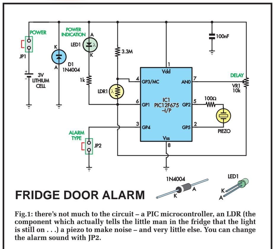
way round. If the polarity is wrong, diode D1 will shunt the reverse current. If the cell holder is installed correctly, then because of the way the CR2032 cell is made, there is no way that it can be inserted back to front. (At least that is true for the particular cell holder we used).
