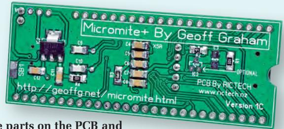
Compare these photos with the layout diagrams when installing the parts on the PCB and check that all polarised parts are correctly orientated. CON1-CON3, IC2 and S1 can be left off if they are not required but most constructors will want to fit them.
