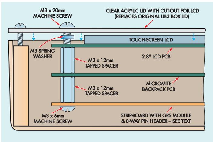
Fig.3: here's how to attach the LCD and Micromite Backpack PCB to the clear acrylic lid. The LCD goes through a cut-out in the lid and sits flush with its top surface.
