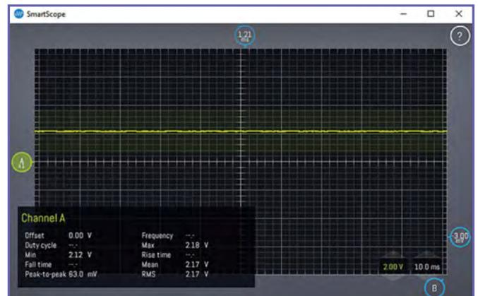
Fig.3.6. Effect of the RC low-pass filter in Fig.3.3(b)
