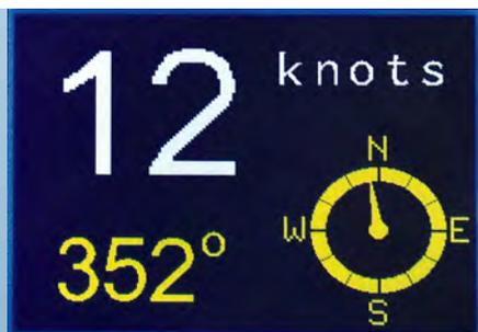
Fig.1: this is the main display shown on the *Boat Computer* when it first powers up. The top half of the screen shows the speed in knots, while the bottom half shows the current heading. The data in both halves can be configured by touching either the top or bottom half of the screen.
