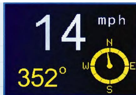
Fig.3: touching the top of the screen again displays the speed in mph. Another touch brings it back to knots.
