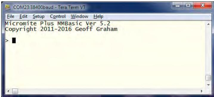
Fig.5: this is what you should see in your terminal emulator when you press the reset button on the Explore 64. If you don't see this, the probable reason is that the USB-serial converter is not connected correctly.
