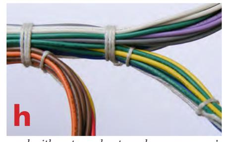
Fig.7. Sequence for basic lacing: a) Start off the cord with a strong knot, such as a surgeon's or square knot; b) Put the cord under the harness; c) Put cord through to form loop; d) The formed twist; e) Tighten the twist; f) Fully tightened twist; g) Straighten things out so it looks good and carry on; h) Branches should be separately tied off.
