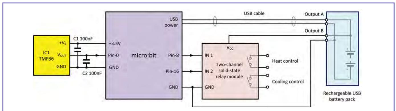
Fig.3.8. Circuit of the micro:bit thermostatic controller
