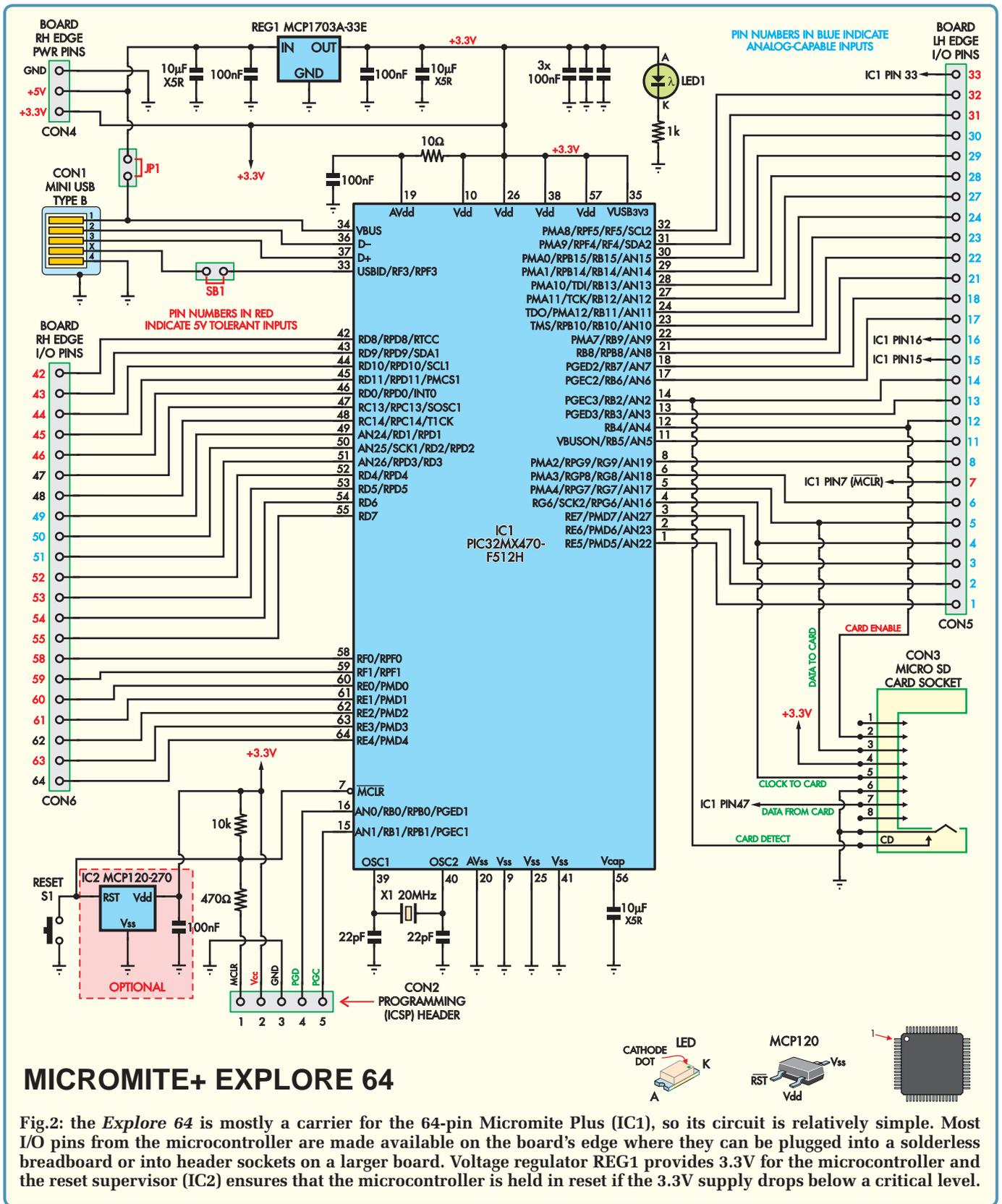
Fig.2: the *Explore 64* is mostly a carrier for the 64-pin Micromite Plus (IC1), so its circuit is relatively simple. Most I/O pins from the microcontroller are made available on the board's edge where they can be plugged into a solderless breadboard or into header sockets on a larger board. Voltage regulator REG1 provides 3.3V for the microcontroller and the reset supervisor (IC2) ensures that the microcontroller is held in reset if the 3.3V supply drops below a critical level.
