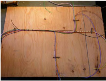
Fig.4. A harness board can be assembled to produce a batch of looms.
