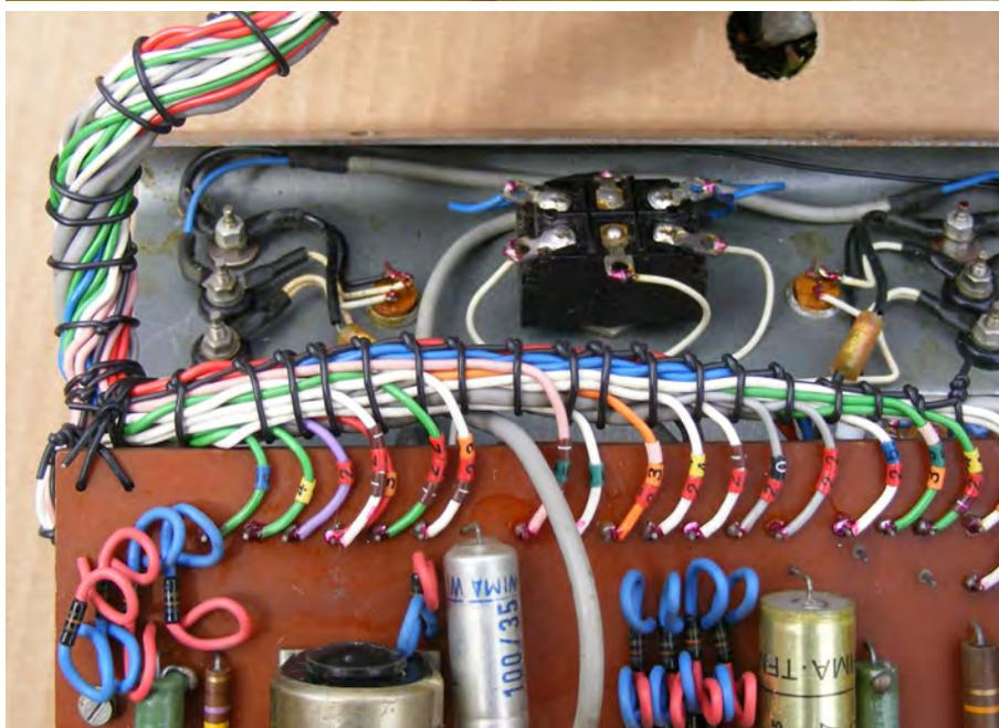
Fig.11. Individual wires can be numbered with push-on sleeves. a) (top) Avionics board, almost a work of art; b) (bottom) Thick harness in an Elliott transistor curve tracer going to multiple pins (Over 50 years old and still intact).
