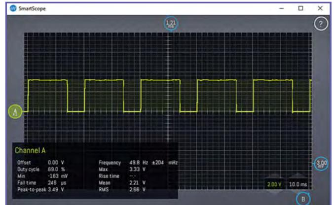
Fig.3.5. PWM output with 70% duty cycle
