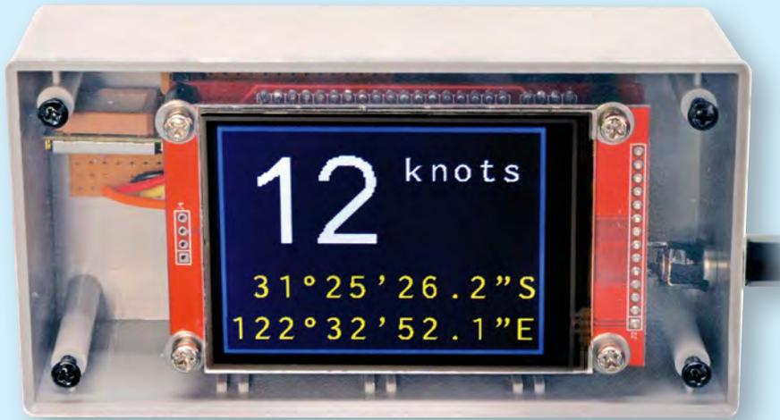
This view shows the unit with the latitude and longitude option selected for the lower half of the display. Changing the displayed data is easy.
