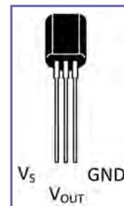
Fig.3.11. Pin connections for the TMP36 temperature sensor
