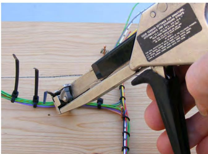
Fig.5 Tie-guns greatly speeds the tightening and cutting process.
