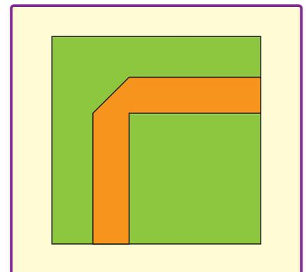
Fig.8. Top view of the layout of a corner geometry that can be used to minimise transmission line reflections.
