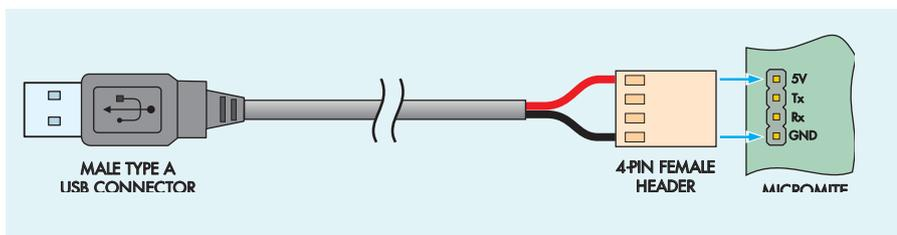
**Fig.4:** the *Touch-Screen Boat Computer* is powered from a 5V USB charger that's either plugged into a 12V cigarette lighter socket or wired permanently into the boat's power supply (see text). To make a suitable power cable, cut off one end of a USB cable, thread the cut end through a cable gland in the side of the case and solder it to a 4-pin female header connector.
