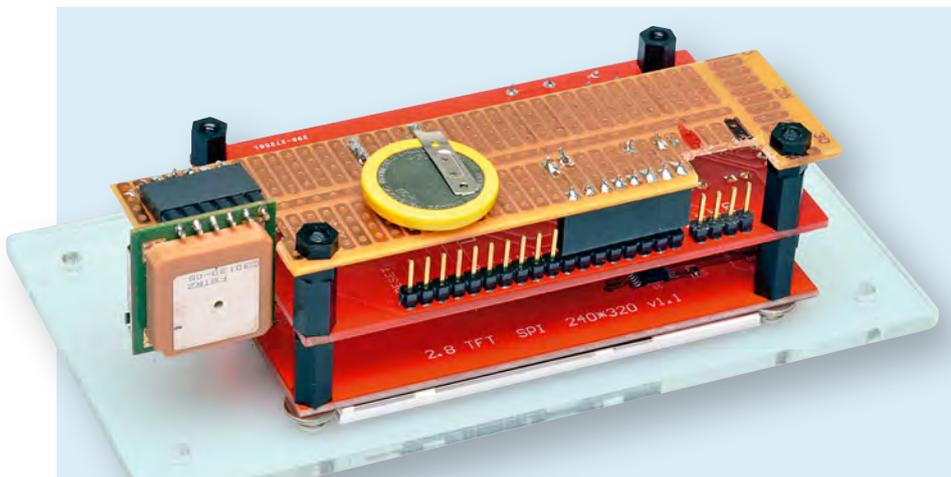
The GPS module used in the prototype required a separate back-up battery and this was also mounted on the strip-board. If you don't need a separate battery, you can simply glue the GPS module to the top of the case and run flying leads to an 8-way pin header to connect to CON2 on the *BackPack* PCB.
