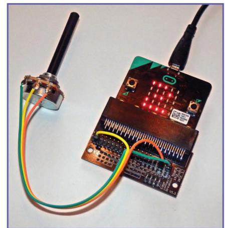
**Fig.3.2.** Connect the potentiometer to the micro:bit. The slider (yellow wire) is taken to the analogue input pin
