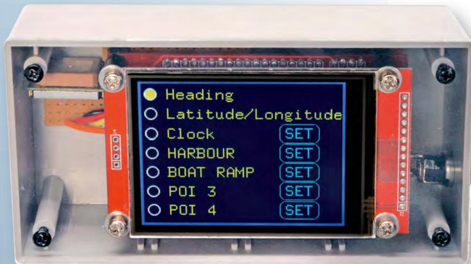
This photo shows the list of data that can be shown in the lower half of the main display. Touching any option switches the unit back to the main display, with the relevant data displayed in the lower half of the screen. Touching a SET button allows you to configure a particular entry (ie, to set the clock or configure a point of interest (POI)).
