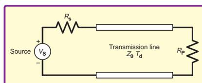
Fig. 1. Transmission line with source and load resistances
