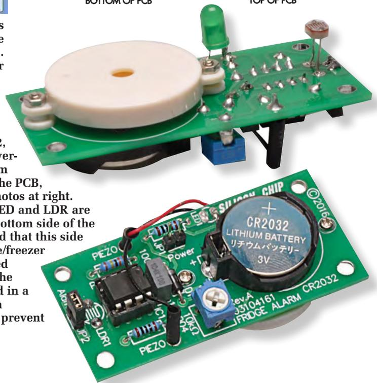
**Above right: Fig.2,** the component overlays for the bottom and top sides of the PCB, with matching photos at right. Only the piezo, LED and LDR are mounted on the bottom side of the PCB; it is intended that this side aim out the fridge/freezer door. As explained later in the text, the PCB was enclosed in a zip-loc bag with a desiccant to help prevent condensation.
