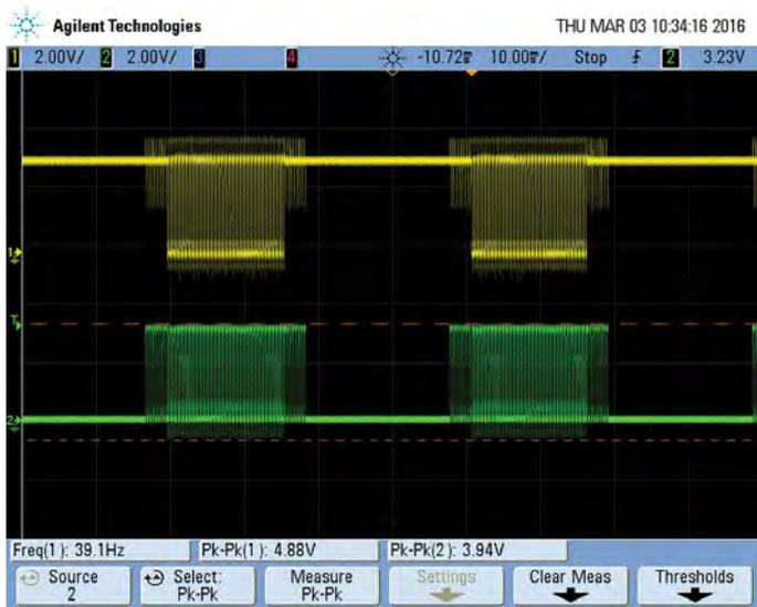
**Scope3:** Taken at the same sweep speed as in Scope2, this is the more complex ‘cricket’ alarm sound which we found to be more arresting (insistent, irritating, annoying – your choice). You can choose either alarm sound by having link JP2 in or out of circuit.
