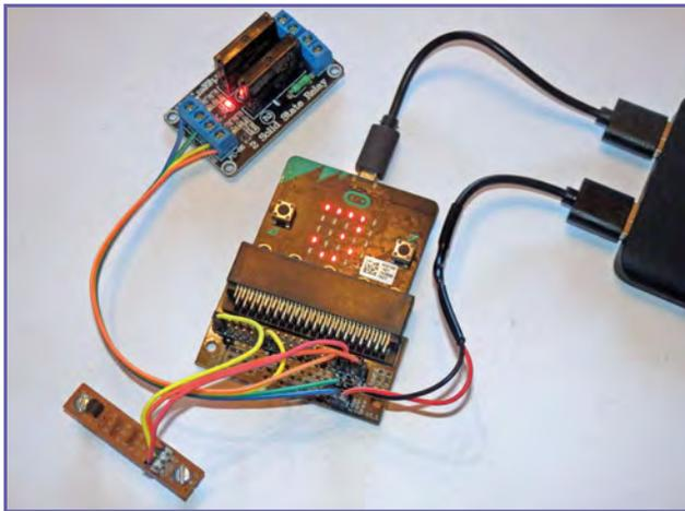
**Fig.3.12. Completed micro:bit thermostatic controller**
