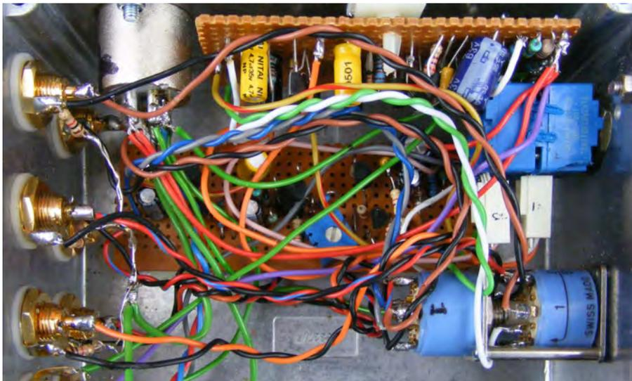
Fig.1. It doesn't have to be like this – use a proper loom.
