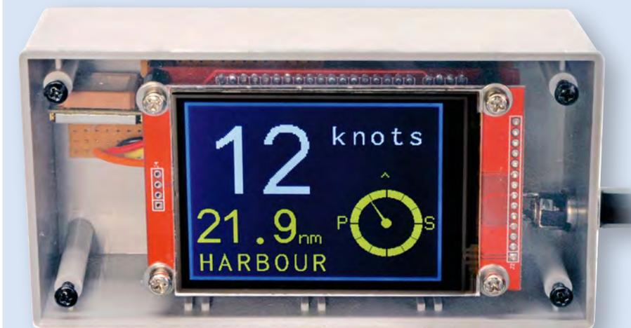
This is what the main screen looks like when a point of interest (POI) has been selected for the lower half. It shows the distance and the direction to the selected POI, in this case one named HARBOUR. To navigate to the POI, all you need do is steer in the direction of the pointer and watch the distance as it counts down to zero.
