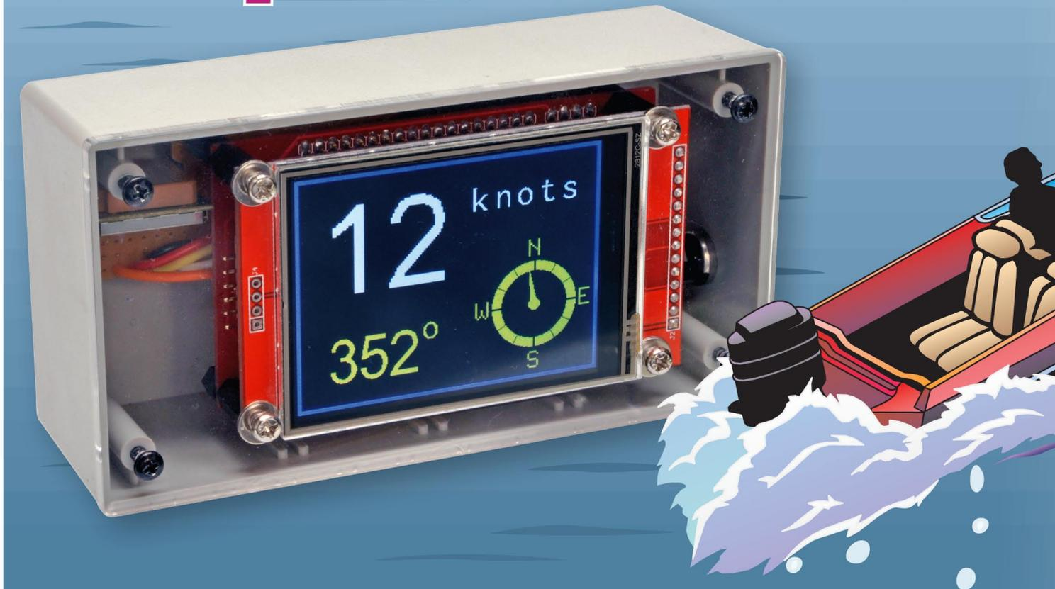
Would you like an accurate digital speedometer for your boat? One with a large clear display? This low-cost unit with touch control is just the shot. It can also display a raft of other information, including your heading, location and the relative bearing to a point of interest, which can be anything from the harbour entrance to a great fishing spot.
