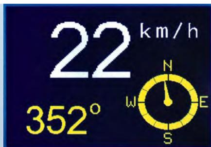
Fig.2: touching the top half of the screen shown in Fig.1 switches the speed indication from knots to km/h.
