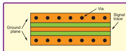
Fig.7. Via fences along the ground plane of a coplanar waveguide signal trace (top view)
