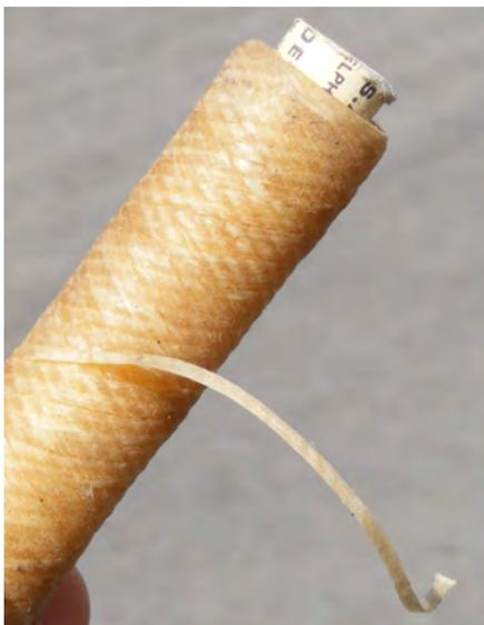
Fig.10. Wax-impregnated cord has superior gripping properties.
