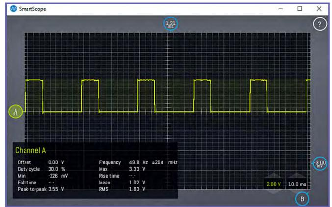
Fig.3.4. PWM output with 30% duty cycle
