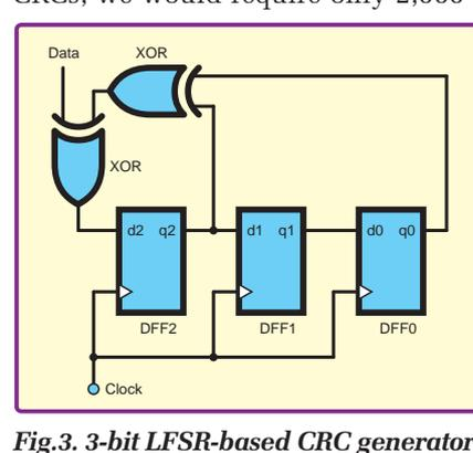
Fig.3. 3-bit LFSR-based CRC generator
