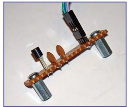
Fig.3.10. The TMP36 temperature sensor is mounted on a small piece of strip board
