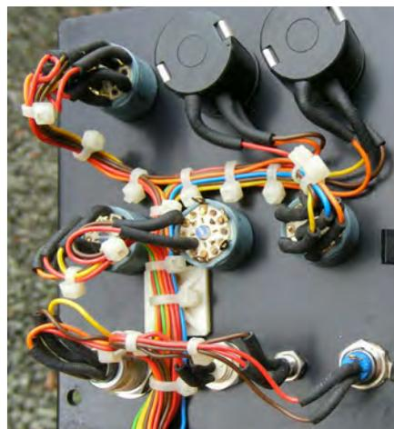
Fig.2. Suitable pathways for the loom around obstacles may take several attempts and can be developed with ties and pads, as in this loudspeaker magnetometer. When finalised, looms can be made up laced, ready for installation.
