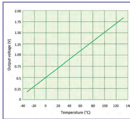
Fig.3.9. The TMP36 temperature sensor characteristic
