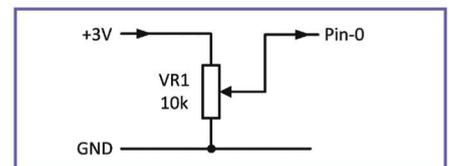
**Fig.3.1.** Testing the micro:bit's analogue I/O
