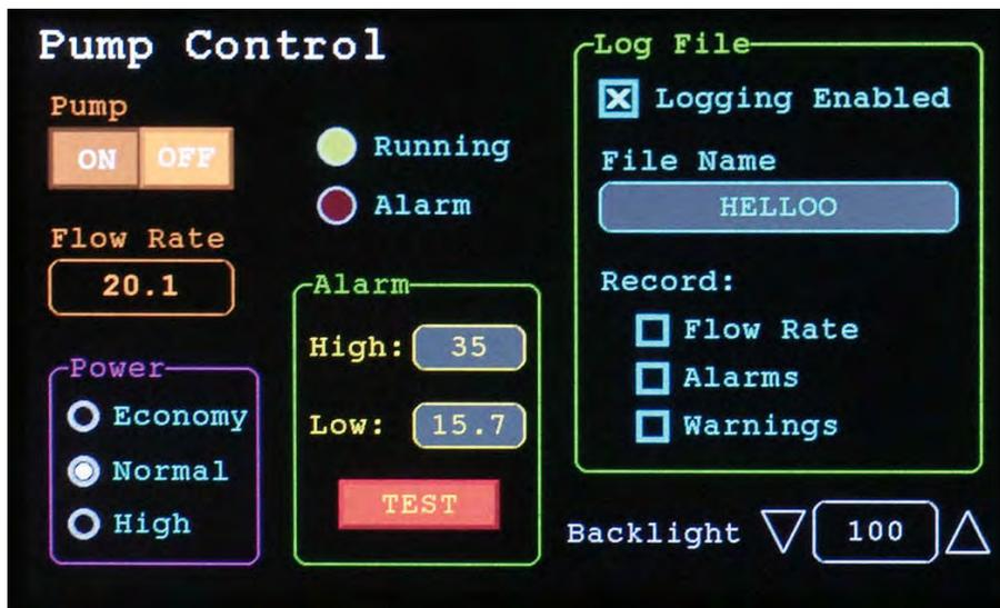
**Fig1:** this is an example of an on-screen control panel that can be created using the *Explore 64* and an LCD panel. Most objects on the screen are touch-sensitive and will react when touched. Each is created with a single BASIC command and from then on MMBasic will manage the display, including animating the objects when a user touches them. We will describe these GUI controls in detail in a later article.
