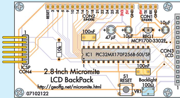
Fig.2: repeated from the May 2017 issue, this parts layout diagram shows how to build the *BackPack* PCB for the 2.8-inch LCD. Note that pin headers CON1 and CON2 are mounted on the rear of the PCB, while CON3 and CON4 are mounted on the top (see photos).
