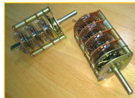
Fig.2. These well-made attenuator multi-way switches do a good job, but they are bulky and expensive (lower image courtesy of Fred Musset, http://a-direct-heating-triode.blogspot.co.uk )
