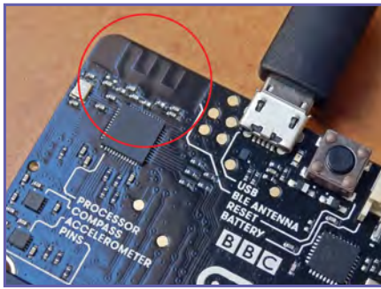
Fig.4.8. The printed antenna (hidden at the top edge of the micro:bit's PCB)
