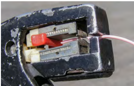
Fig.18. The Miller wire stripper, which is my favourite for stranded hook-up wire.
