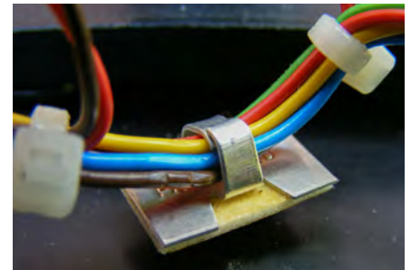
Fig.15. Self-adhesive clips are only temporary and must be avoided.
