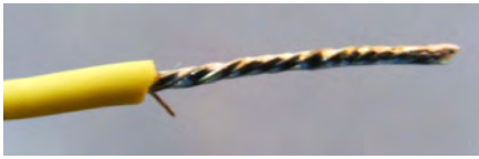
Fig.17. Broken/loose strands can easily cause shorts.
