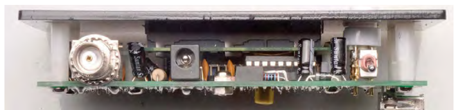
The view of the assembled PCB mounted on the front panel, from the input socket/DC supply/power switch side.
