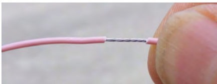
Fig.19. Twist the wire by turning the insulation. It gives a straighter result with no contamination.
