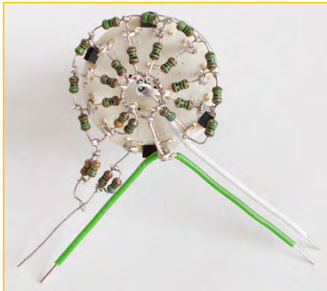
Fig.12. 600Ω attenuator (rear view) shown in Fig.10
