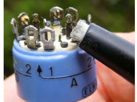
Fig.26. Clean dirty tags before tinning with a glass-fibre bush.
