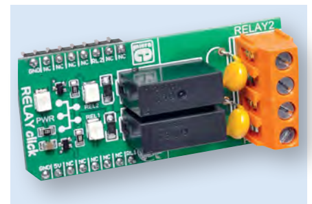
The Explore 100 has two sockets for mikroBUS Click boards, allowing a range of functions to be easily added to the Explore 100 (for example, the twin-relay board pictured here – there are lots more to choose from).
