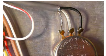
Fig.25. For screened wire, the braid conductor is normally the thickest, so it should be the shortest for strength.
