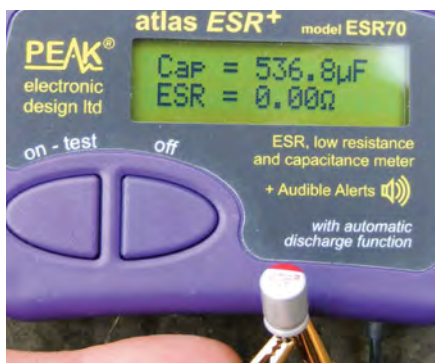
Fig.3. Solid polymer electrolytics give the lowest ESR; the best for power-rail decoupling
