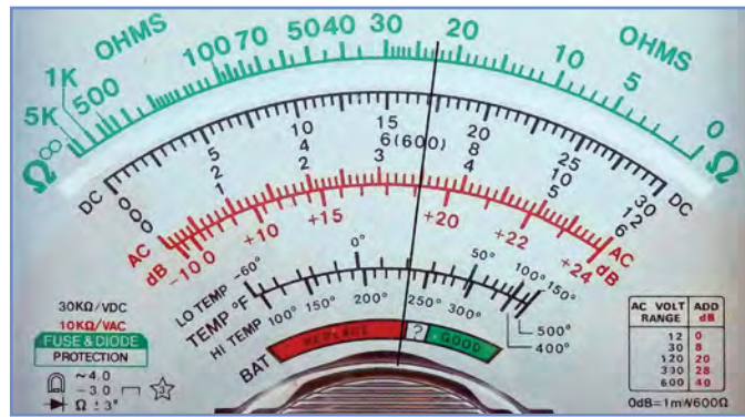
Fig.1.10. Reading the scale of an analogue multimeter
