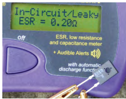
Fig.4. The ESR70 can be used to measure low-value resistors such as this 0.2Ω component.
