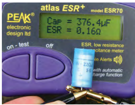
Fig.2. This old electrolytic may be in need of reforming – its nominal value is 220µF, but the meter reads 376µF
