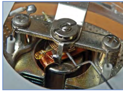
Fig.1.3. Internal arrangement of a typical moving-coil meter
