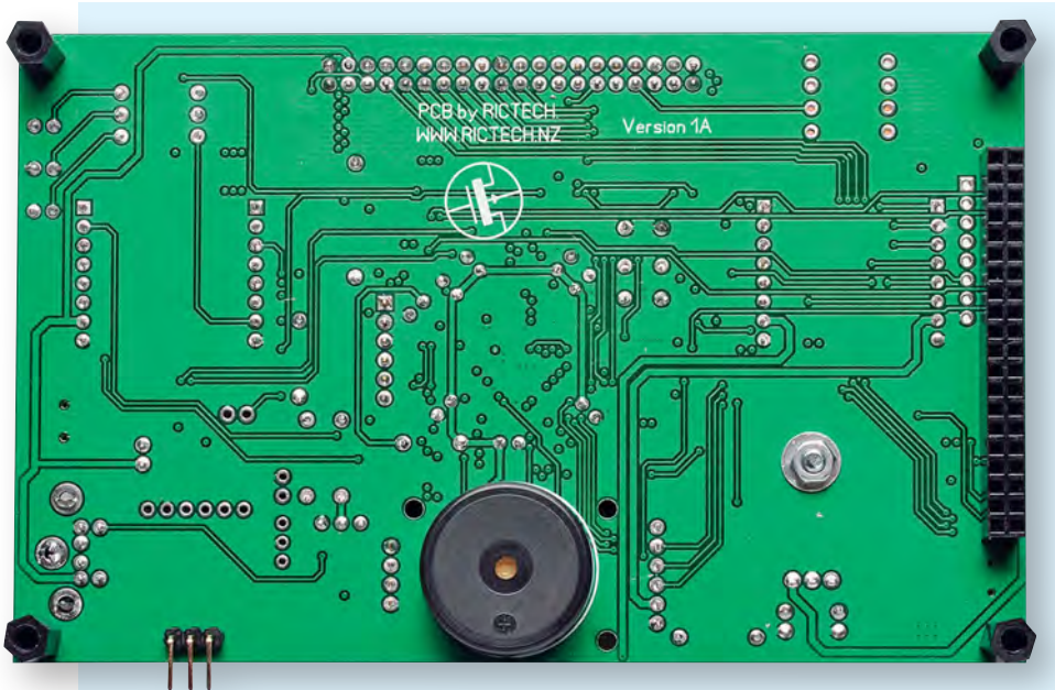
The piezo buzzer and the 40-way connector for the LCD panel mount on the rear of the PCB. The connector plugs directly into a matching pin header on the back of the 5-inch LCD panel (see photos and page 37, August 2017).
