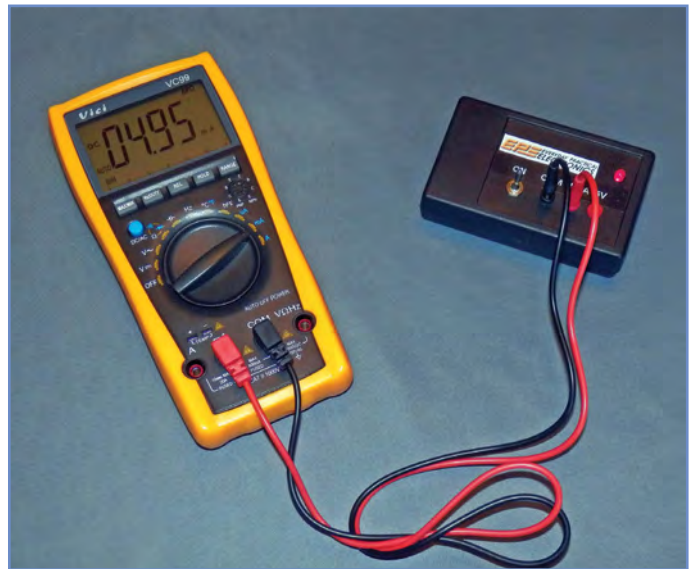
Fig.1.24. Checking the DC current function with the multimeter checker
