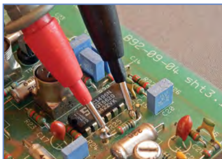
Fig.1.12. A set of properly insulated test probes is essential when making measurements on live circuits
