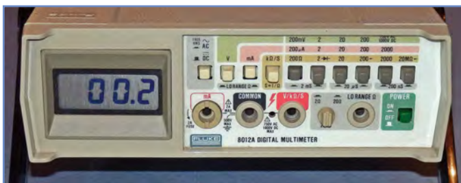
Fig.1.14. A laboratory-grade Fluke bench multimeter
