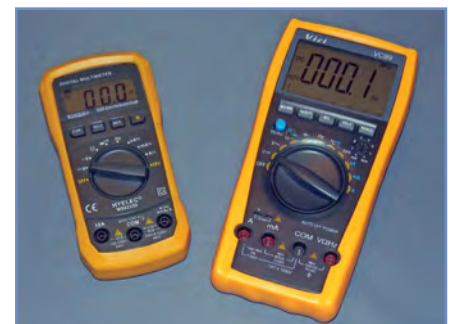
Fig.1.11. Two low-cost autoranging digital multimeters
