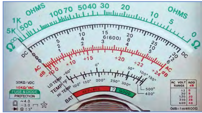
Fig.1.7. Scale of a typical analogue multimeter showing non-linearity of the resistance range (outer green scale marked 'OHMS')
