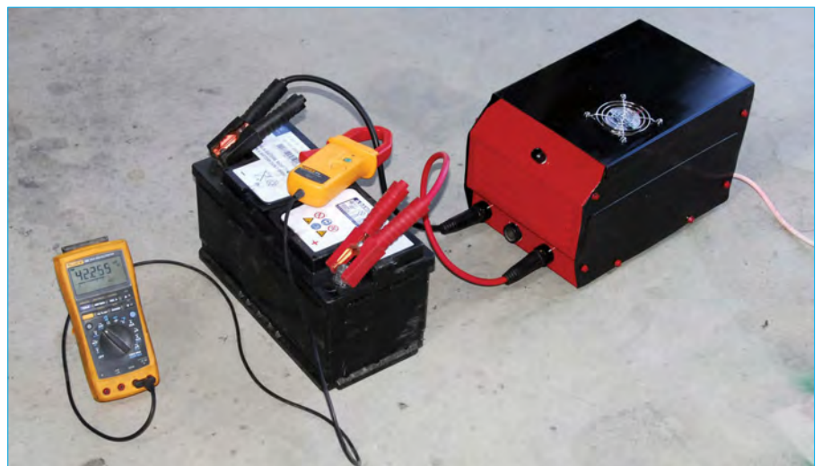
Here's the welder-battery charger pushing over 42A into a large car battery.
