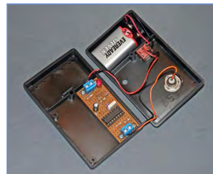
Fig.2.19. Internal wiring of the scope calibrator
