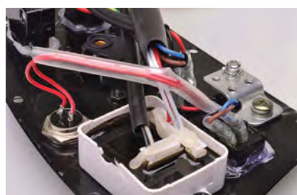
The modified control panel of the Powertech (Jaycar) 1kW Generator. At left is the two-pin microphone socket we added (about the only spot possible!). Centre is a close-up of the wiring and right is the panel about to go back in.
