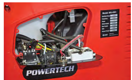
The modified control panel of the Powertech (Jaycar) 1kW Generator. At left is the two-pin microphone socket we added (about the only spot possible!). Centre is a close-up of the wiring and right is the panel about to go back in.
