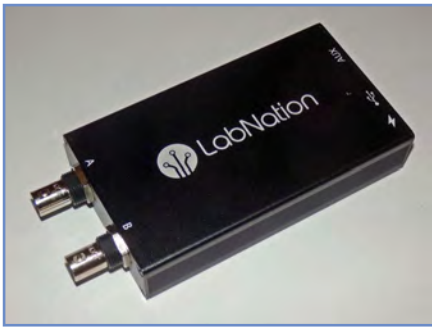
Fig.2.8. High-performance dual-channel USB DSO with a sampling rate of 2 \times 100M samples per second. SmartScope can be used with a wide range of operating systems, currently including Windows, Linux, OS X, Android and iOS
