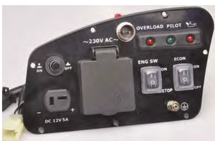
The modified control panel of the Powertech (Jaycar) 1kW Generator. At left is the two-pin microphone socket we added (about the only spot possible!). Centre is a close-up of the wiring and right is the panel about to go back in.
