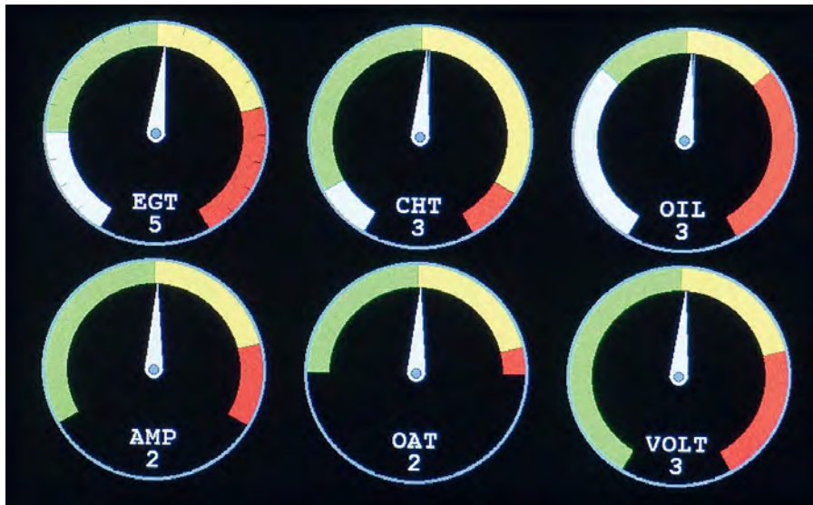
Fig.3: it's easy to show a lot of information on a single screen if using a large LCD panel. This is a simulation of an engine monitor, and although you cannot see it in the photograph, the meters update in real time with a smooth response.
