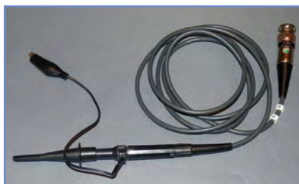
Fig.2.12. Typical x1 and x10 scope probe
