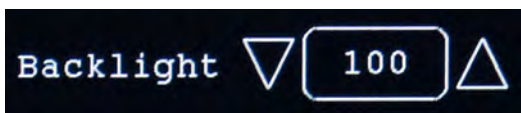
Fig.4: the SPINBOX control consists of a box displaying a number and up and down arrows at each end. It acts like a potentiometer; when either the up or down arrow is pressed, the number will increment or decrement by a set amount. If the touch is held down, the increment or decrement process will repeat at a fast rate.
