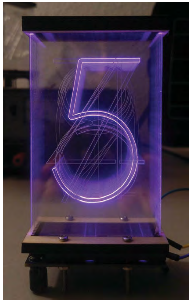
Fig.2. An LED-based Lixie display (Source: Connor Nishijima)
