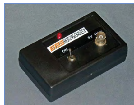
Fig.2.21. External appearance of the finished scope calibrator
