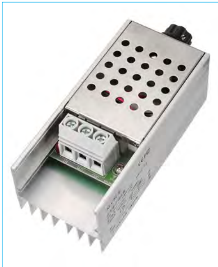
Making possible the conversion of a welder into a high current battery charger is this 10kW SCR module that costs under £10. It's used to adjust the primary transformer current.
