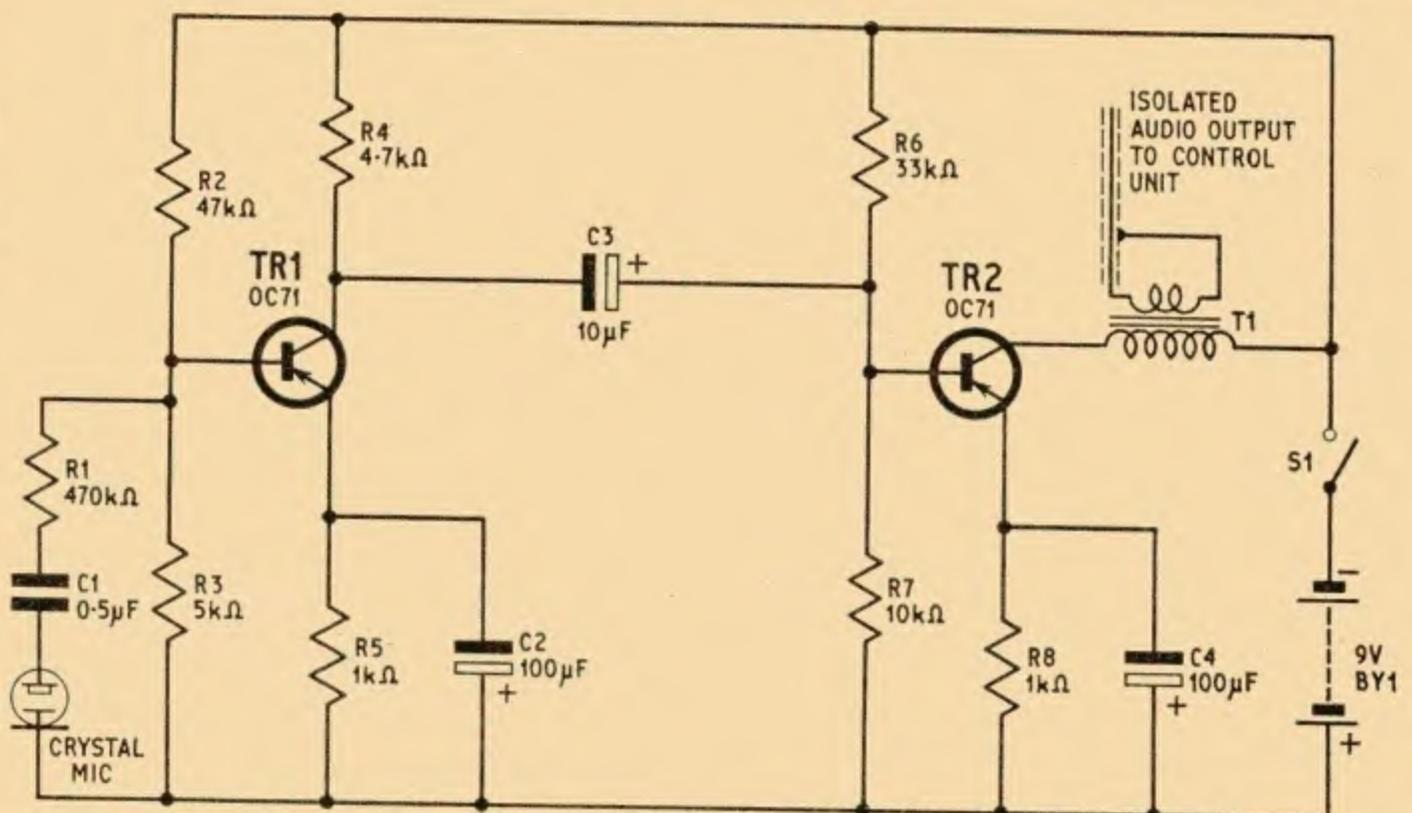
Fig. 1. Circuit of the microphone pre-amplifier which is situated close to the child
