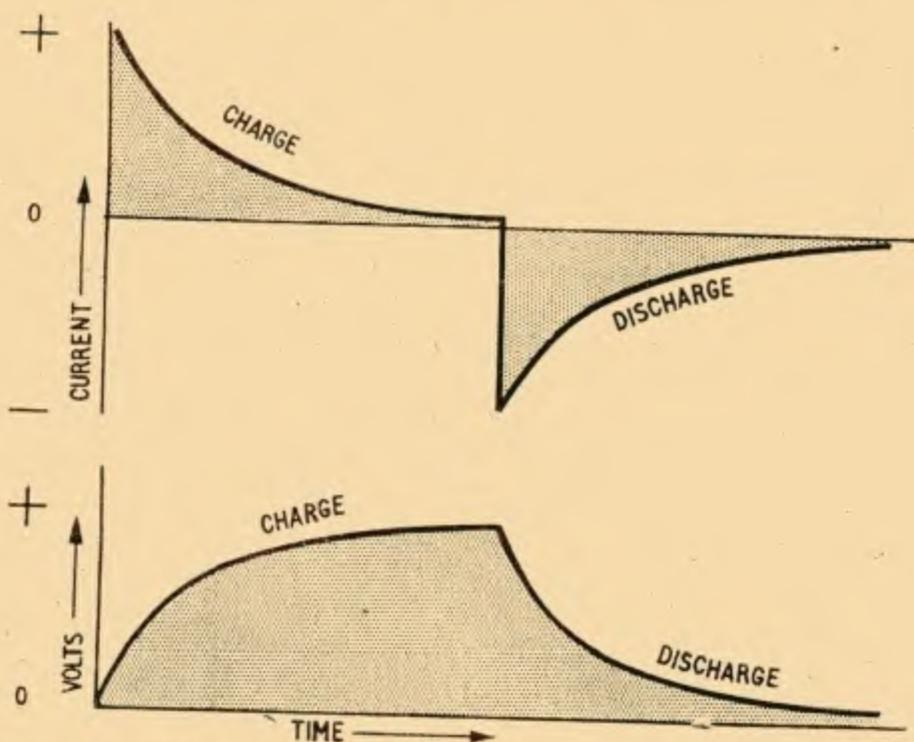
Fig. 4.4. The charging and discharging action of a capacitor is made clear by these curves
