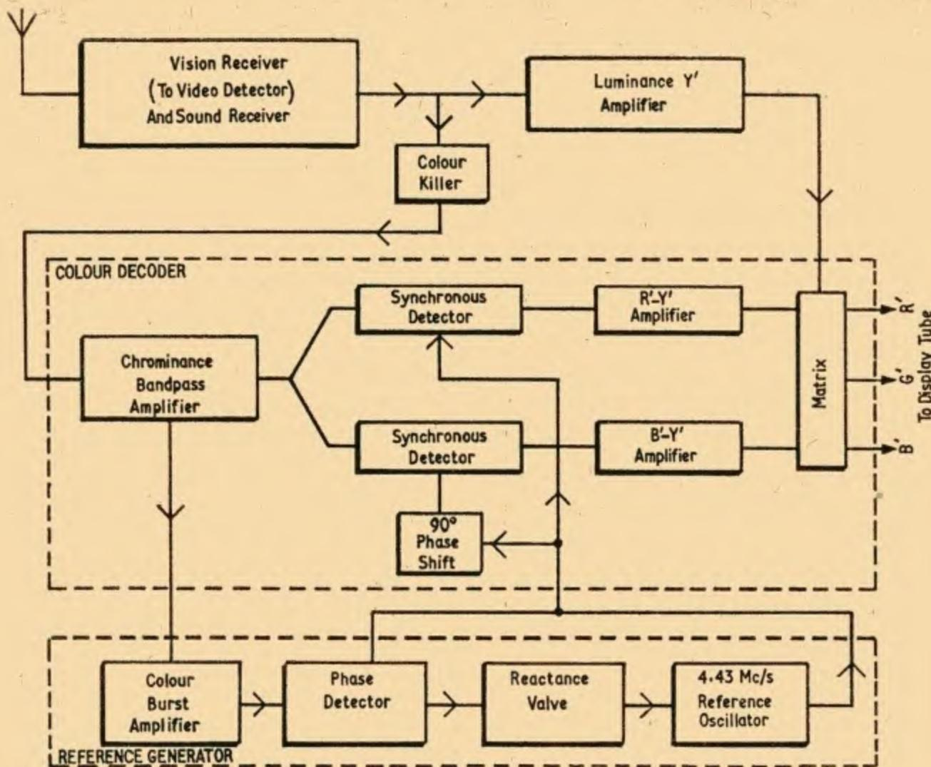
Fig. 1. Basic outline of a typical NTSC receiver
