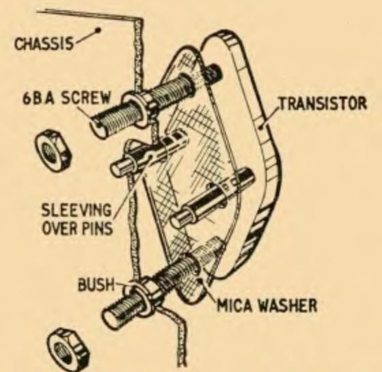
Fig. 3. Exploded view of the transistor mountings showing the insulation bushes and washer
