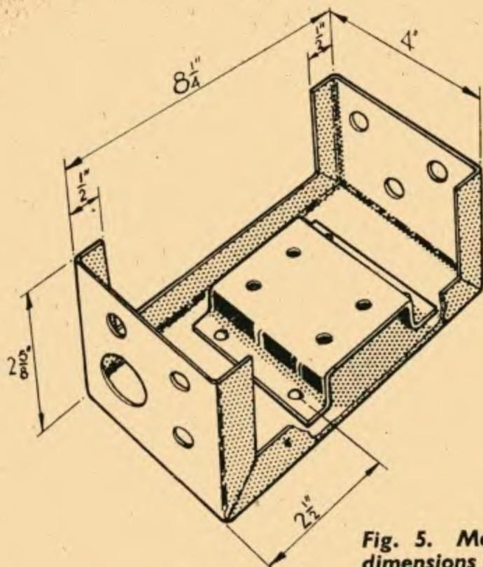
Fig. 5. Main chassis dimensions and drilling details of the transformer mounting plate
