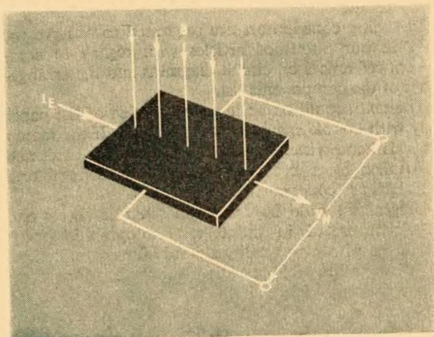
wherever units appear in this article they will be based upon this system. This gives " $I$ " in amps, " $B$ " in webers per square metre,  $V_H$  in volts and  $K$  in volts metre<sup>2</sup> per amp weber.
