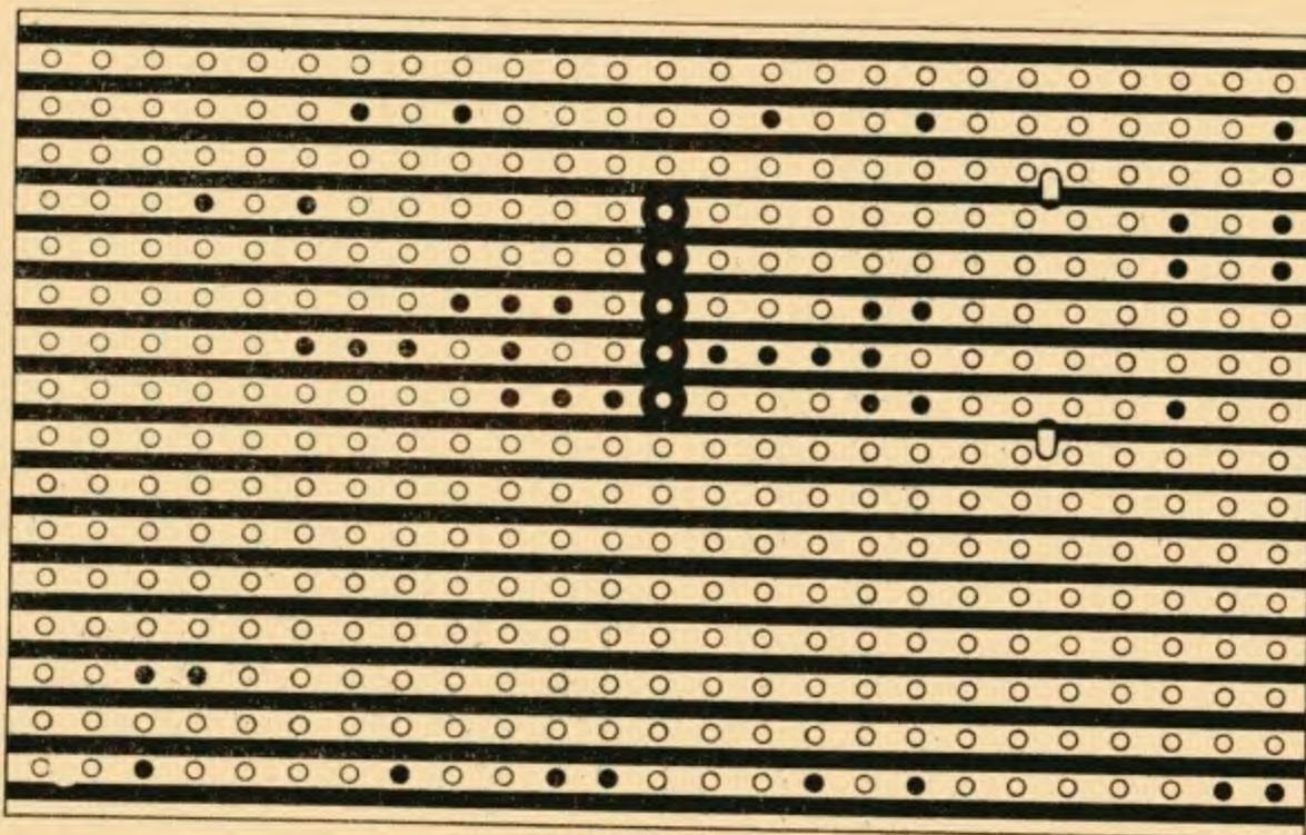
Fig. 5. Underside view of the pre-amplifier unit showing the breaks in the copper strips. The black dots indicate the holes which are used for component wiring
