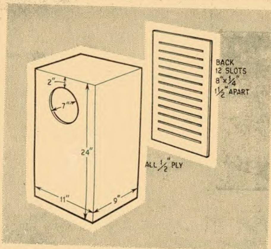
Fig. 6. External dimensions of 1 cu ft enclosure
