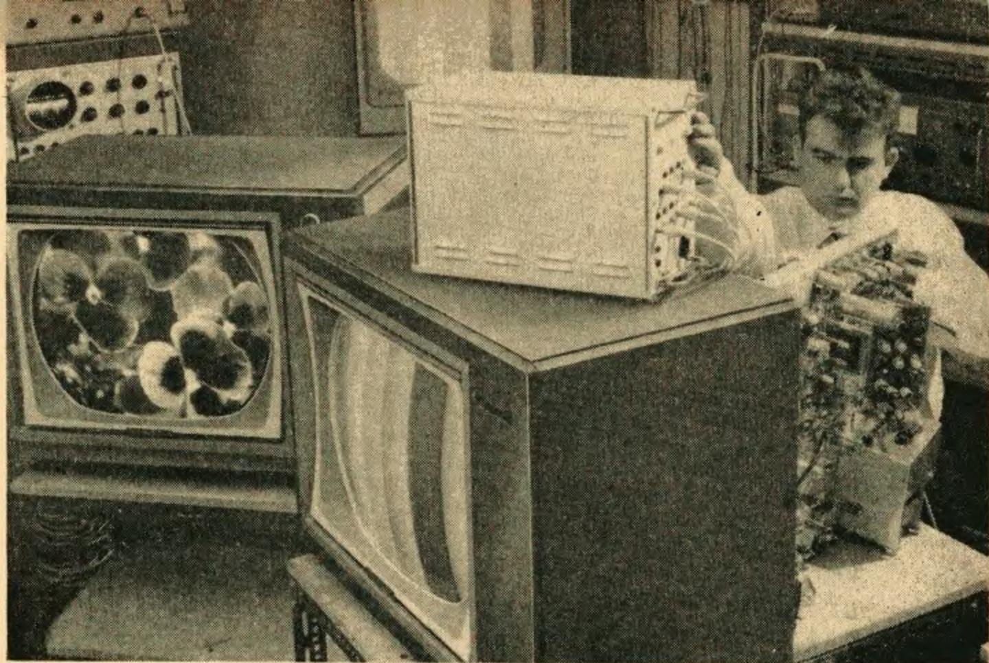
SECAM colour receivers being set up by means of a newly developed CFT waveform generator
