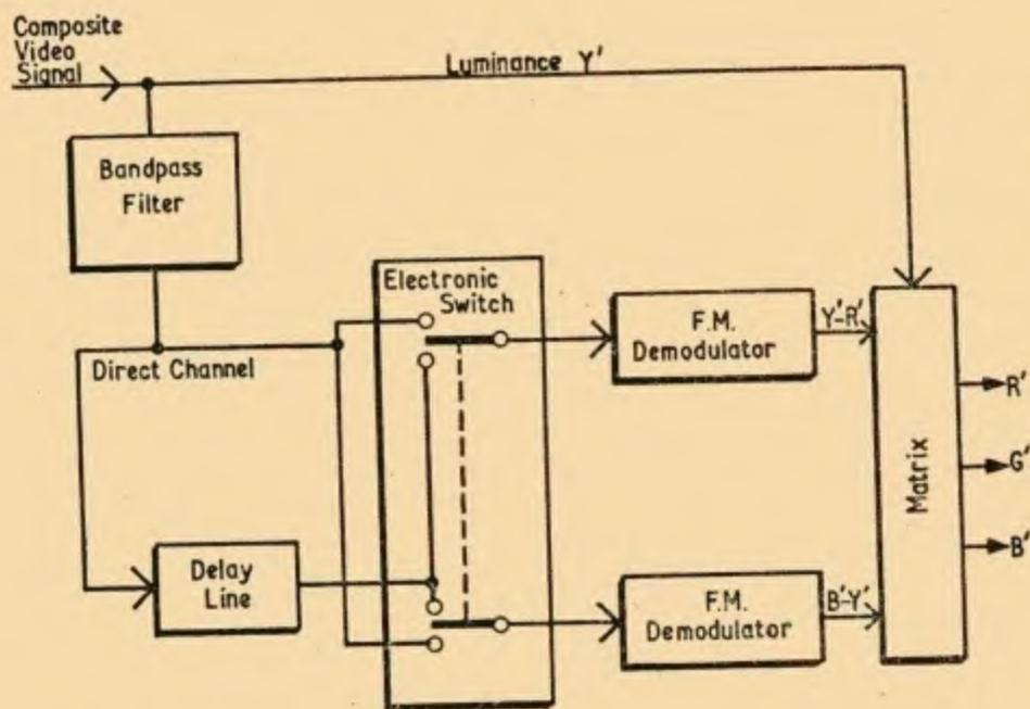
Fig. 2. Simplified decoder for SECAM receiver
