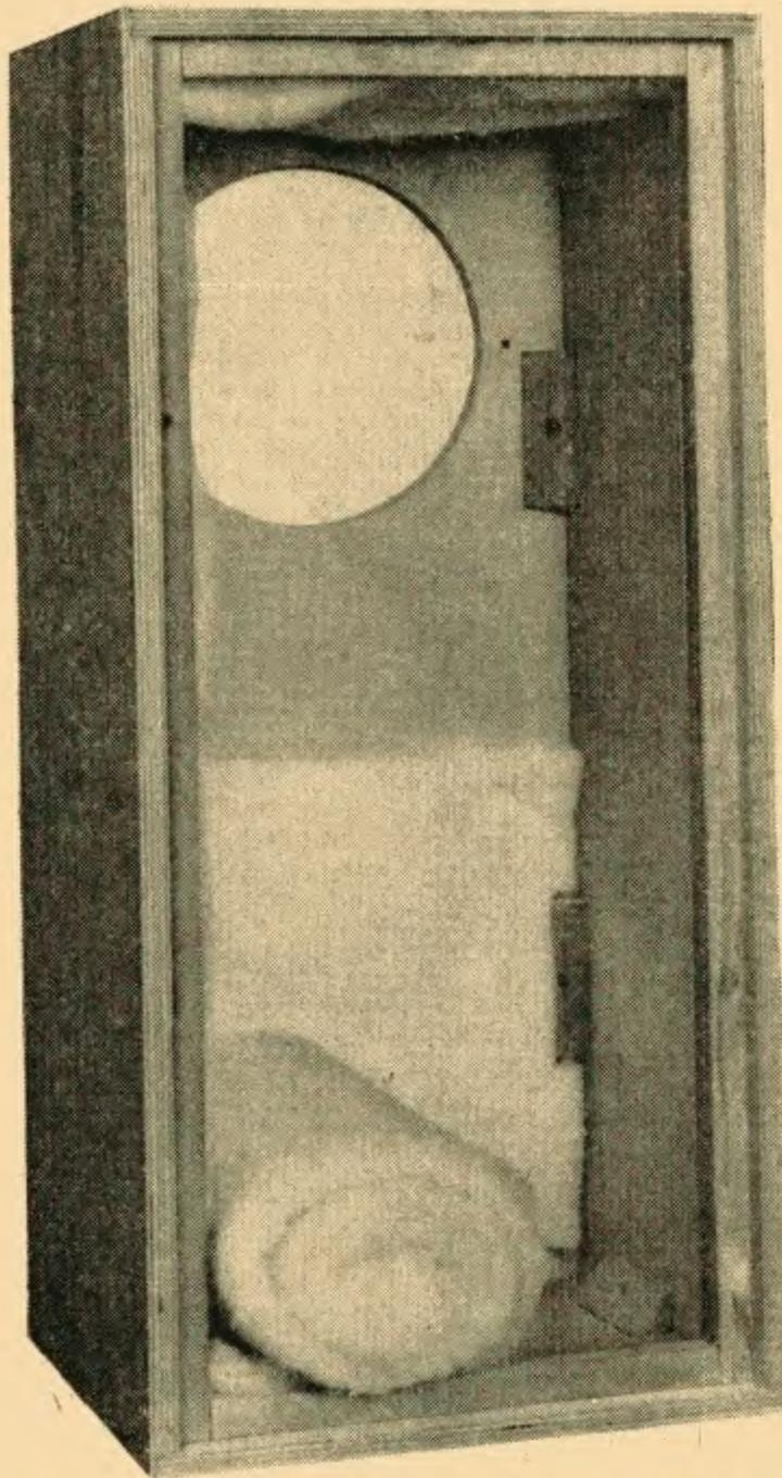
Fig. 10. Rear view of 1 cu ft enclosure with rear panel removed, and absorbent material rolled back to show triangular blocks and fixing rail
