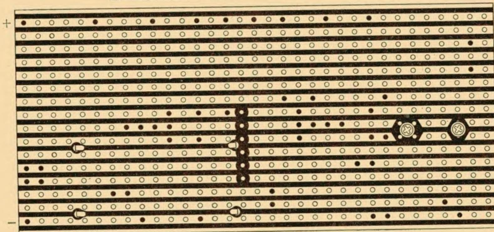
Fig. 7. Underside view of the control unit. The black dots indicate the holes which are used for component wiring
