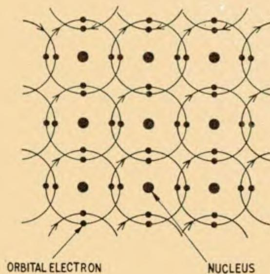
Fig. 1.2. Doping of germanium with arsenic results in one electron becoming "free"
