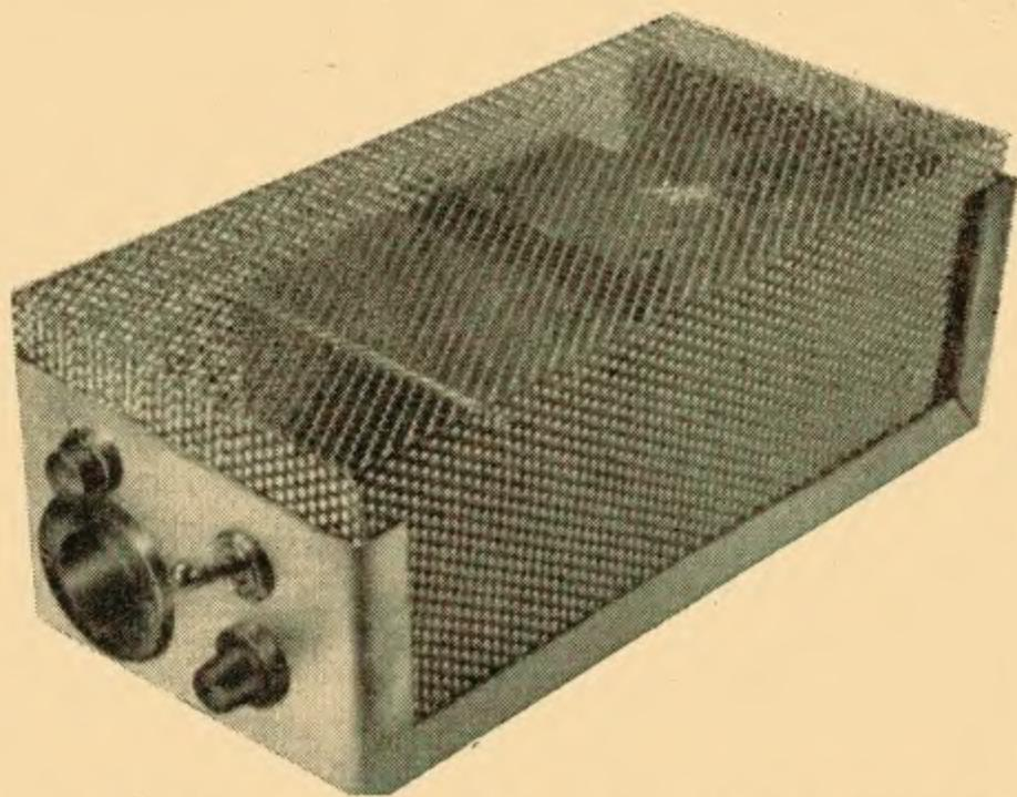
**T**HIS INVERTER is designed to operate from a 12V d.c. source to provide an output of 230V a.c. at about 65 to 70mA current (i.e. an output of approximately 15W). The design is based on readily available components to which a few refinements have been added, including d.c. and a.c. fuses, on/off switch, a.c. mains plug, indicator lamp, d.c. supply terminals and a diode to prevent damage through reverse connection of the d.c. supply.
