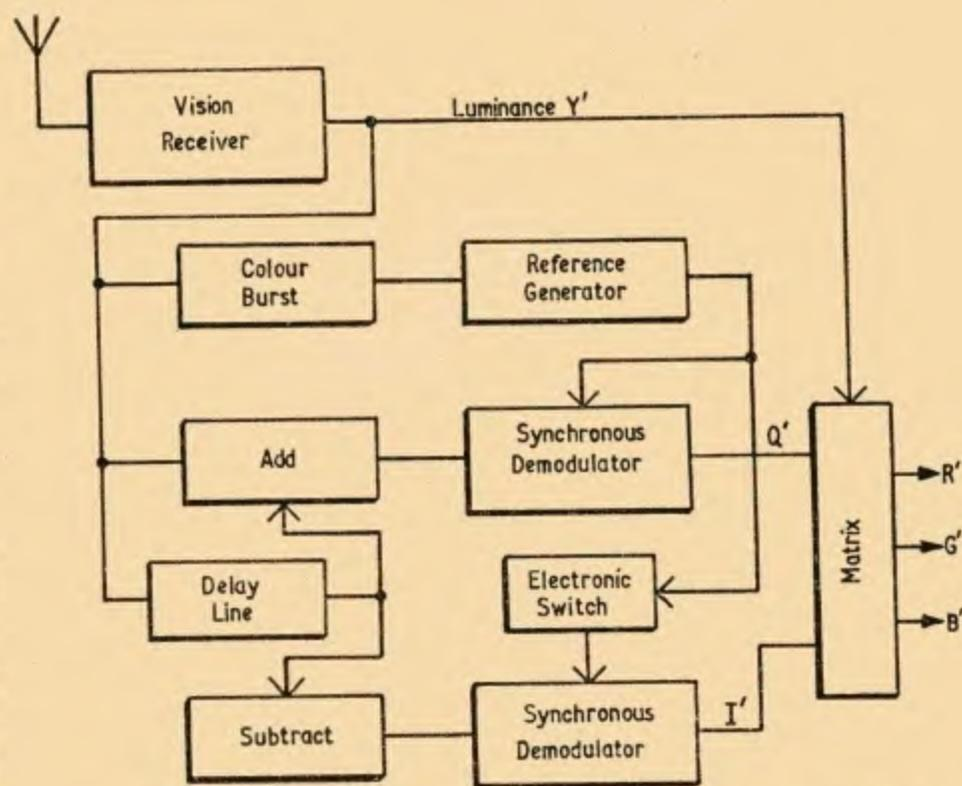
Fig. 3. Simplified decoder for "PAL de Luxe" receiver
