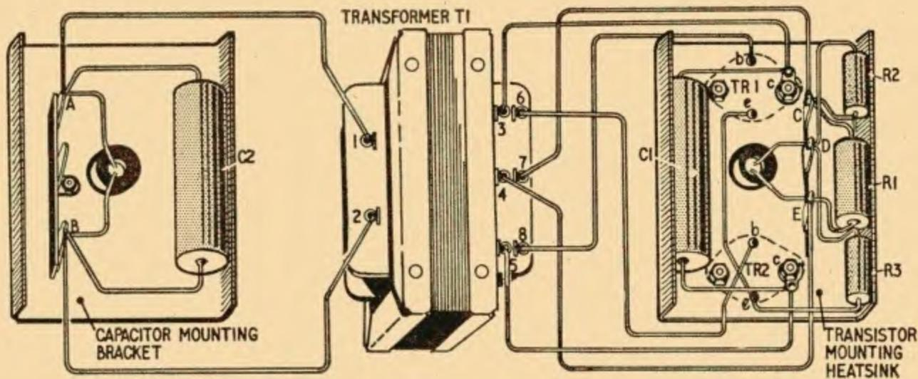
Fig. 2. Wiring diagram of the transformer and transistors
