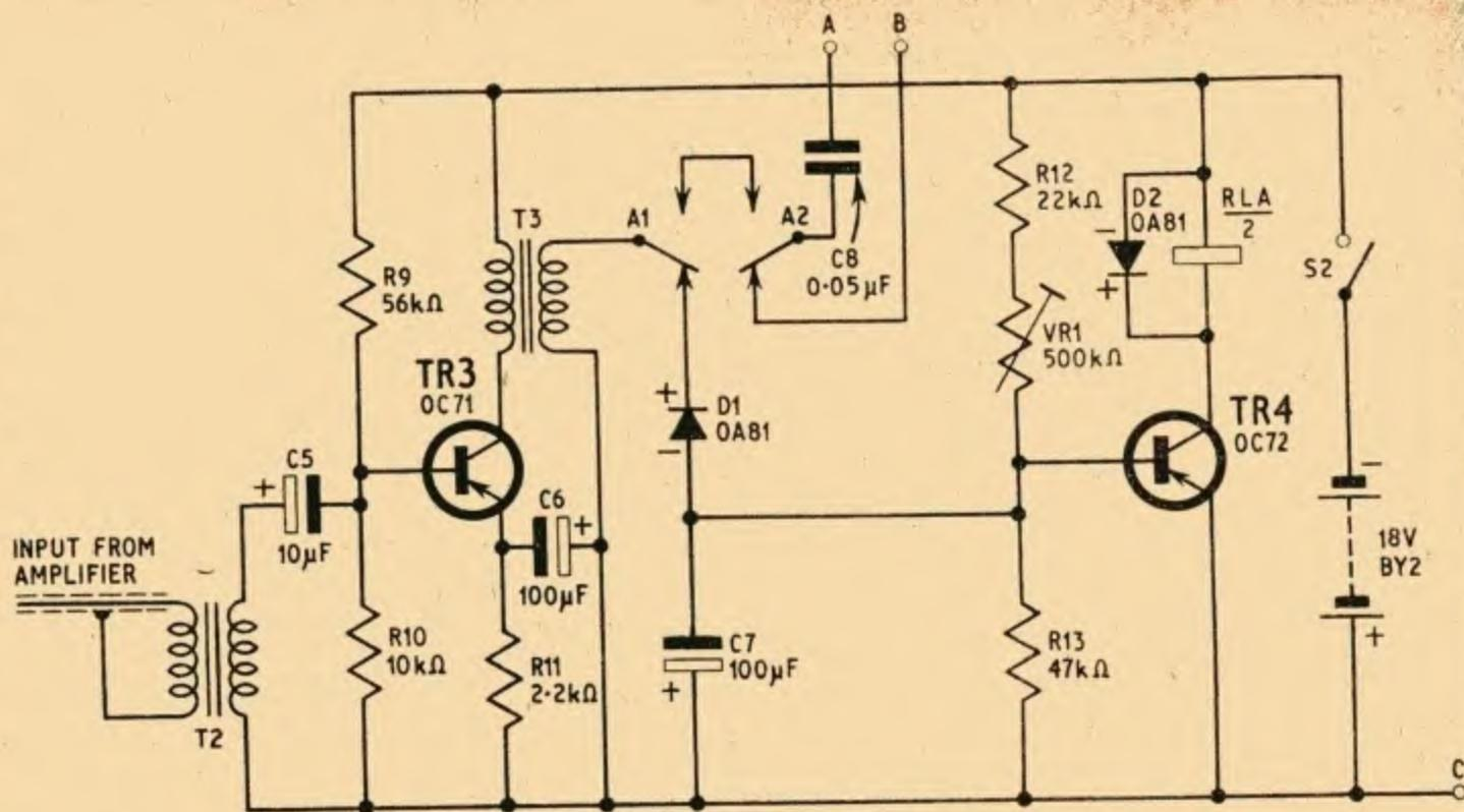
Fig. 2. Circuit of the control unit to be mounted in the broadcast receiver
