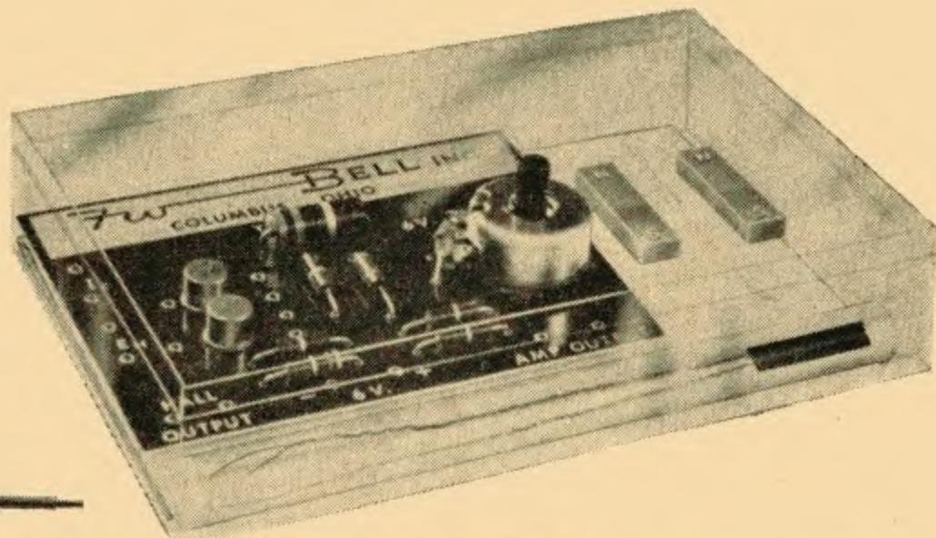
Fig. 4. Hall effect kit suitable for experimental use
