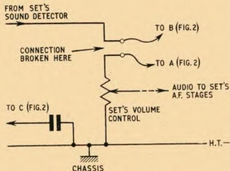
Fig. 3. Modification to the television or radio volume control circuit to accept the control unit
