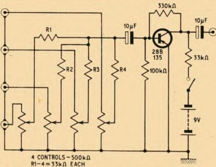
Fig. 4.4. Four-channel transistorised mixer
