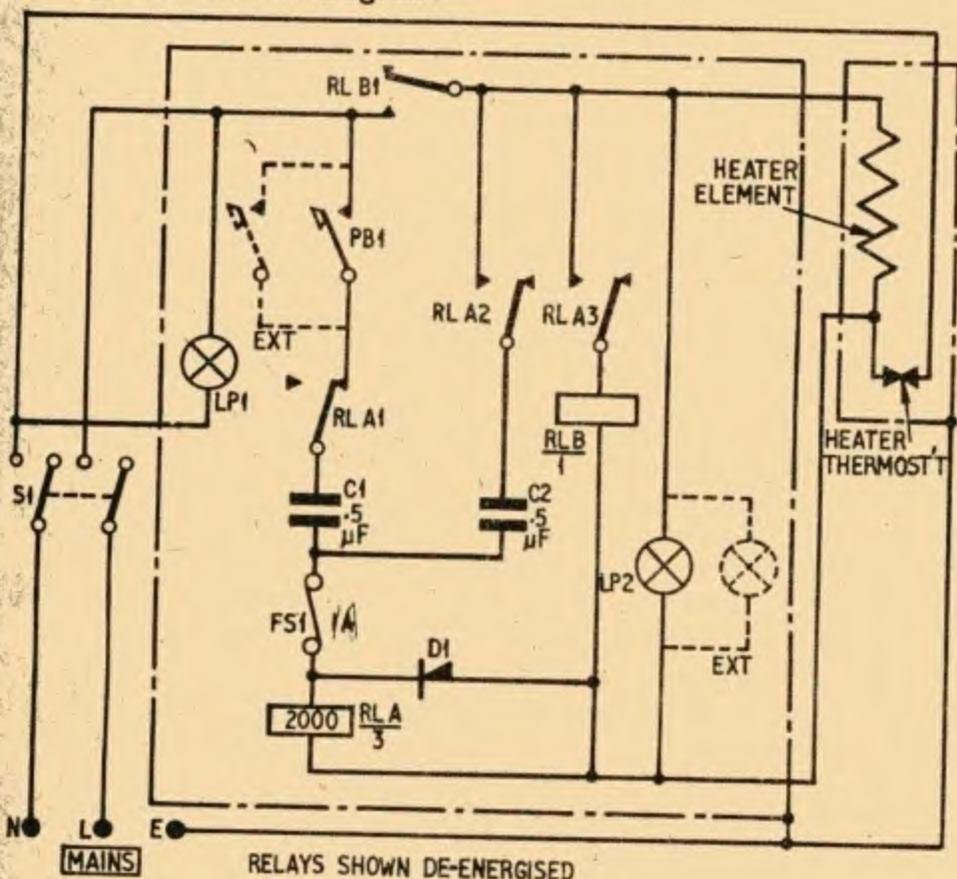
The function of diode D1 is to develop a d.c. voltage across the relay A. Capacitors C1 and C2 act as voltage droppers. Resistors could of course be used for this purpose, but arrangements for adequate cooling of the unit would then have to be made.
