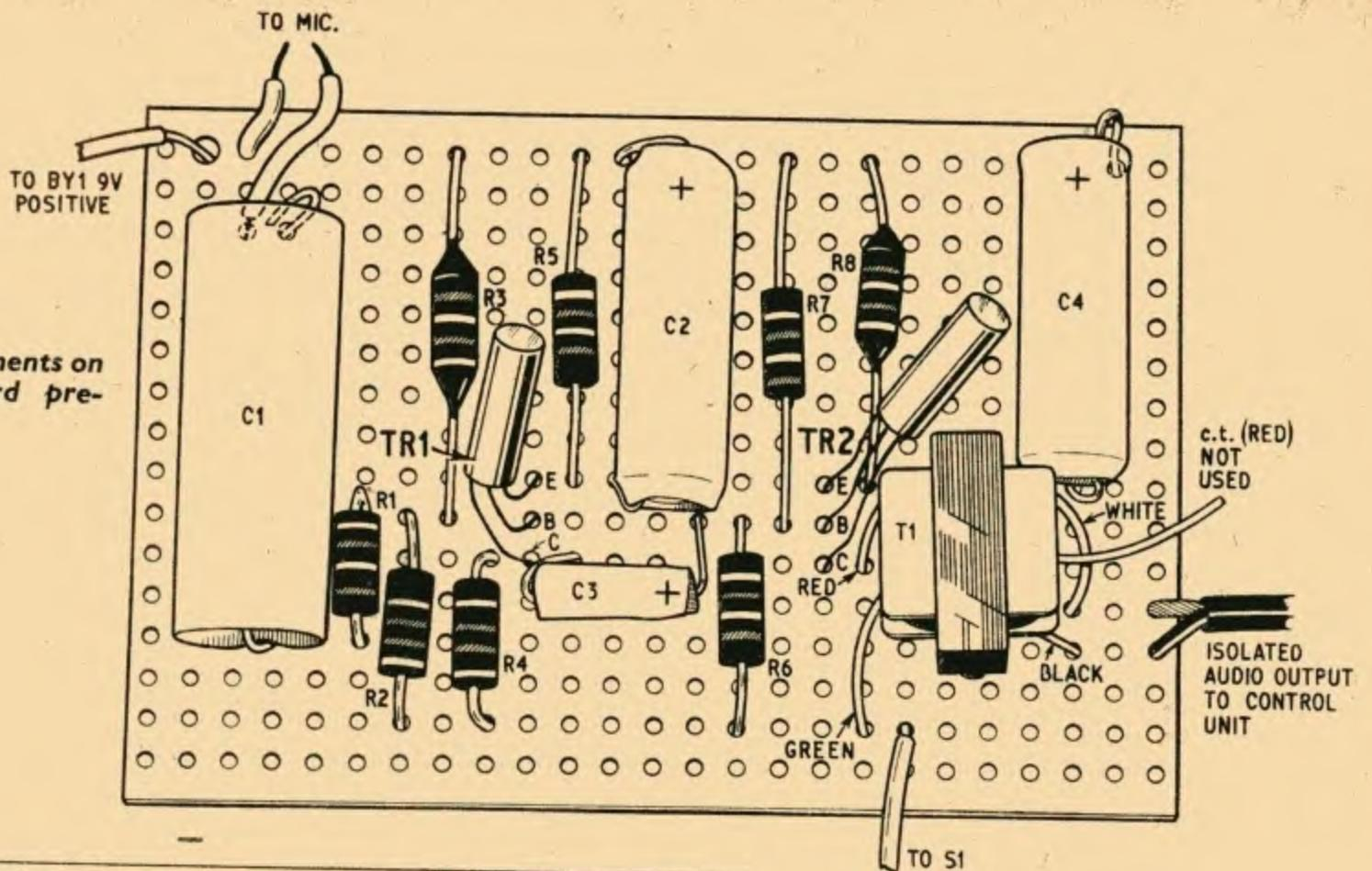
Fig. 4. Layout of components on the printed wiring board pre-amplifier unit
