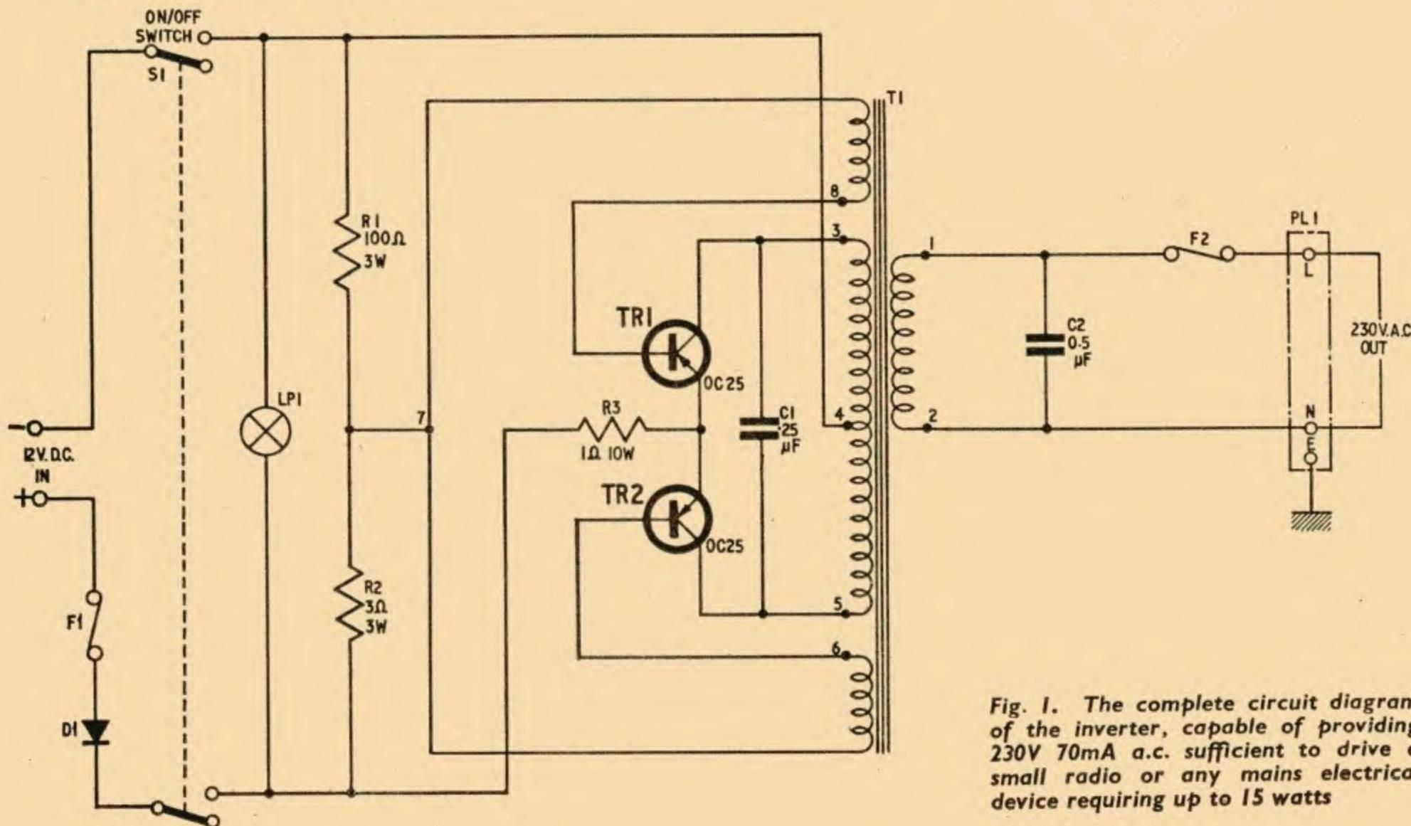
Fig. 1. The complete circuit diagram of the inverter, capable of providing 230V 70mA a.c. sufficient to drive a small radio or any mains electrical device requiring up to 15 watts
