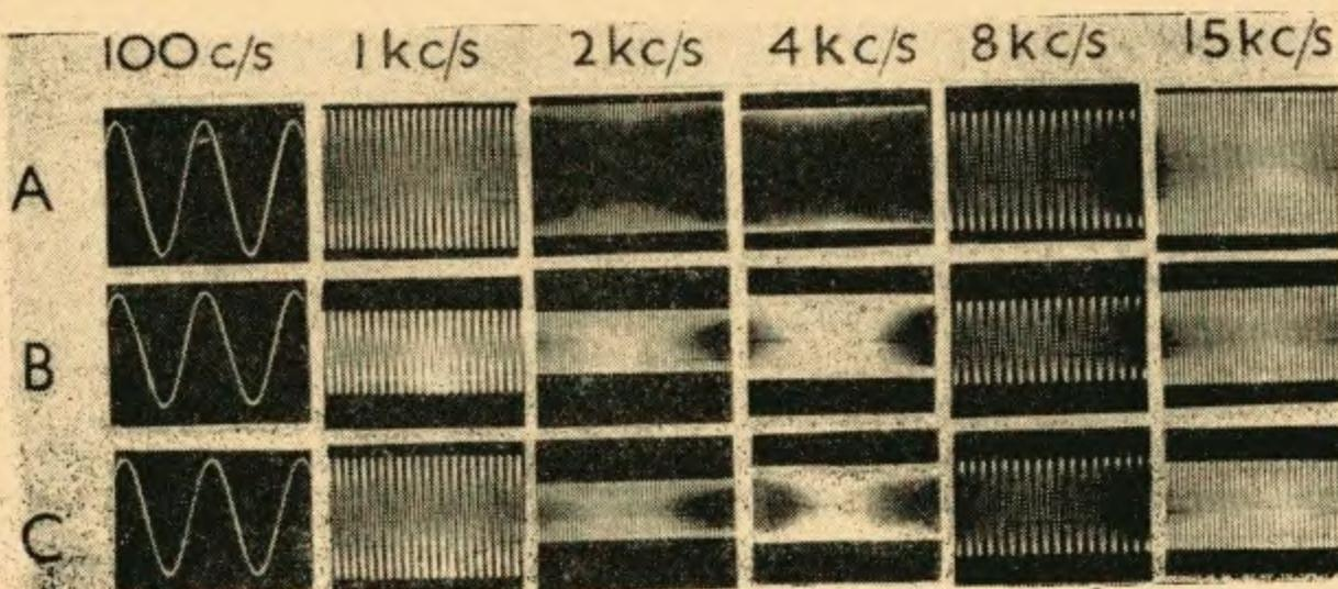
Fig. 11. Attenuation of loudspeaker output due to different covering materials
