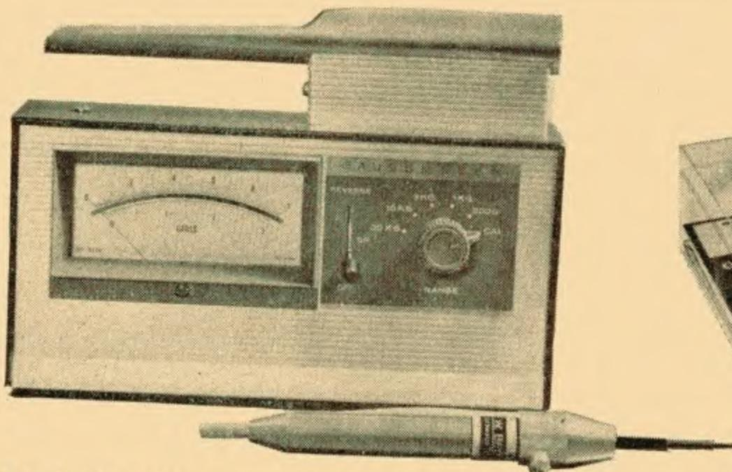
Fig. 3. A modern gaussmeter using indium arsenide as the Hall device
