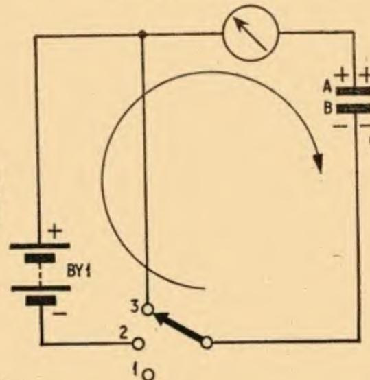
Fig. 4.1 (far left). This illustrates charging of a capacitor C by the battery BY1
