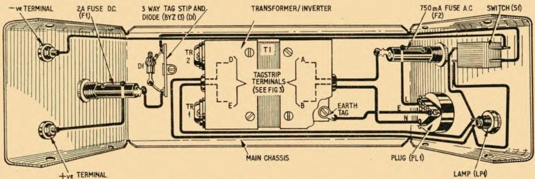
Fig. 4. Main chassis wiring diagram showing input and output connections
