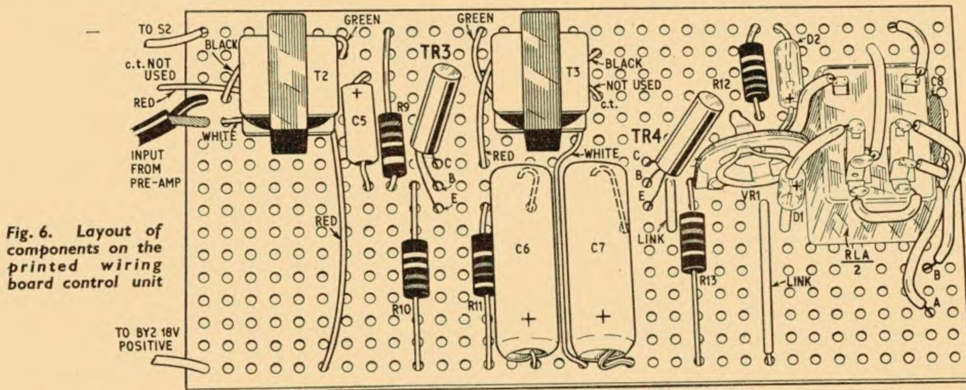
Fig. 6. Layout of components on the printed wiring board control unit
