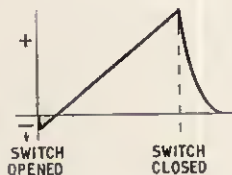
Fig. 8.4b. Output waveform of the Miller integrator circuit
