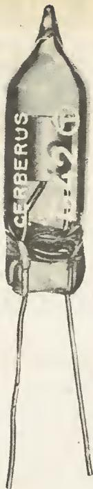
The G42 switching diode designed mainly for use in timer circuits (Cerberus A.G.)
