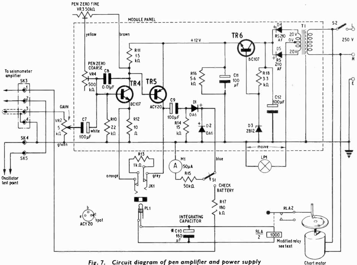
Fig. 7. Circuit diagram of pen amplifier and power supply
