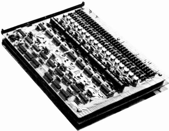
*Basic memory module of the Plessey Planar 850 core memory built on three printed circuit boards*
