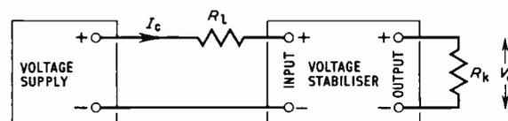
Fig. 8. The stabiliser being used to provide a constant current
