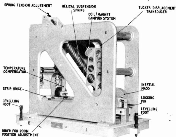
Fig. 4. A professional seismometer
