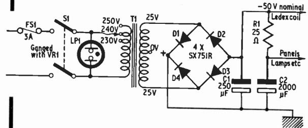
Fig. 6. Circuit diagram of the power supply (stage one)
