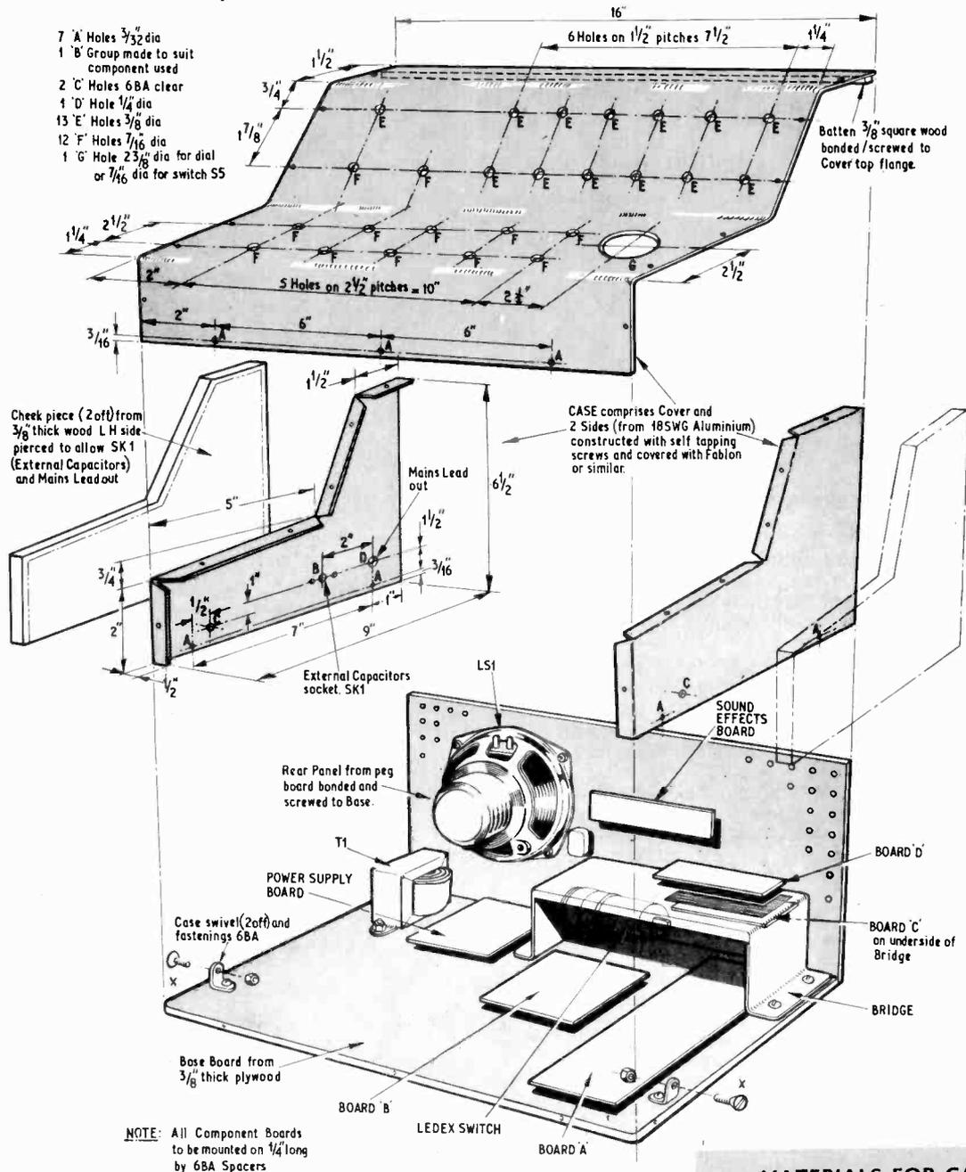
Fig. 4. Construction details of the case and baseboard layout
