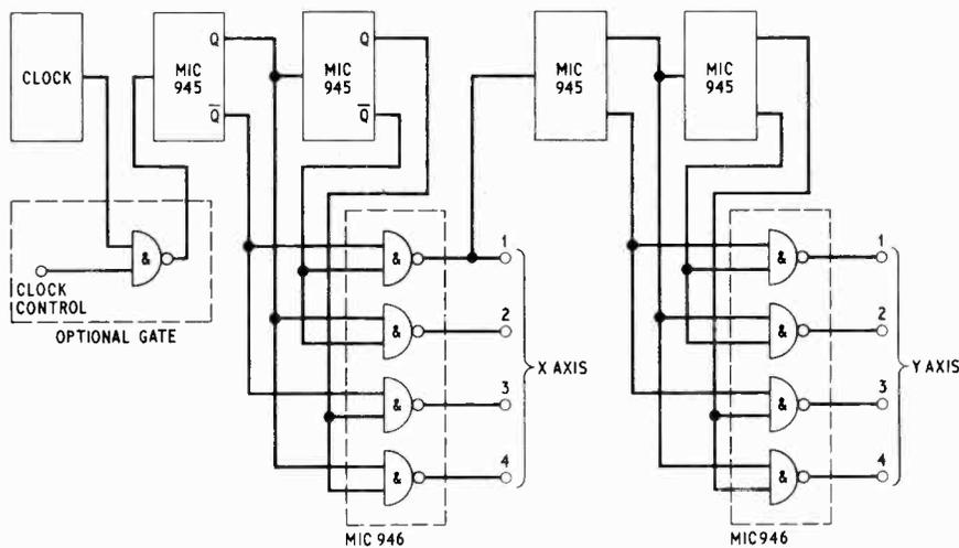
**Fig. 3.** Using the output from one of the gates of Fig. 2 to drive an identical system, we can sequentially switch on every lamp in turn in a 4 × 4 lamp matrix
