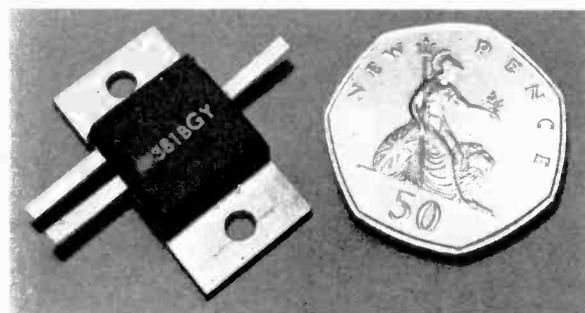
One of the new u.h.f. amplifier modules by Mullard compared with a 50 pence piece (above)
