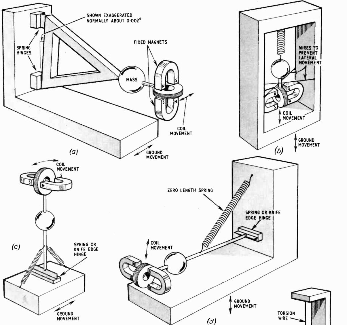
Fig. 5. The five seismometer structures that can be used: (a) horizontal pendulum, (b) mass-spring pendulum, (c) vertical pendulum, (d) spring pendulum, (e) torsion pendulum
