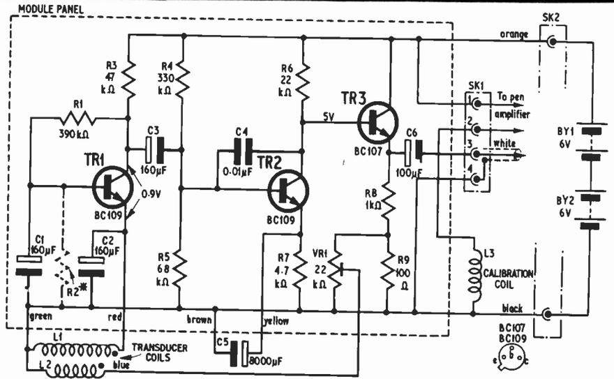
Fig. 6. Circuit diagram of low noise seismometer amplifier
