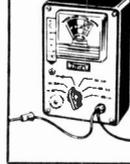
Made by Mallory but suitable for all batteries made by Ever Ready and others, most of which are zinc carbon types but also mercury manganese-nickel-silver oxide and alkaline batteries may be tested. The tester puts a dummy load on the battery and the meter scale indicates the condition depending upon which section the pointer rests. The section reads "replace", "weak" or "good". The tester is complete in its case, size 3 1/2 x 6 1/2 x 2 in with leads and prods. Price £1-75 plus 20p postage.
