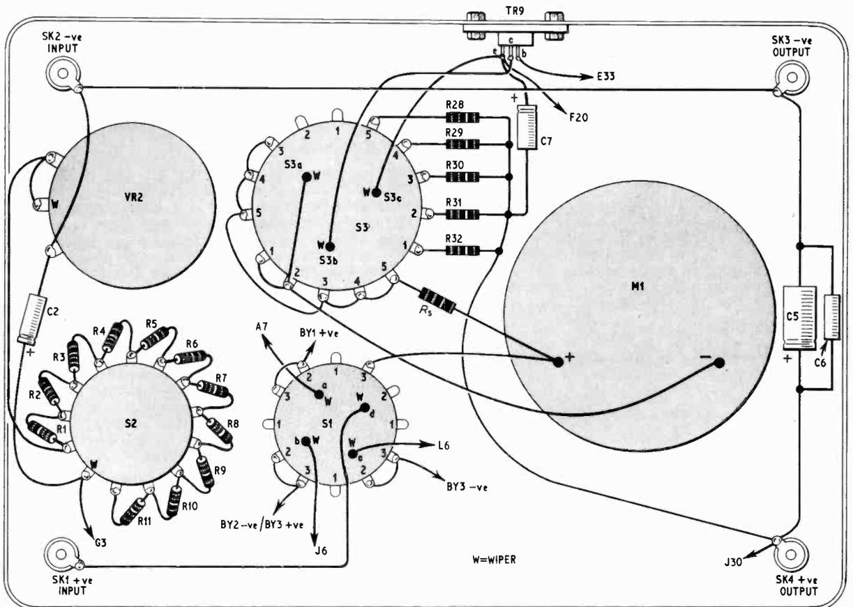
Fig. 5. Internal wiring of the stabiliser
