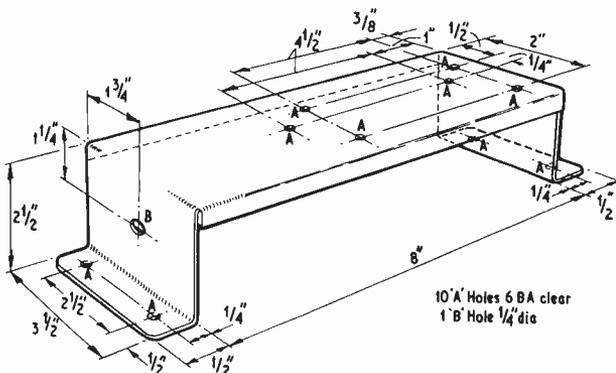
Fig. 5. Panel bridge for mounting the various stage panels
