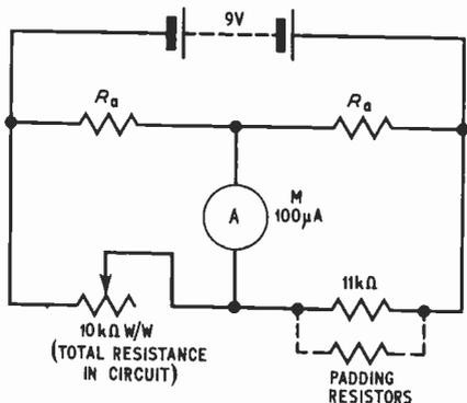
Fig. 3. Wheatstone bridge for resistor matching
