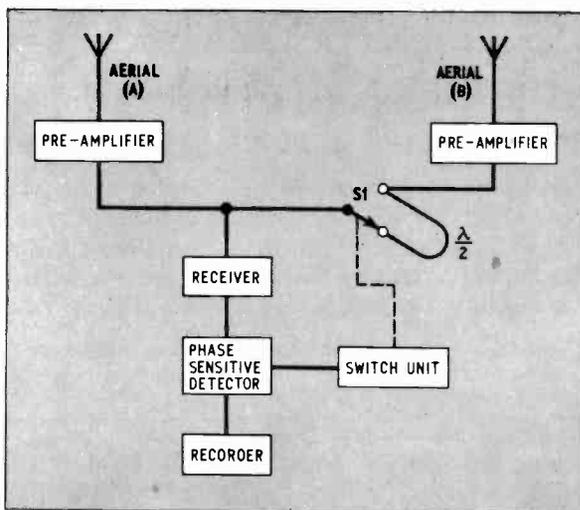
Fig. 3.1. Block diagram of a phase-switched interferometer
