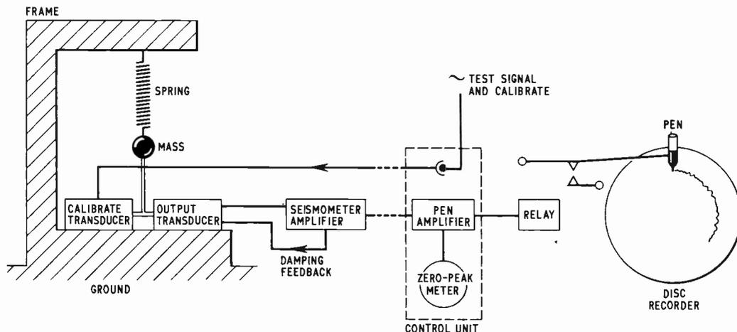
Fig. 1. Block diagram of seismograph
