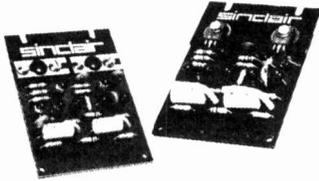
The Z.30 and Z.50 are of advanced design using silicon epitaxial planar transistors to achieve unsurpassed standards of performance. Total harmonic distortion is an incredibly low 0.02% at full output and all lower outputs. Whether you use Z.30 or Z.50 amplifiers in your Project 60 system will depend on personal preference, but they are the same size and may be used with other units in the Project 60 range equally well.
