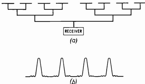
Fig. 3.4. A grating interferometer: (a) arrangement of aerials; (b) reception pattern
