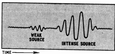
Fig. 3.2. Pattern recorded on phase-switching interferometer
