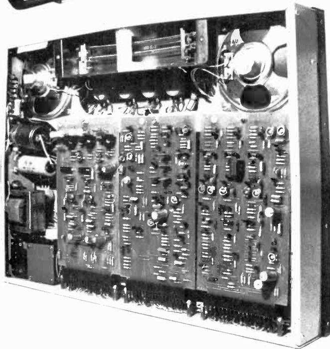
range 1Hz to 10kHz. A third oscillator provides square and ramp waveforms but over the exceptionally low frequency range of 0.025Hz (1 cycle every 40 seconds) to 500Hz.
