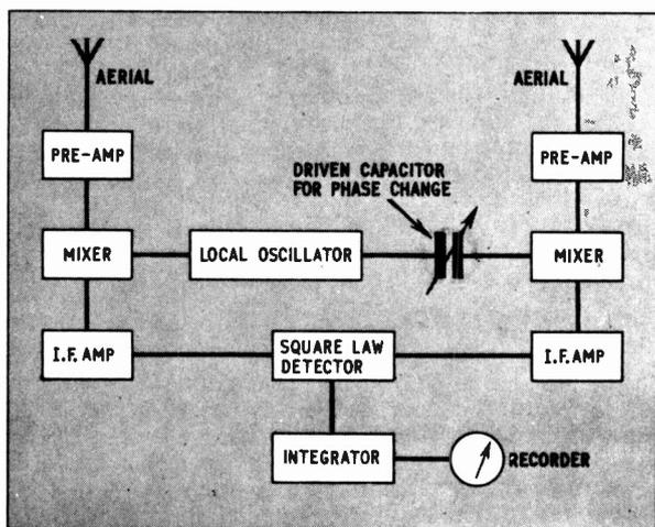
Fig. 3.3. Rotating lobe interferometer
