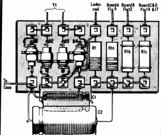
Fig. 7. Wiring of the diodes and capacitors. R1a, R1b, R1c are decoupling resistors 330Ω 3W to supply Boards A, B, C, and D.
