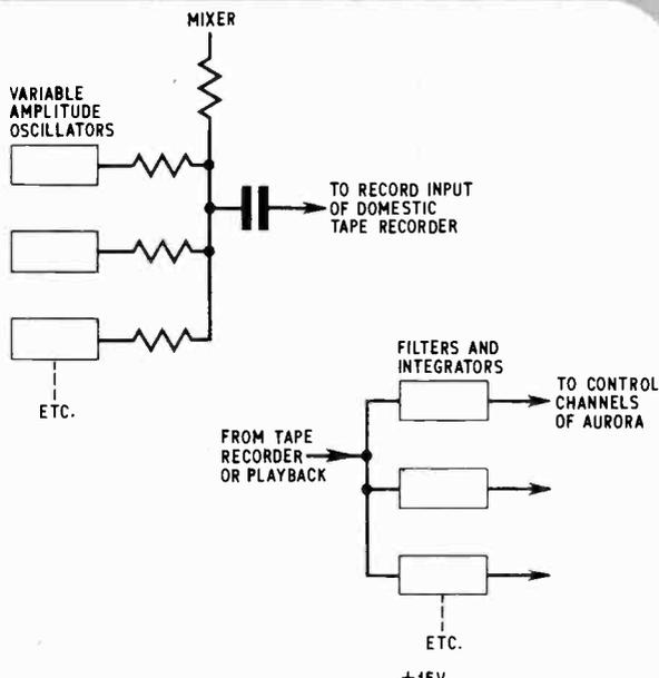
Fig. 6 (top right). Simple schematic for a tape control lighting. The prototype used only three channels to avoid the possibility of interaction. It is quite possible that by careful selection of frequencies harmonic interaction could be avoided if a larger number of channels was desired
