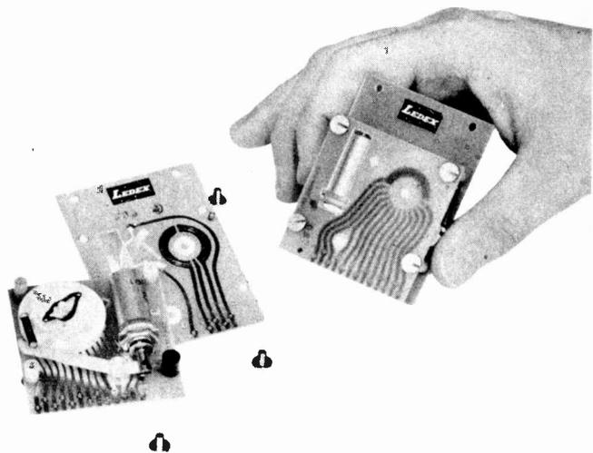
**New approach to the Lexus motorised switch by NSF. Printed circuit board is tracked by a ratchet operated rotating contact wheel (above)**
