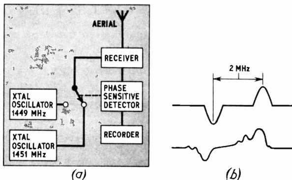
Fig. 3.9. The detection of spectral lines: (a) the switched comparison receiver; (b) typical outputs from receiver
