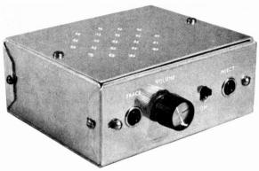
Photograph of the completed signal injector and tracer unit showing the layout of the front panel. The box is built using universal chassis members
