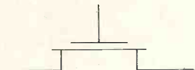
Fig. 1b. Circuit symbol for a MOS transistor
