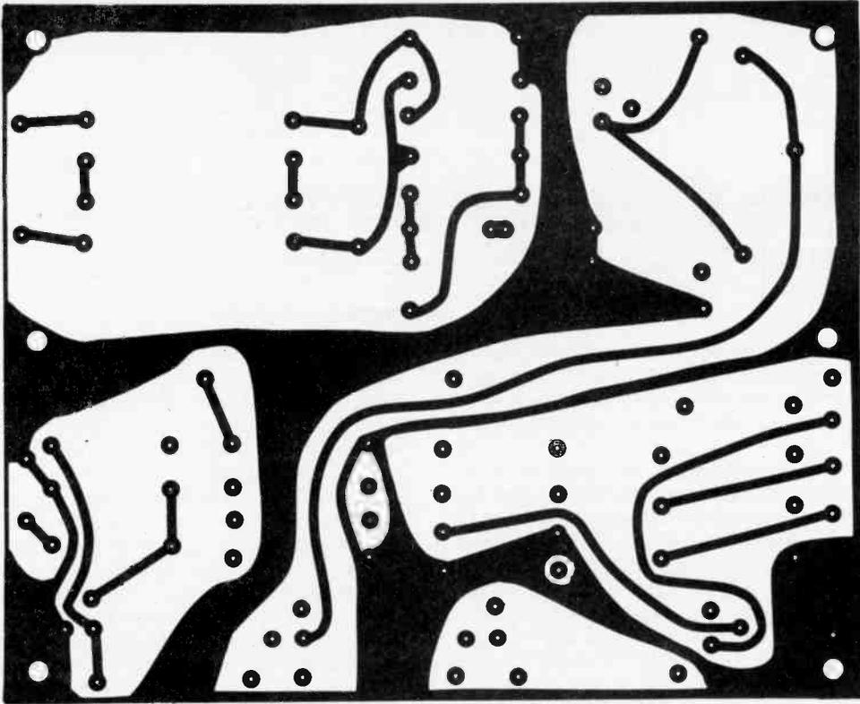
Fig. 3. P.c.b. layout for component side
