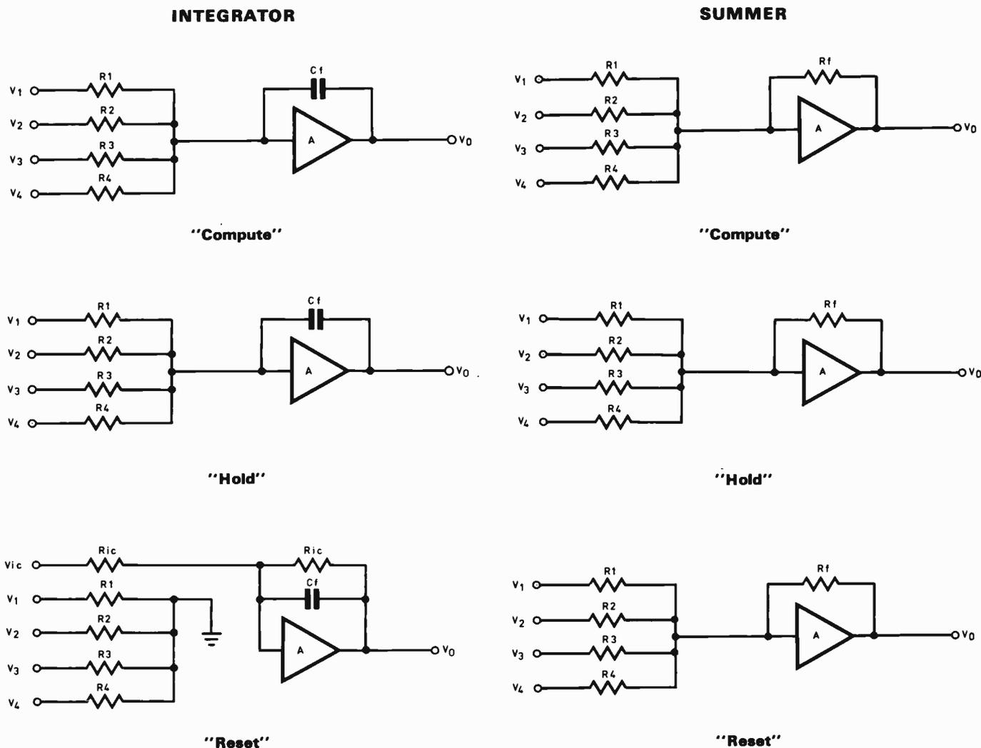
Fig. 1.8. "Initial Condition" circuits for Integrators and Summers
