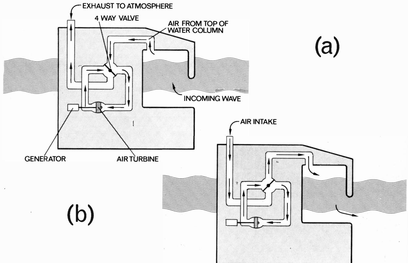
Rectification is achieved by the system shown above, which illustrates the simple OWC principle in its entirety. It employs a kind of pneumatic version of the familiar bridge rectifier circuit. A four-way valve is used to re-route the flow of air in each half cycle so that it always passes through the turbine blades in the same direction. (a) shows the airflow whilst the wave is rising, and (b) shows the situation as a wave trough develops.
