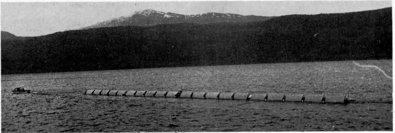
At Edinburgh University where the Salter Duck was originally developed, study is now concentrated on the theoretical and behavioural nature of the machine. On a more practical level at Lanchester Polytechnic (Coventry), Sea Energy Associates build scale models for testing. Shown above are one-fifteenth scale machines (50m string with 30 tonnes displacement) undergoing trials on Loch Ness. Illustrations courtesy of Lanchester Polytechnic
