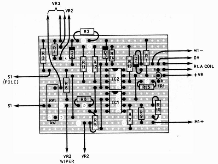
Fig. 2. Stripboard layout shown at full size. Note that C1 is not shown on this diagram
