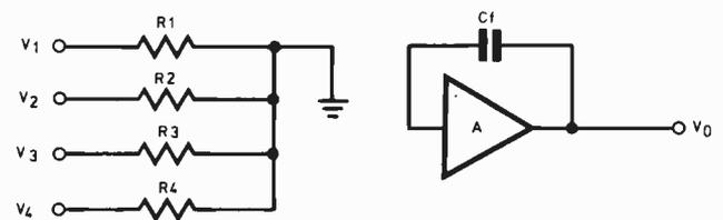
**Fig. 1.3. "Integrator" circuit**
