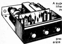
A superb solid state audio amplifier. Brand new components throughout. 5 silicon transistors plus 2 power output transistors in push-pull. Full wave rectification. Output approx. 13 watts r.m.s. into 8 ohms. Frequency response 12Hz-30KHz  $\pm$  3db. Fully integrated pre-amplifier stage with separate Volume, Bass boost and Treble cut controls. Suitable for
