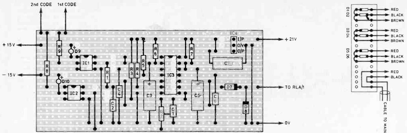
Fig. 2. Stripboard layout of the Combination Lock. The diodes D1 to D6 are mounted separately on a tag board which can be placed next to the code switches. The diode tag board is shown above right
