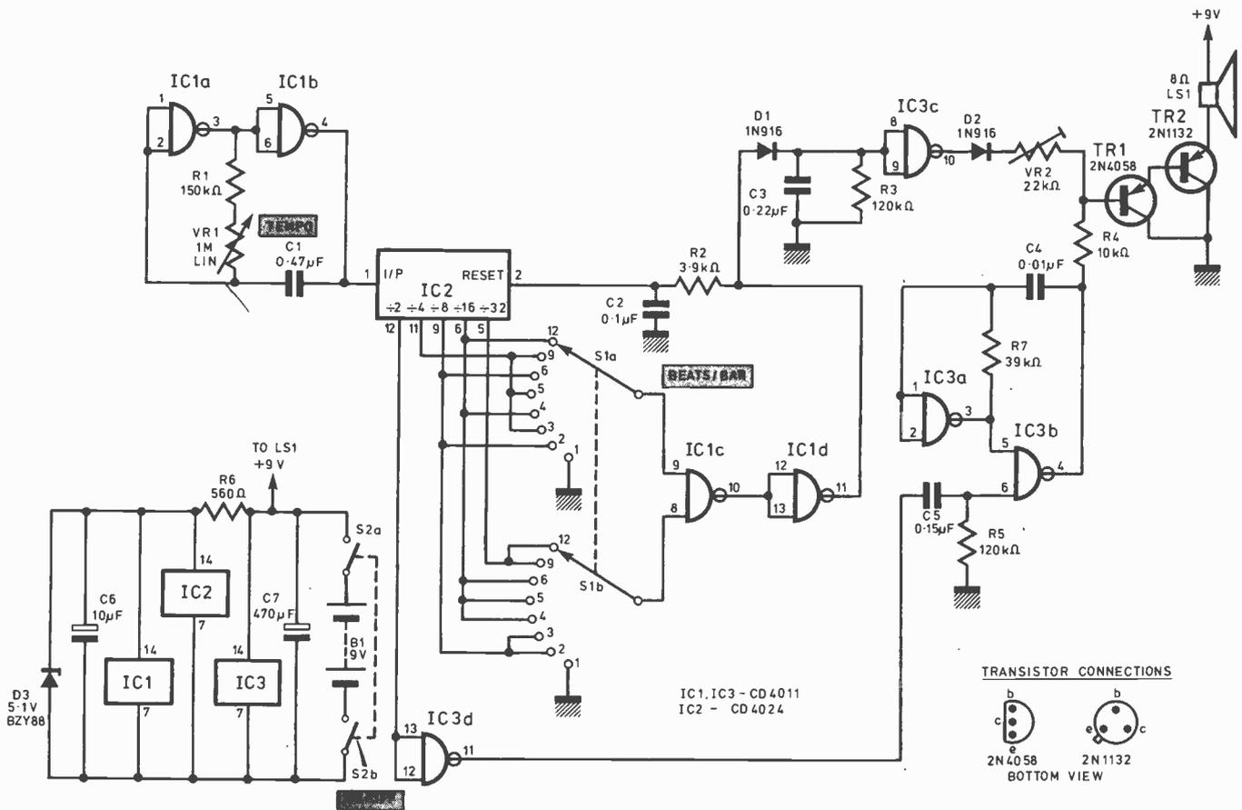
Fig. 1. Full circuit diagram of the Metronome
