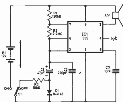
THE enclosed circuit utilises the timing capability of the 555, together with its capacity to directly drive a small audio transducer. It provides an economical arrangement to provide an audible alarm.
