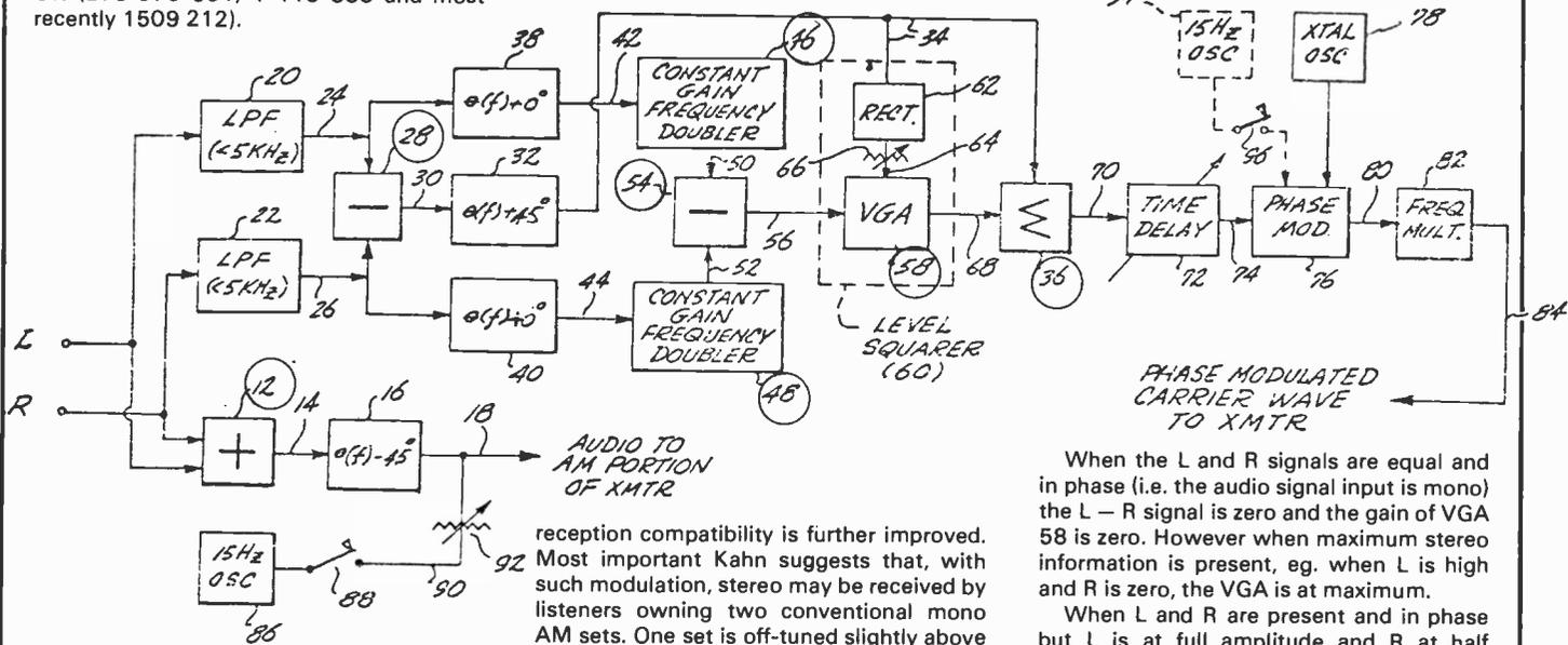
reception compatibility is further improved. Most important Kahn suggests that, with such modulation, stereo may be received by listeners owning two conventional mono AM sets. One set is off-tuned slightly above the carrier and the other slightly below the carrier to provide combined reception in the stereophonic mode.
