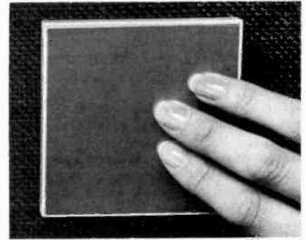
A subsequent long touch will alter the light level in the reverse direction and removing the hand from the control during the cycle will establish the light level.
