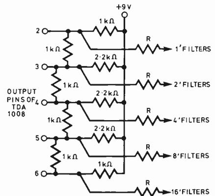
Fig. 8. A method for staircasing the output pitches as an alternative to square waves produced by the simple arrangement in Fig. 1
