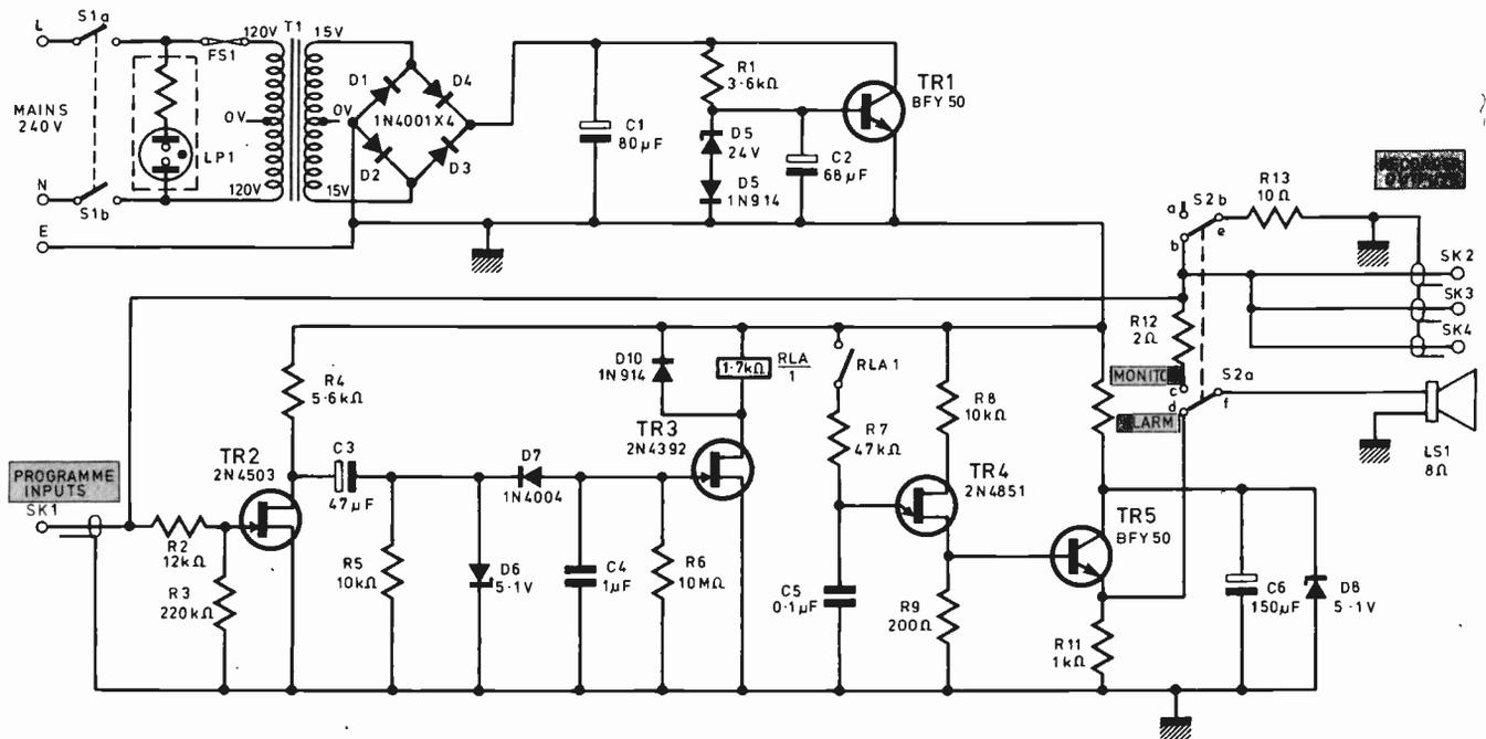
Fig. 2. Circuit of Sound Monitor
