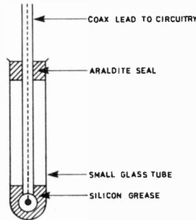
A temperature probe can be fabricated from a small test tube
