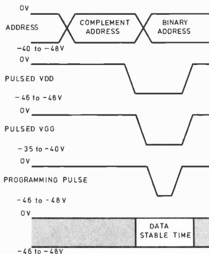
*that the program pulse is a 3ms -47V pulse as required. As with many things in electronics, the secret lies in viewing the circuit operation with one's feet firmly on the ground (or in this case, the ceiling!). If you check the other supplies with this new perspective, you will find that they are substantially as dictated in the data sheet.*
