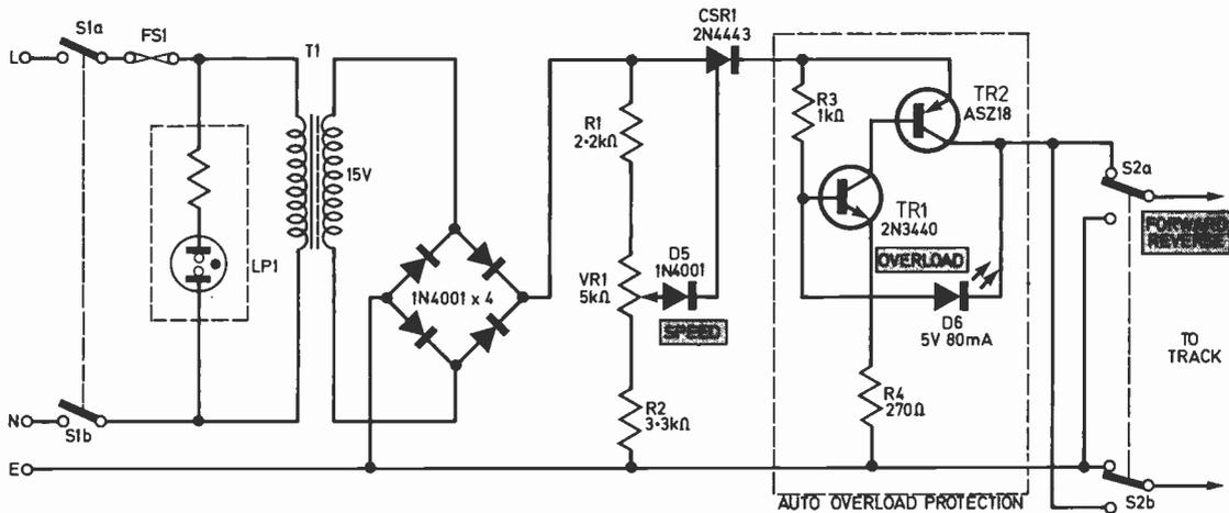
THE circuit shown in the diagram is based on the "Model Train Speed Controller" that appeared in PE December, 1976. The additional circuitry is shown within the dotted lines. This addition, which is suitable for one engine only, can be included to perform three functions:
