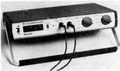
The unit is very light—less than 1½lbs—and measures 255 x 148 x 40mm. It is powered by four dry cell batteries and optional extras include a rechargeable battery pack, carrying case and a 30kV probe.
