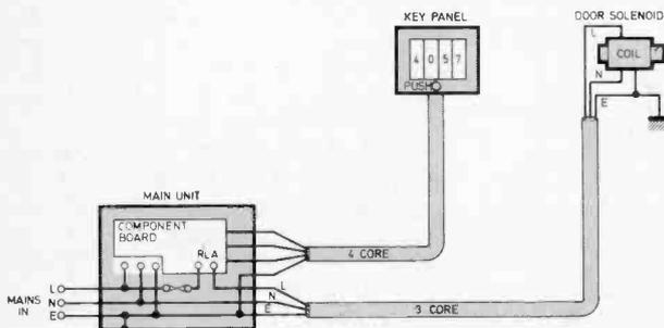
Fig. 3. Wiring diagram of solenoid circuit. Care should be taken when wiring up this mains portion of the system
