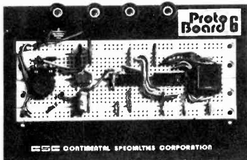
THE PB-6 630 SOLDERLESS CONTACTS. TAKES UP TO SIX 14-PIN DIP'S OR EQUIVALENT IN LARGER AND SMALLER IC'S. FOUR 5-WAY BINDING POSTS. 6" x 4"
