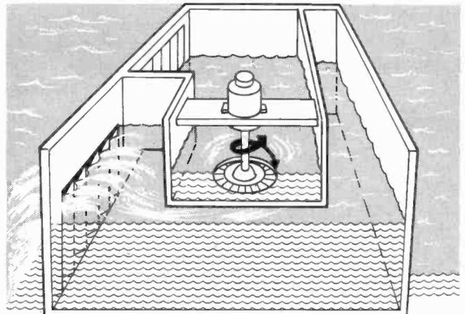
The Russell Rectifier is shown above in both states of flux. (left) The upper chamber fills as the wave rises. (right) The lower chamber empties during the trough of a wave. Courtesy of HRS
