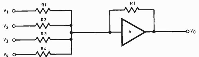
**Fig. 1.2. "Addition" circuit**
