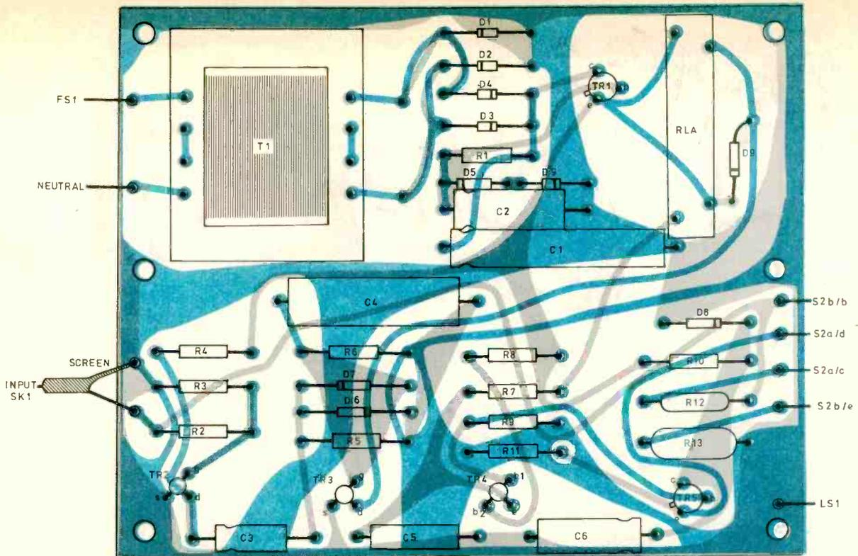
Fig. 5. Component assembly in double sided p.c.b.
