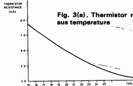
Fig. 3(a). Thermistor resistance versus temperature
