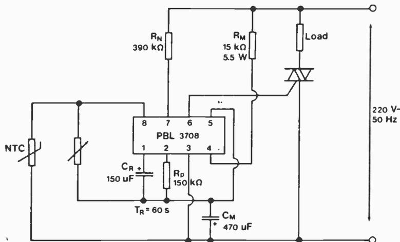
A typical design for control of room temperature with a heating element of 1,000W, 220V a.c. and a proportional band of 1°C.
