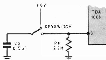
keying is achieved by supplying +6V through a keyswitch. Signal output voltage is proportional to keyed input voltage, whilst multiple inputs produce sum signals. Unused outputs should be connected to +6V to avoid intermodulation, though all five will normally be in use.
