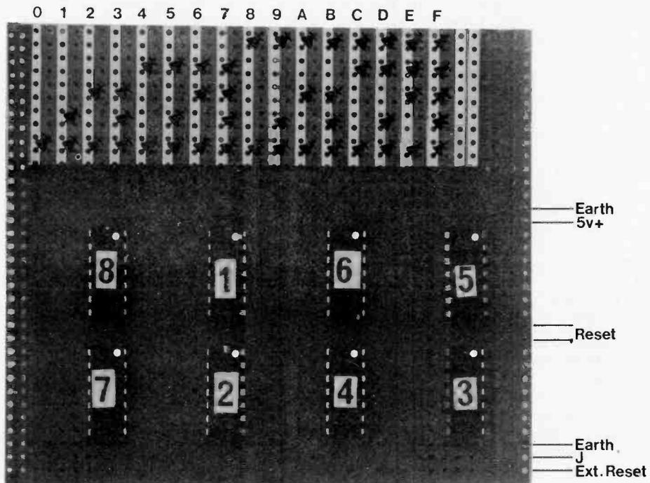
**Main board prototype showing component layout and surface wiring. Note that the copper tracks of the two boards for the diode matrix are at right angles and the diodes are mounted diagonally so that each diode wire passes through the copper strip of only one board**
