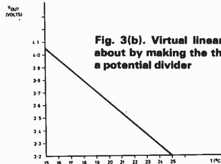
Fig. 3(b). Virtual linearisation brought about by making the thermistor part of a potential divider
