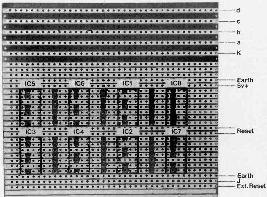
**Fig. 2. Identification of rows on the circuit board for the wiring schedule. Copper cuts for the i.c.s are also shown**
