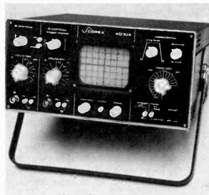
The black 4D10A dual trace scope, at £180, still retains the characteristics of the 4D10; stabilised power supplies in both the low voltage areas and e.h.t. allowing mains variation of as much as ten per cent. Accuracy on both time and voltage measurements is three per cent.
