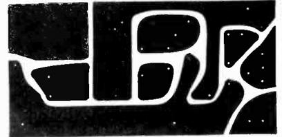
Fig. 4. Component layout for AF Oscillator
