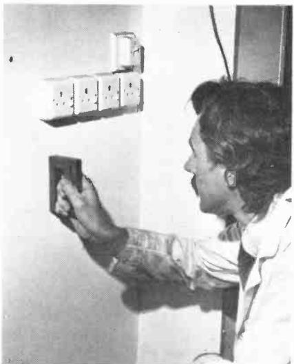
There are three models: a metal detector (403), a voltage indicator (405), and a combination unit (407).
