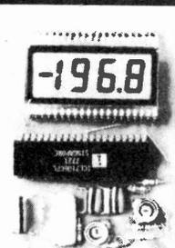
Based on the 7106 single IC 3 1/2 digit D.V.M. the Kit contains a PCB, resistors, capacitors, presets, I.C. and 0.5" liquid crystal display. Components are also included to enable the basic D.V.M. kit to be modified to a Digital Thermometer using a single transistor as the sensor.
