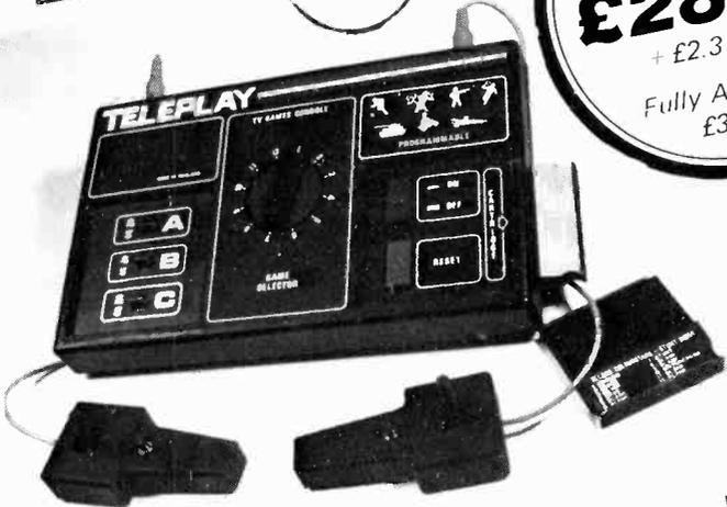
Main Console has 3 Facility Handicapping Switches.
