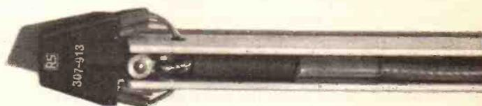
THIS INSTRUMENT WILL MEASURE THE R.P.M. OF A REVOLVING OBJECT, USING A REFLECTIVE OPTO SWITCH AS THE SENSOR. ALL THAT IS REQUIRED IS THE APPLICATION OF STICKY TAPE TO ACT AS AN OPTICAL MARKER.
