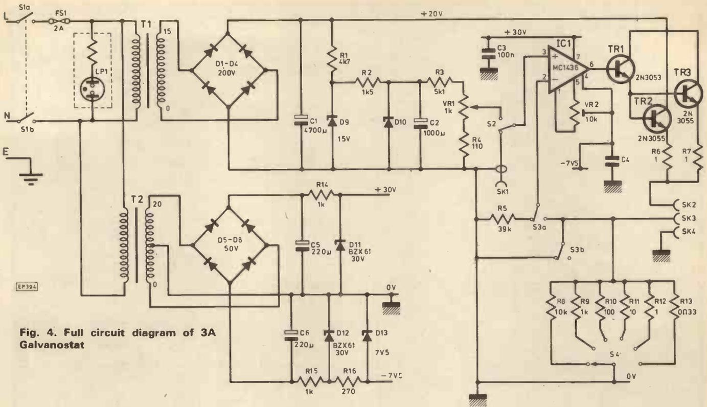
Fig. 4. Full circuit diagram of 3A Galvanostat
