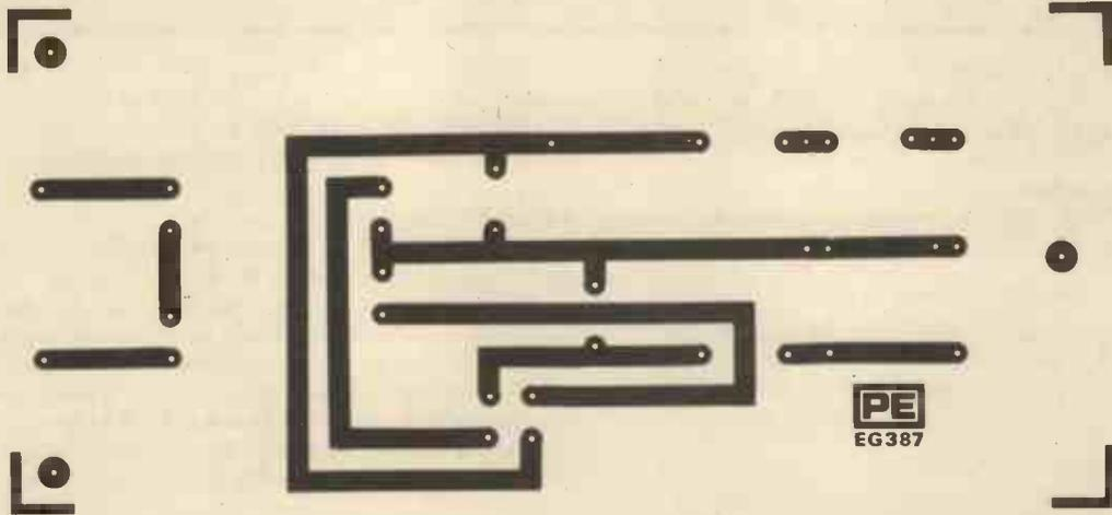
Fig. 5. Printed circuit for op. amp. power supply board (actual size)
