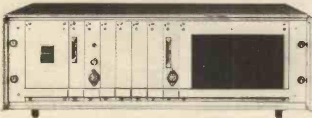
System 3, contains the 6502 CPU, 16K RAM with DOS and BASIC, VDU Interface, Disc controller and 5" drive, Printer Interface, backplane and power supplies. The entire unit costs about £1,000 and can be added to or reformatted as required.
