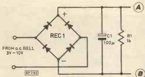
Fig. 1. If used with a battery operated bell connect A and B to the existing bell-push switch wires. For a.c. bells (3-10V) connect the rectifier circuit as shown.
