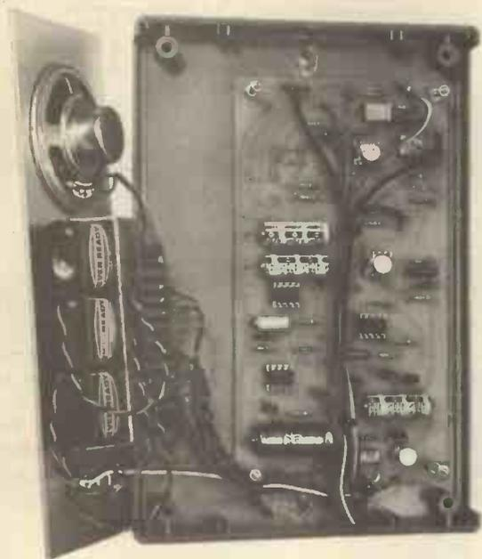
Power supply, autotune and output board
