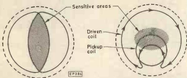
Fig. 1 (left). 'Widescan' coil layout; (right) 'Pinpoint' coil layout
