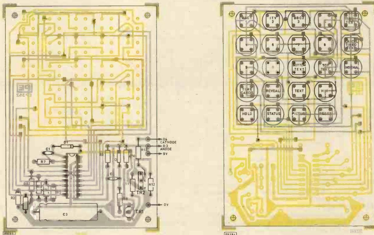
Fig. 1.5. Component layout for the transmitter board which also shows the through board links (square pads)
