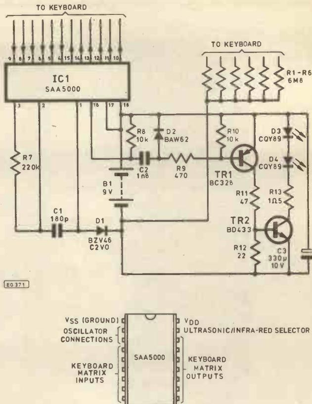
Fig. 1.2. Circuit diagram of the Transmitter unit
