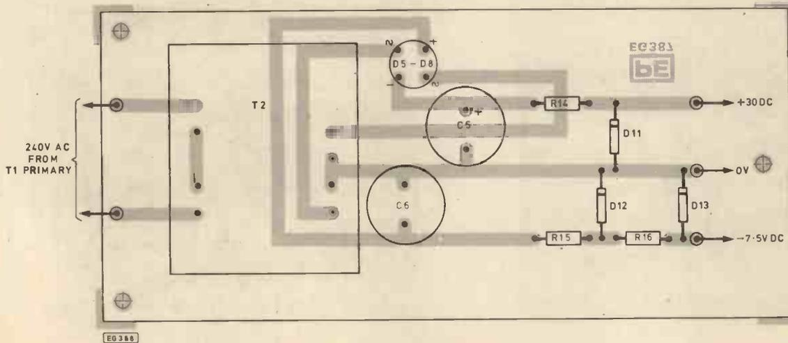
Fig. 6. Component overlay for above
