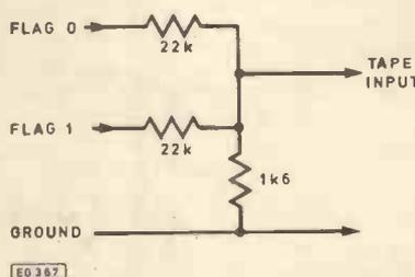
Fig. 2. Interface circuit to enable the Mk14 to drive the auxiliary input of a tape recorder.
