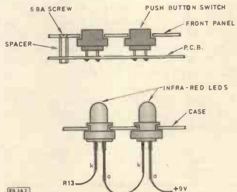
Fig. 1.6. Wiring diagram for the infra-red diodes (D3 and D4) and the mounting details for the p.c.b.
