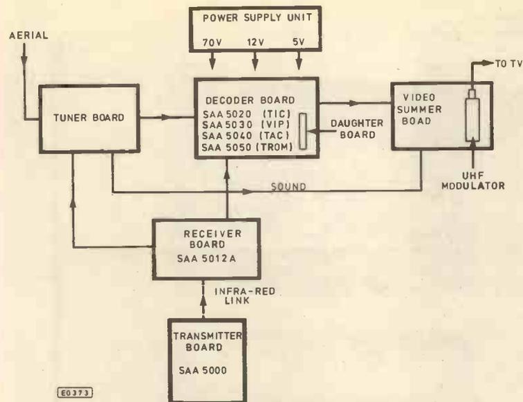
Fig. 1.1. Block diagram of the PE Teletext system
