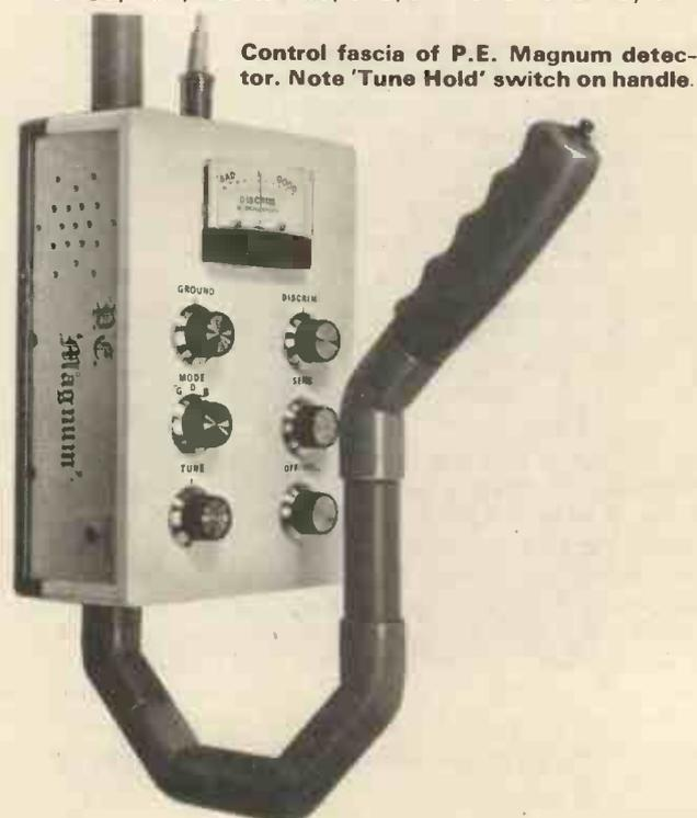
Control fascia of P.E. Magnum detector. Note 'Tune Hold' switch on handle.
