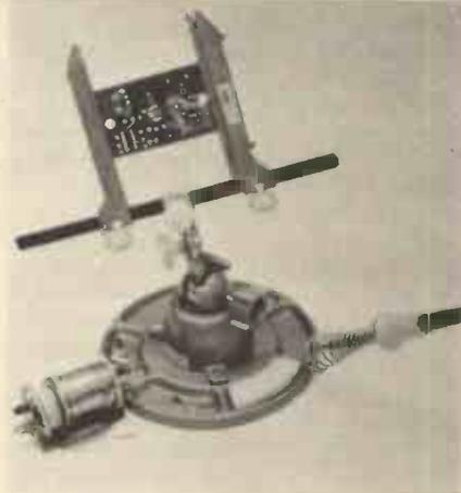
tion. The 315 p.c.b. Holder handles circuit boards up to 200mm wide and 4mm thick and extra pairs of arms and an extension bar are available to enable several p.c.b.'s to be worked on at once. The 371 Solder Station consists of a wire spring soldering iron holder, capable of holding most popular irons, a shaped sponge which fits the tray base and a combined wire and solder reel holder. (Soldering iron, reel of solder and wire not supplied).
