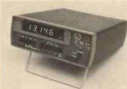
between 0.15 and 0.8 per cent on the resistance range; 0.05 per cent on the d.c. voltage range and 0.5 per cent on the a.c. voltage range.
