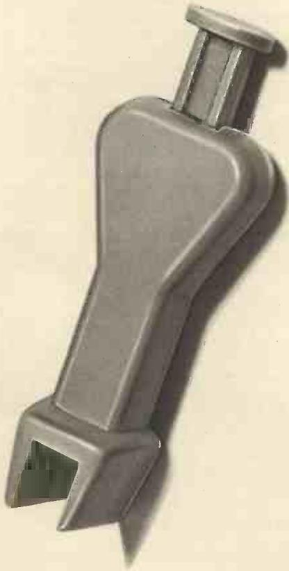
The I.C. INSERTION TOOL attached to the front cover of this issue has been specially designed and manufactured for P.E. and is **exclusive to this magazine**. The tool can be used to insert any standard size d.i.l. i.c.s with up to 16 pins, and enables insertion without the problems of pin misalignment or handling; the tool is made of anti-static plastic.
