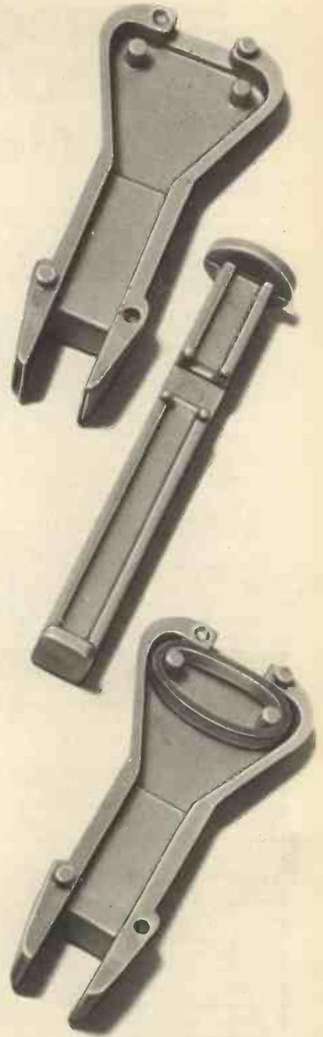
The above photograph shows the tool dismantled. This enables the elastic band, which forms the plunger return spring, to be replaced should it ever perish. The two halves of the body can be parted by carefully inserting a blade in the joint. It is then a simple operation to replace the band and reassemble the tool.
