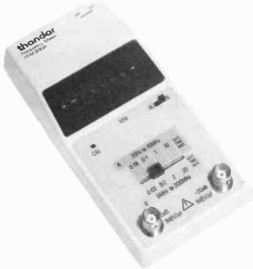
The **PFM 200A** is a pocket sized counter with an 8-digit l.e.d. display covering a frequency range from 20Hz to 200MHz using two ranges. Resolution for the unit is down to 0.1Hz and the sensitivity is typically 10mV r.m.s. Battery life, depending upon range and display, is around 10 hours. Two prescalers (up to 600MHz and 1GHz) are available as optional accessories. The PFM 200A is priced at £79.93 and is available from **Audio Electronics**, 301 Edgware Road, London. (01-724 3564).
