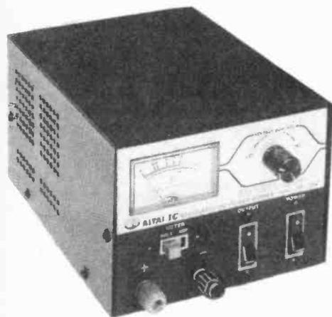
**Altai PP154** variable stabilised PSU with overload protection, ranges from 5-15V d.c. output at 4A. Stability is 0.1% with ripple confined to 5mV. Meter reads voltage or current (switched). Price £46. Available from **Semiconductor Supplies International Ltd.**, Dawson House, 128/130 Carshalton Rd., Sutton, Surrey SM1 4RS. (01-643 1126)
