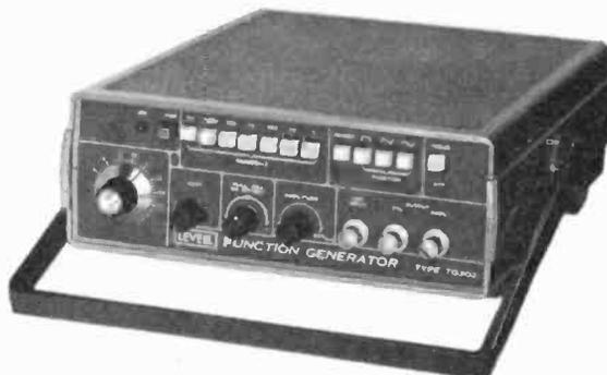
**Levell TG302** function generator can generate triangle, square, sine, pulse and ramp waveforms from 0.02Hz to 2MHz in 7 ranges. It provides 20V p.p. from a 50 $\Omega$  source with variable offset. TTL output. External sweep over three decades. Built-in frequency counter to 10MHz. Price £155.25. Available from **Levell Electronics Ltd.**, Moxon St., Barnet, Herts EN5 5SD. (01-440 8686)
