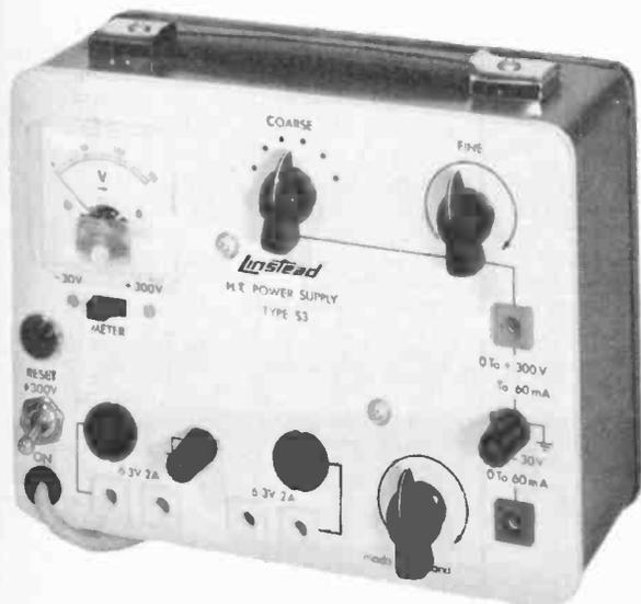
**Linstead S3 HT/LT** bench PSU has 0-300V (@ 60mA) and 0-30V d.c. (ripple = 100mA). Also incorporates two isolated 6.3V @ 2A heater supplies. The PSU is fully protected against overload and short circuit by a variable trip. Voltage outputs monitored by switched meter. Price £140.30. Available from **Supercat Electronics Ltd.**, PO Box 201, St. Albans, Herts AL1 4EN. (0727 62171)
