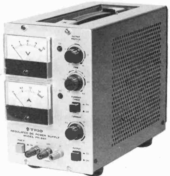
The **PR 651** is a regulated power supply, 0V to 18V at 1.5A. Both voltage and current can be read at the same time. The unit features circuit protection to minimise constant current/voltage output drift. Also available is the **PR 653**, this is a 0 to 35V at 1.5A supply with the same characteristics and features. Prices respectively are £212.75 and £228.85. From **House of Instruments**, Clifton Chambers, 62 High Street, Saffron Walden, Essex CB10 1EE (0799 24922).
