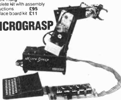
A real programmable robot for under £300! Micrograsp has an articulated arm jointed at shoulder, elbow and wrist positions. The entire arm rotates about its base and there is a motor driven gripper. All five axes are motor driven and four of these are servo controlled giving positive positioning. The robot can be controlled by any microcomputer with an expansion bus - the Sinclair ZX81 being particularly suitable.
